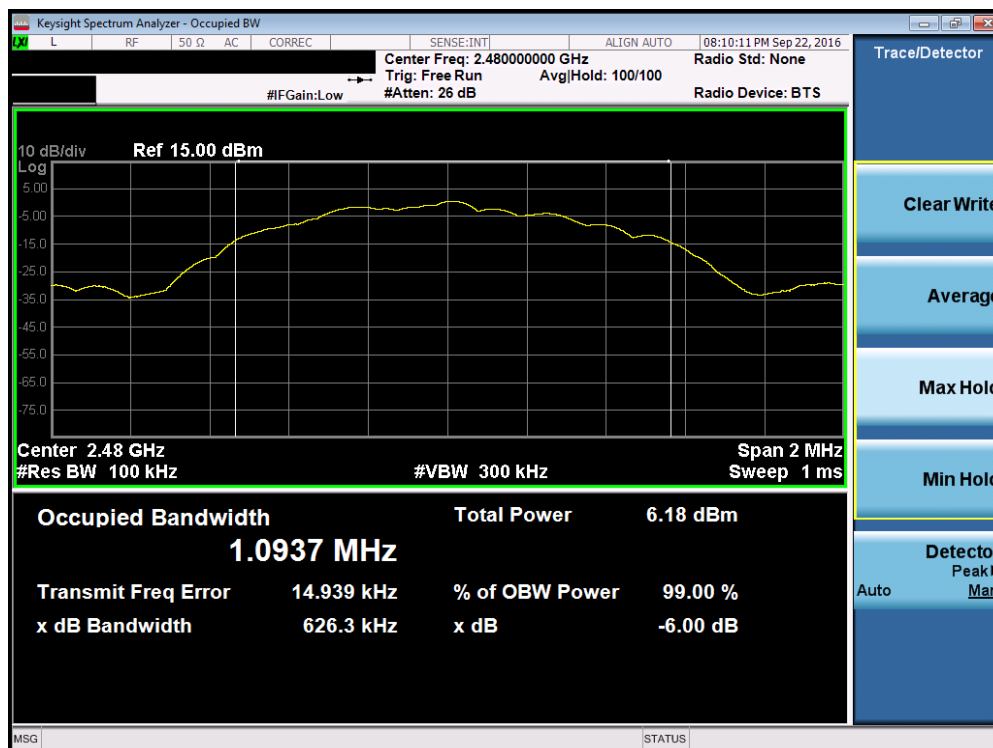
Plot 7-3. 6dB Bandwidth Plot (Bluetooth (LE) – Ch. 39)
