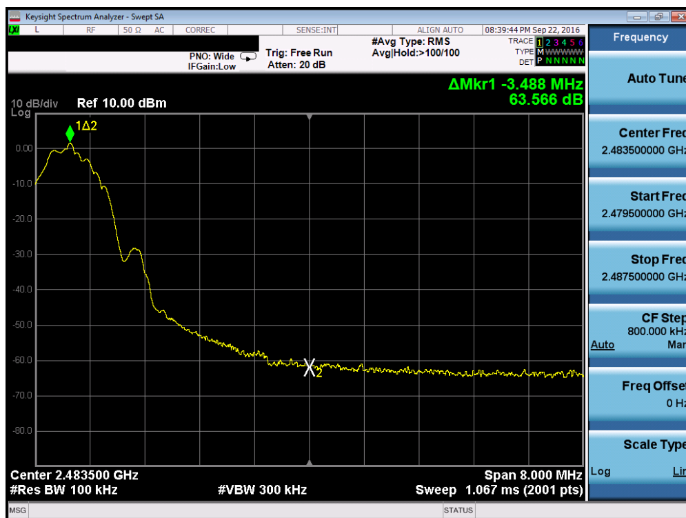
Plot 7-11. Band Edge Plot (Bluetooth (LE) – Ch. 39)
