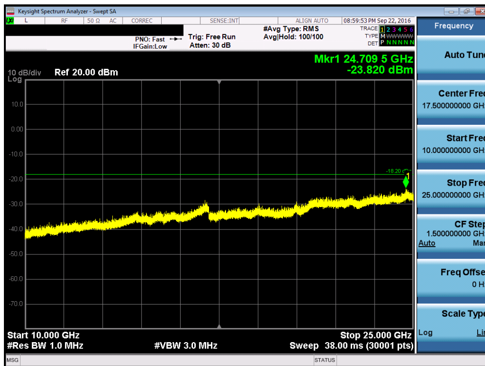
Plot 7-13. Conducted Spurious Plot (Bluetooth (LE) – Ch. 0)
