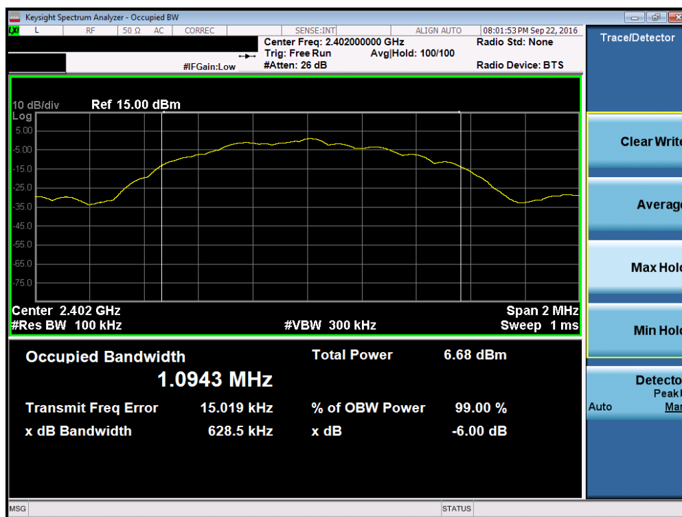
Plot 7-1. 6dB Bandwidth Plot (Bluetooth (LE) – Ch. 0)
