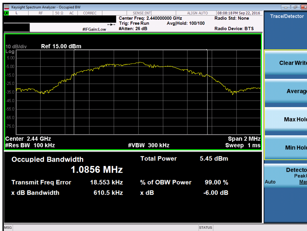
Plot 7-2. 6dB Bandwidth Plot (Bluetooth (LE) – Ch. 19)
