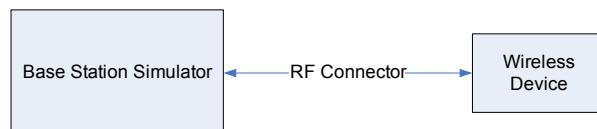
Figure 9-1 Power Measurement Setup
