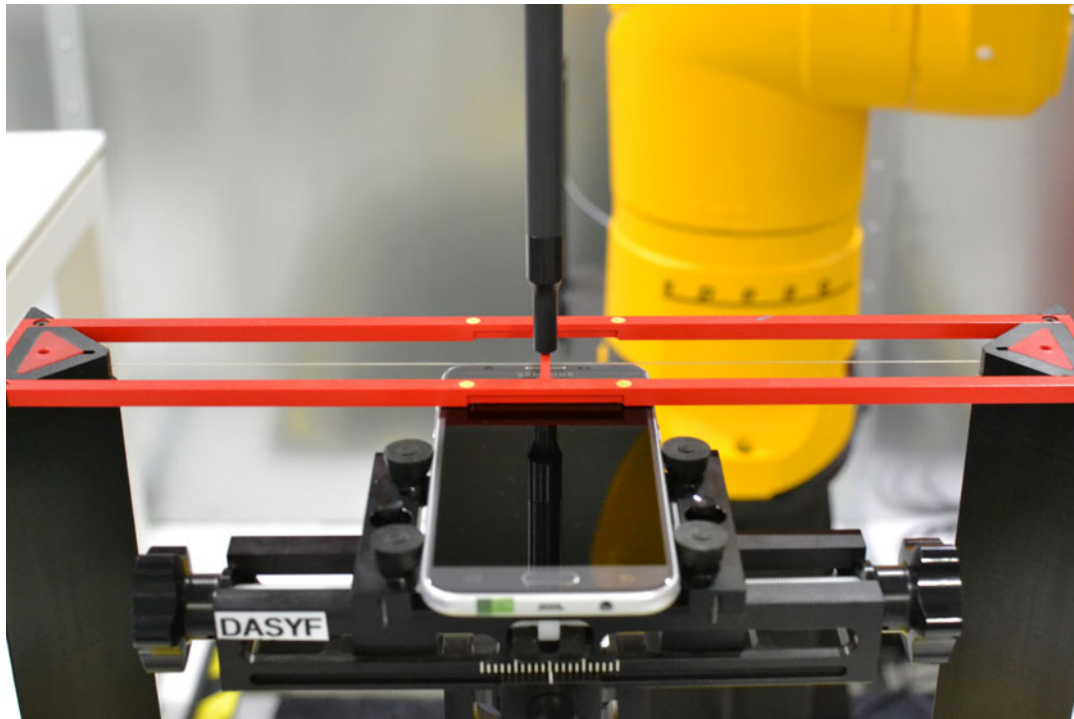
Figure 17-1 Ear Reference Point HAC Phantom Alignment
