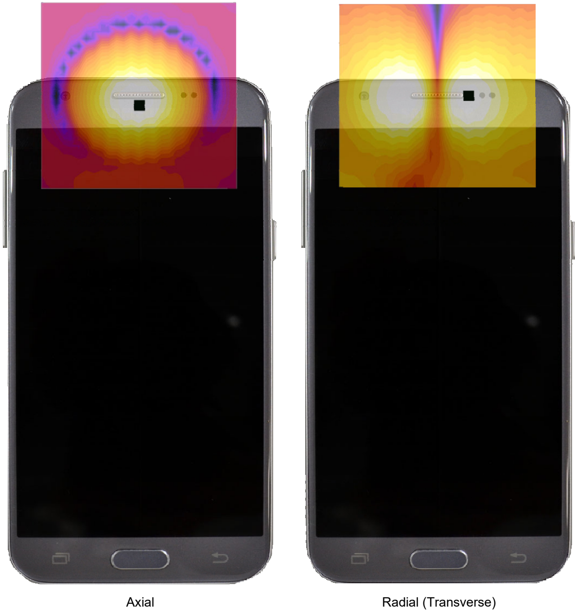
Figure 14-3 T-Coil Scan Overlay Magnetic Field Distributions
