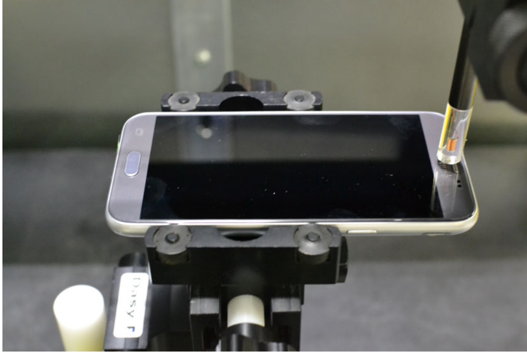
Figure 14-1 Test Setup for Wireless Device
