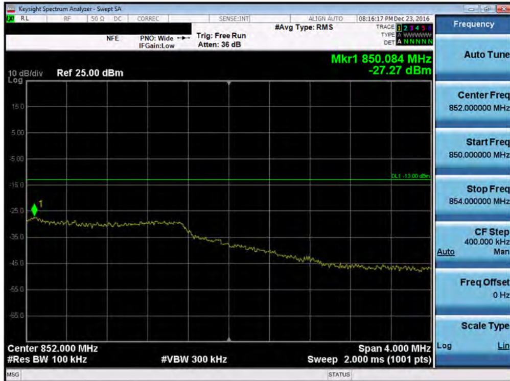
Plot 7-98. Upper Extended Band Edge Plot (Band 5 – Band 5 – 3.0MHz QPSK – RB Size 15)
