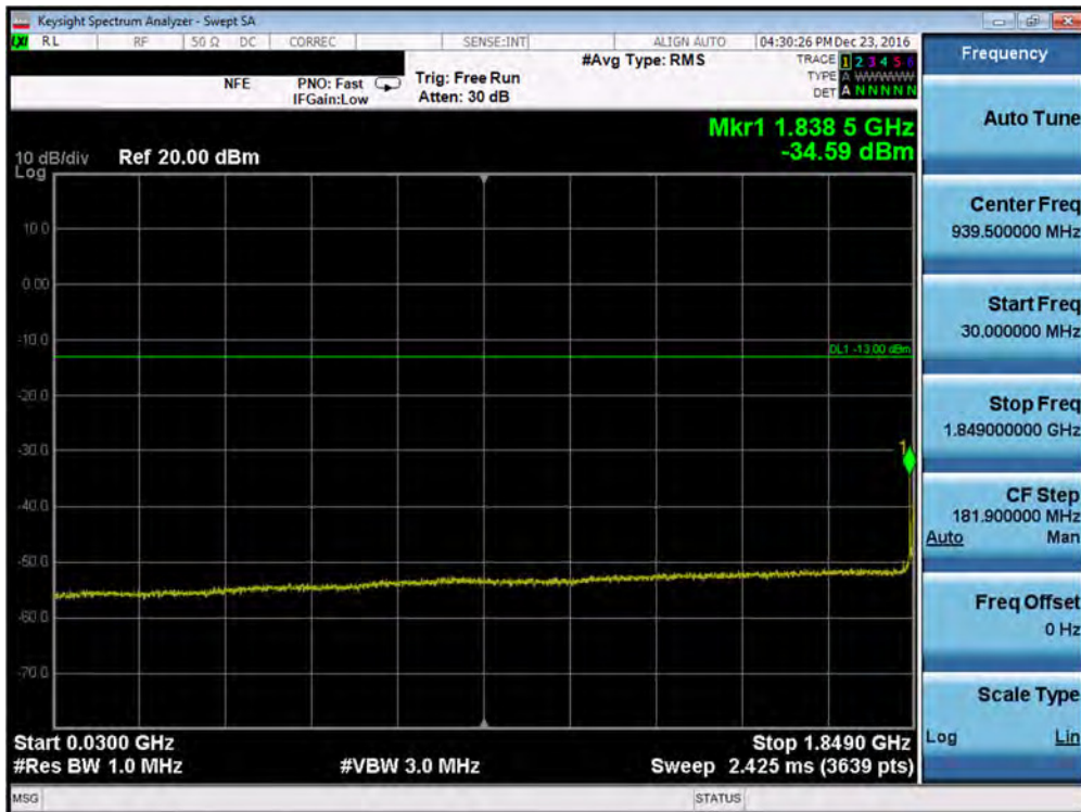
Plot 7-68. Conducted Spurious Plot (Band 2 – 15.0MHz QPSK – RB Size 1, RB Offset 0 – Low Channel)
