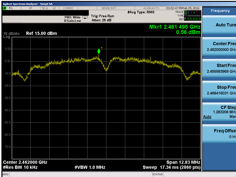
Plot 7-12. Power Spectral Density Plot (802.11b – Ch. 11)
