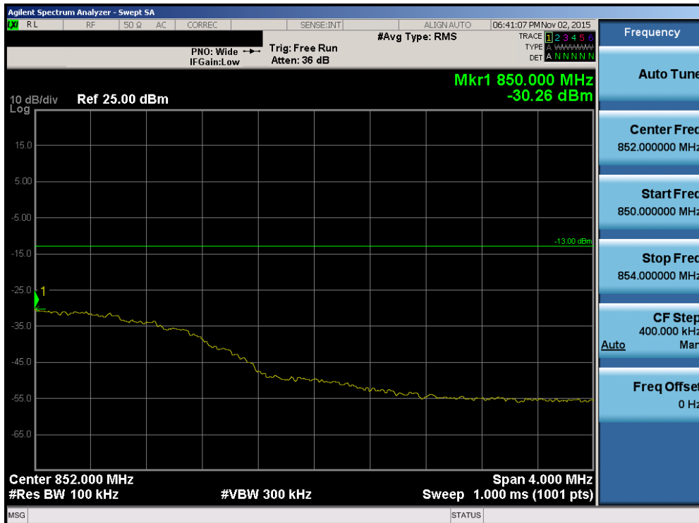
Plot 7-117. Upper Extended Band Edge Plot (Band 5/26 – 3.0MHz QPSK – RB Size 15)
