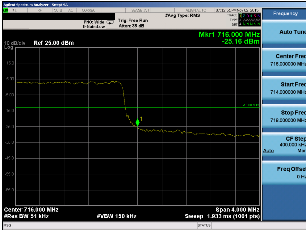
Plot 7-106. Upper Band Edge Plot (Band 12 – 5.0MHz QPSK – RB Size 25)
