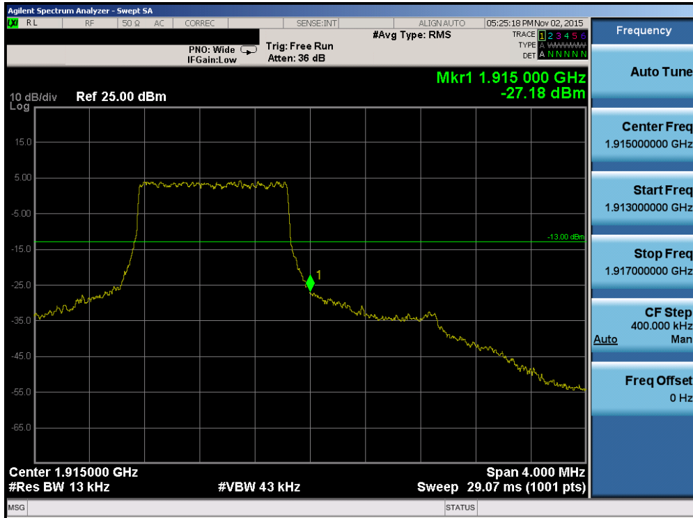
Plot 7-152. Upper Band Edge Plot (Band 2/25 – 1.4MHz QPSK – RB Size 6)
