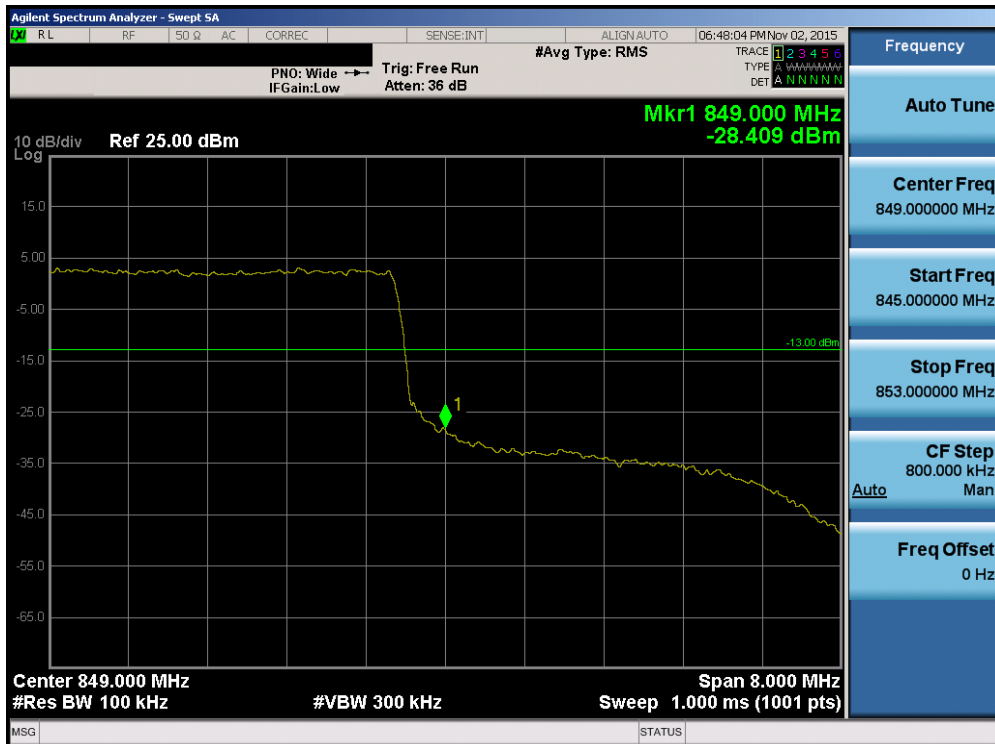
Plot 7-123. Upper Band Edge Plot (Band 5/26 – 10.0MHz QPSK – RB Size 50)
