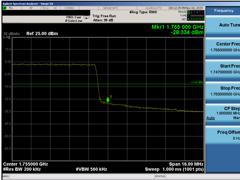
Plot 7-148. Upper Band Edge Plot (Band 4 – 20.0MHz QPSK – RB Size 100)
