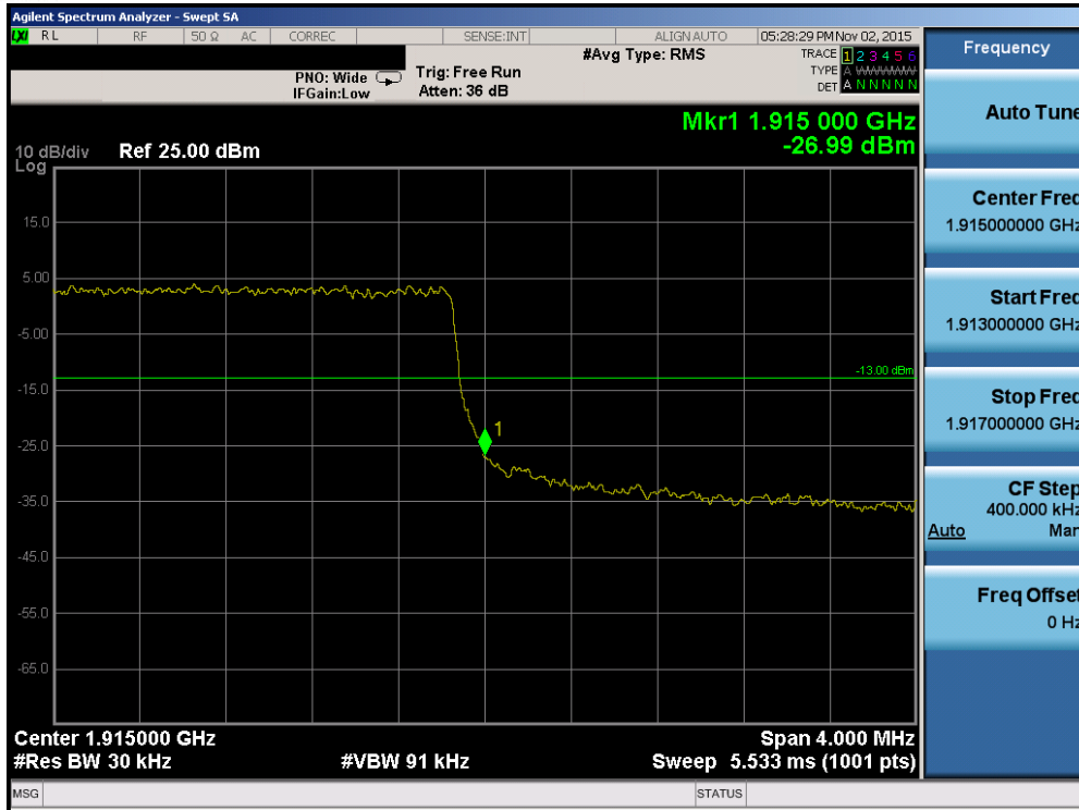
Plot 7-156. Upper Band Edge Plot (Band 2/25 – 3.0MHz QPSK – RB Size 15)
