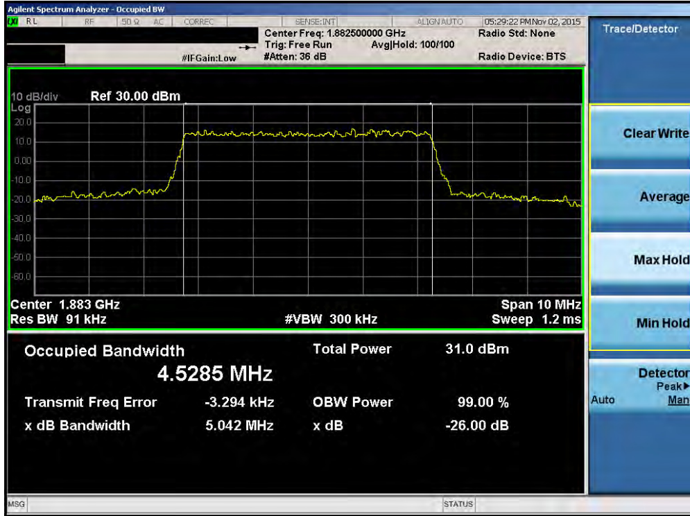
Plot 7-35. Occupied Bandwidth Plot (Band 2/25 – 5.0MHz QPSK – RB Size 25)
