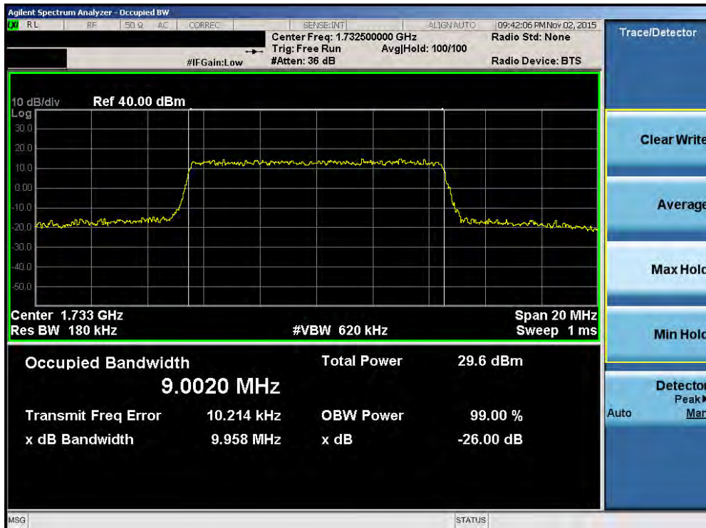
Plot 7-26. Occupied Bandwidth Plot (Band 4 – 10.0MHz 16-QAM – RB Size 50)
