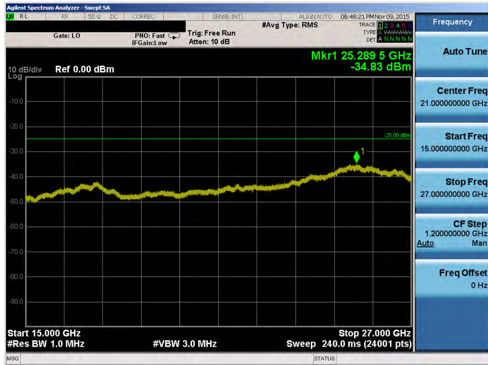
Plot 7-92. Conducted Spurious Plot (Band 41 – 5.0MHz QPSK – RB Size 1, RB Offset 0 – Mid Channel)
