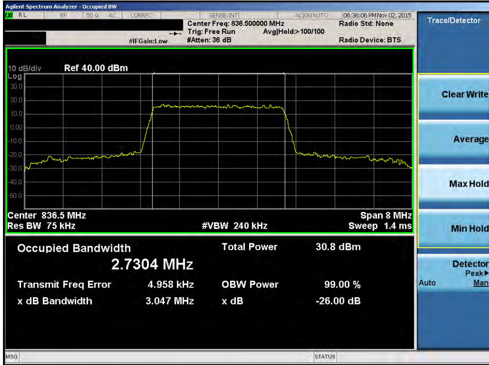
Plot 7-11. Occupied Bandwidth Plot (Band 5/26 – 3.0MHz QPSK – RB Size 15)
