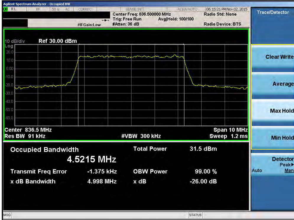
Plot 7-13. Occupied Bandwidth Plot (Band 5/26 – 5.0MHz QPSK – RB Size 25)
