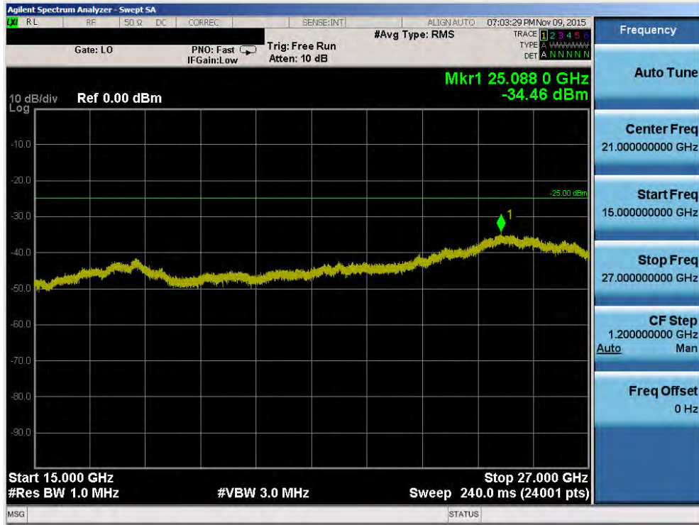
Plot 7-89. Conducted Spurious Plot (Band 41 – 5.0MHz QPSK – RB Size 1, RB Offset 0 – Low Channel)
