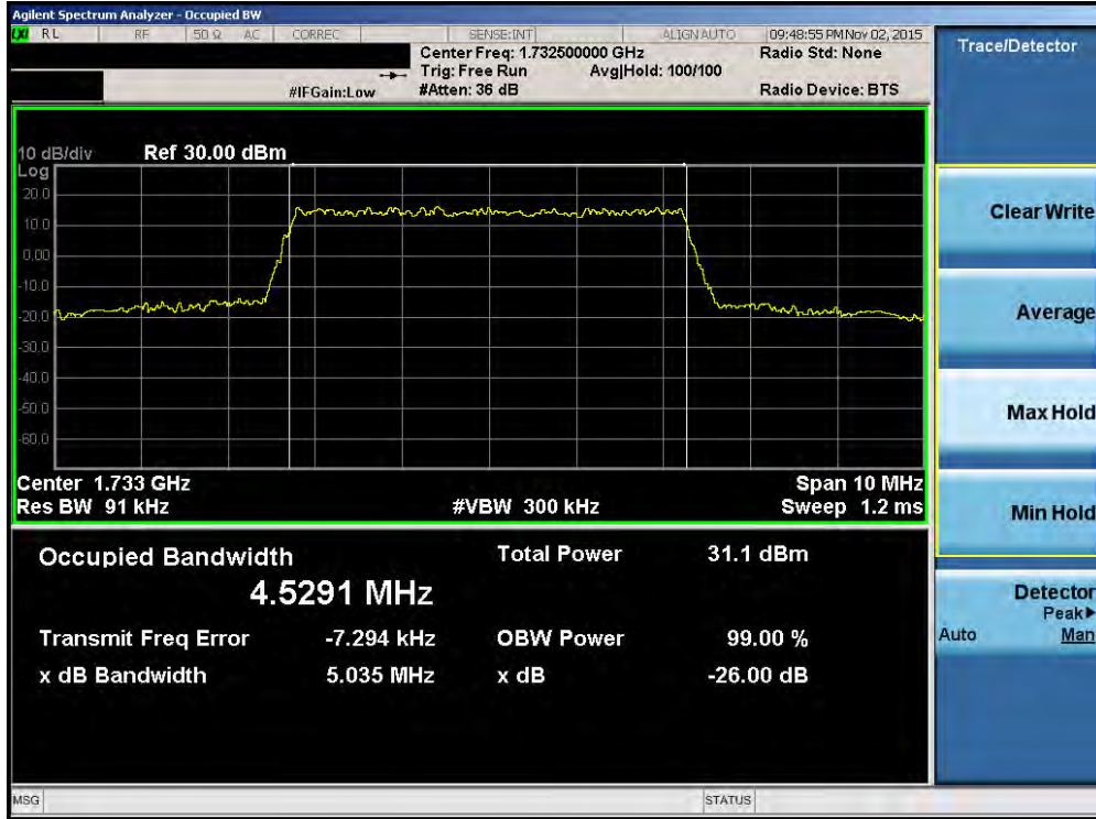
Plot 7-23. Occupied Bandwidth Plot (Band 4 – 5.0MHz QPSK – RB Size 25)
