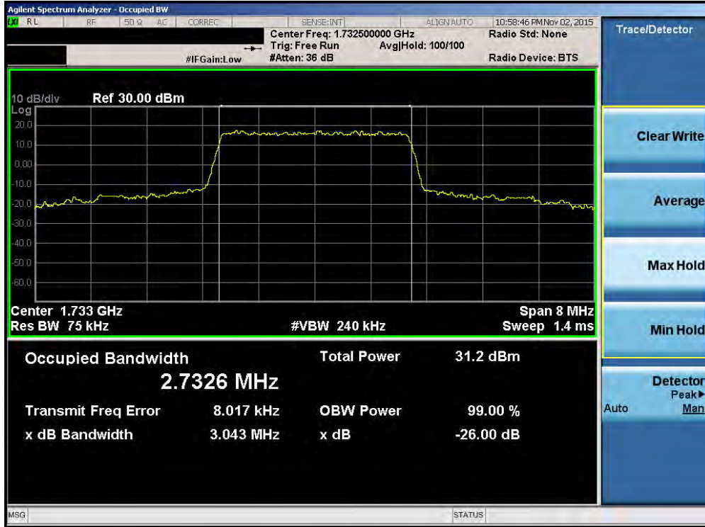
Plot 7-21. Occupied Bandwidth Plot (Band 4 – 3.0MHz QPSK – RB Size 15)
