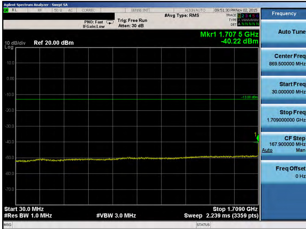
Plot 7-69. Conducted Spurious Plot (Band 4 – 5.0MHz QPSK – RB Size 1, RB Offset 0 – Low Channel)
