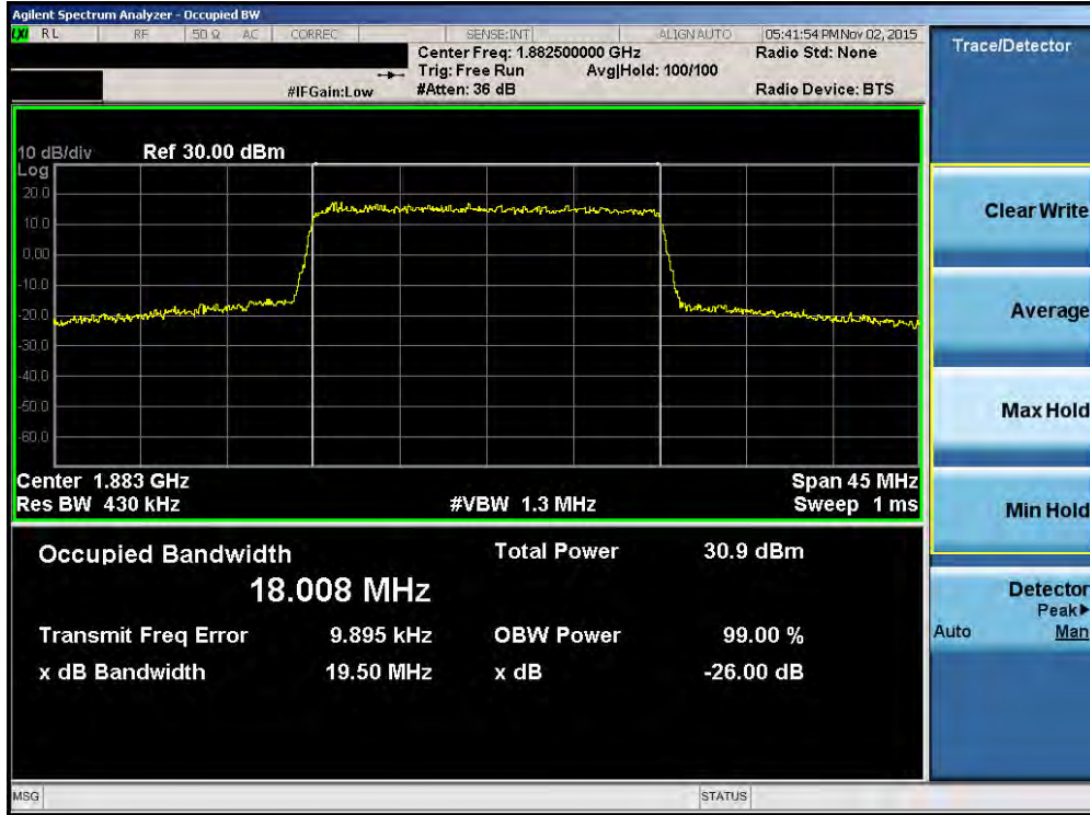
Plot 7-41. Occupied Bandwidth Plot (Band 2/25 – 20.0MHz QPSK – RB Size 100)
