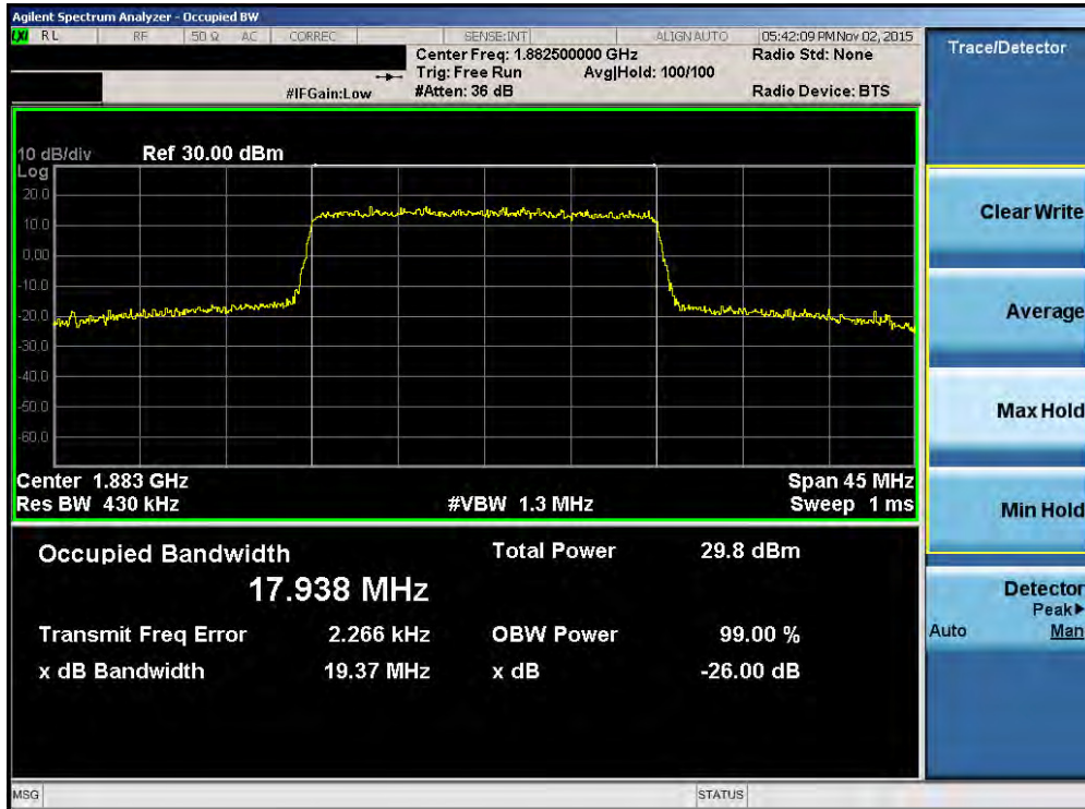
Plot 7-42. Occupied Bandwidth Plot (Band 2/25 – 20.0MHz 16-QAM – RB Size 100)
