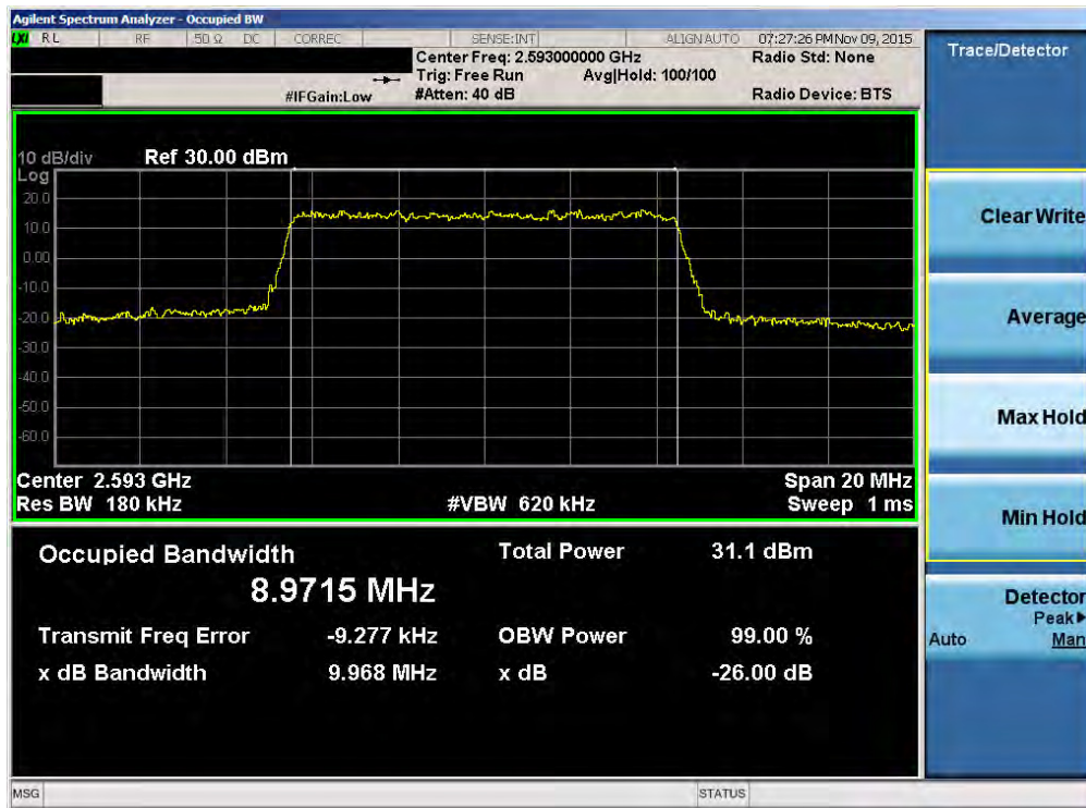
Plot 7-46. Occupied Bandwidth Plot (Band 41 – 10.0MHz 16-QAM – RB Size 50)
