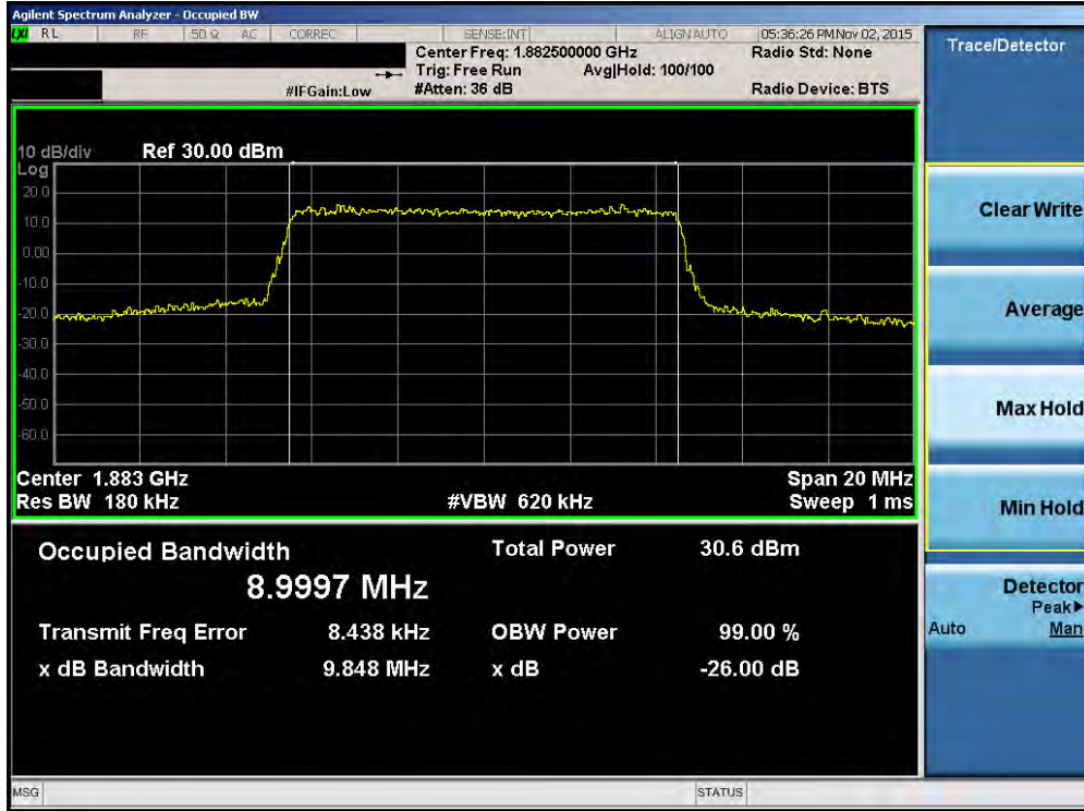
Plot 7-37. Occupied Bandwidth Plot (Band 2/25 – 10.0MHz QPSK – RB Size 50)
