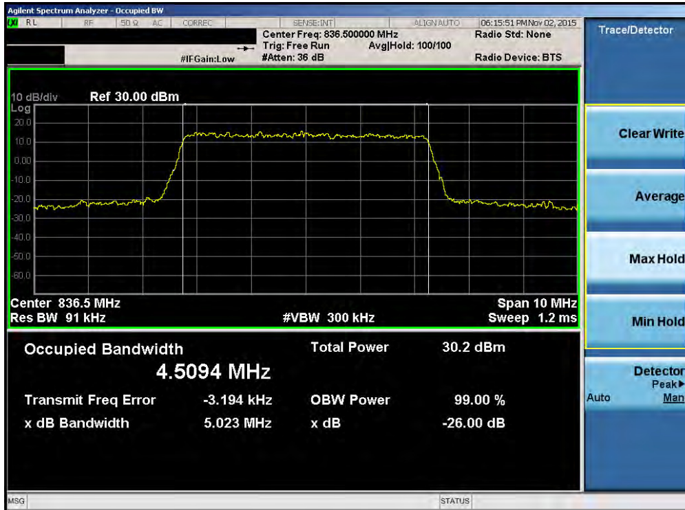
Plot 7-14. Occupied Bandwidth Plot (Band 5/26 – 5.0MHz 16-QAM – RB Size 25)
