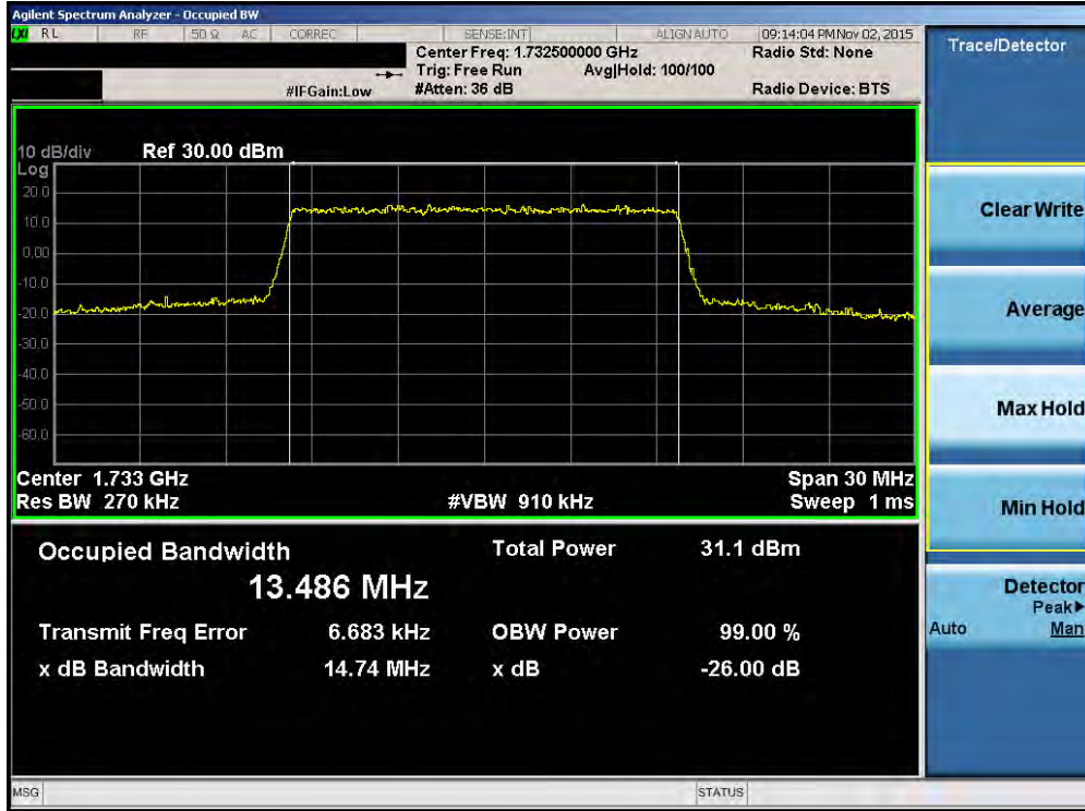
Plot 7-27. Occupied Bandwidth Plot (Band 4 – 15.0MHz QPSK – RB Size 75)
