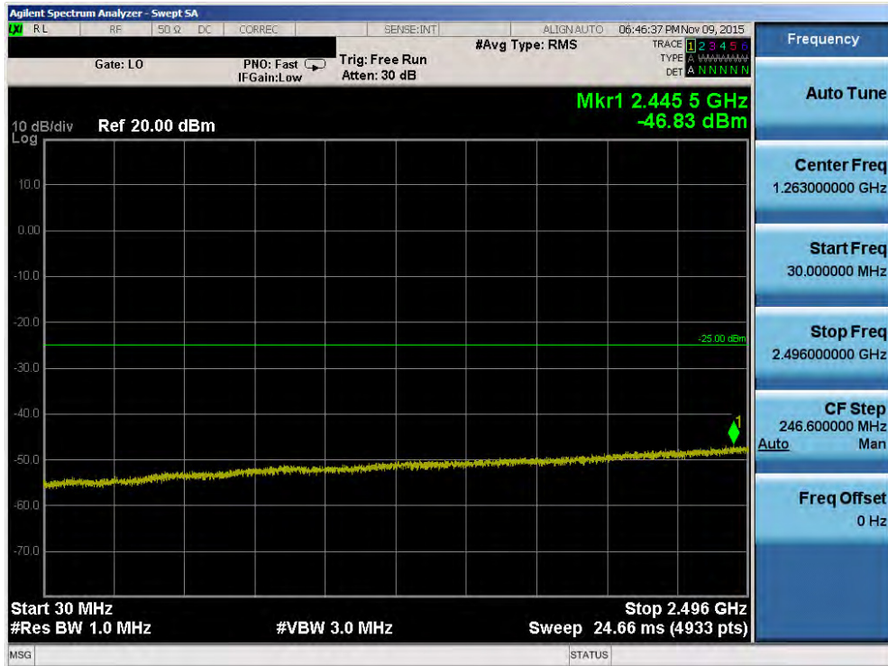
Plot 7-90. Conducted Spurious Plot (Band 41 – 5.0MHz QPSK – RB Size 1, RB Offset 0 – Mid Channel)
