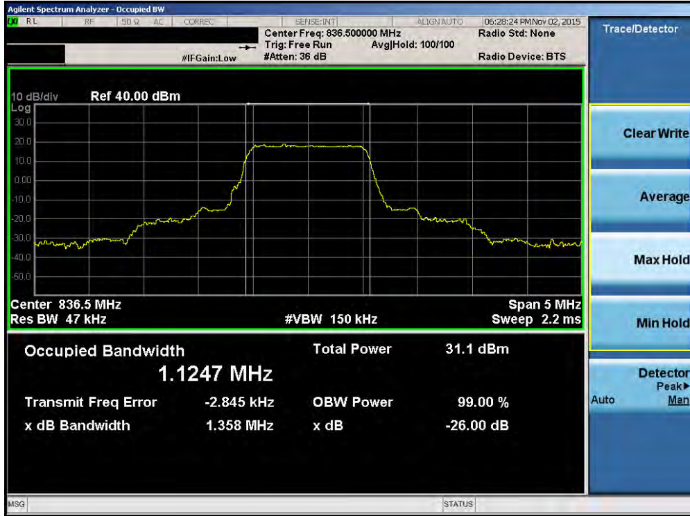
Plot 7-9. Occupied Bandwidth Plot (Band 5/26 – 1.4MHz QPSK – RB Size 6)
