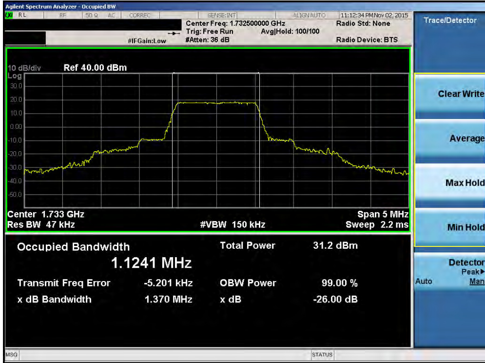
Plot 7-19. Occupied Bandwidth Plot (Band 4 – 1.4MHz QPSK – RB Size 6)
