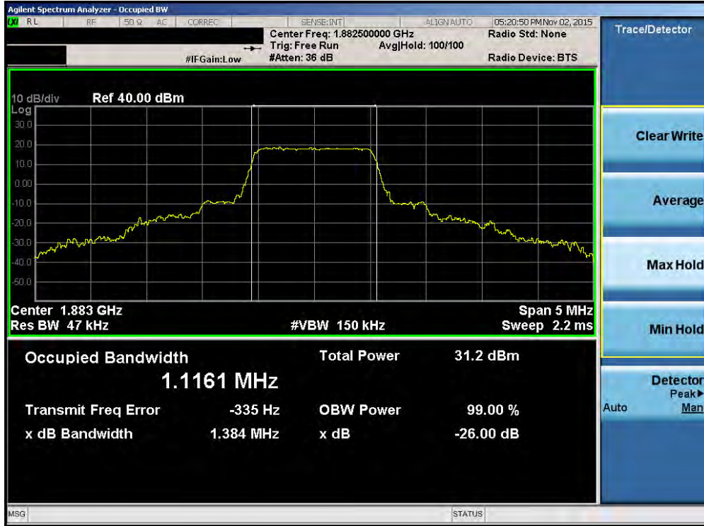
Plot 7-31. Occupied Bandwidth Plot (Band 2/25 – 1.4MHz QPSK – RB Size 6)
