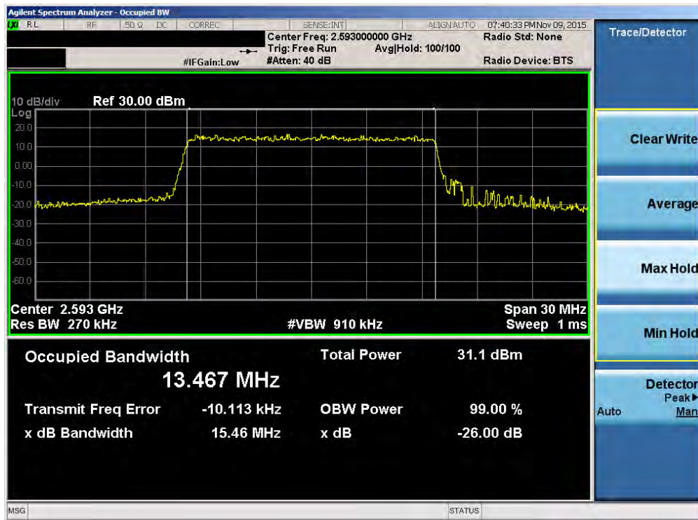
Plot 7-48. Occupied Bandwidth Plot (Band 41 – 15.0MHz 16-QAM – RB Size 75)
