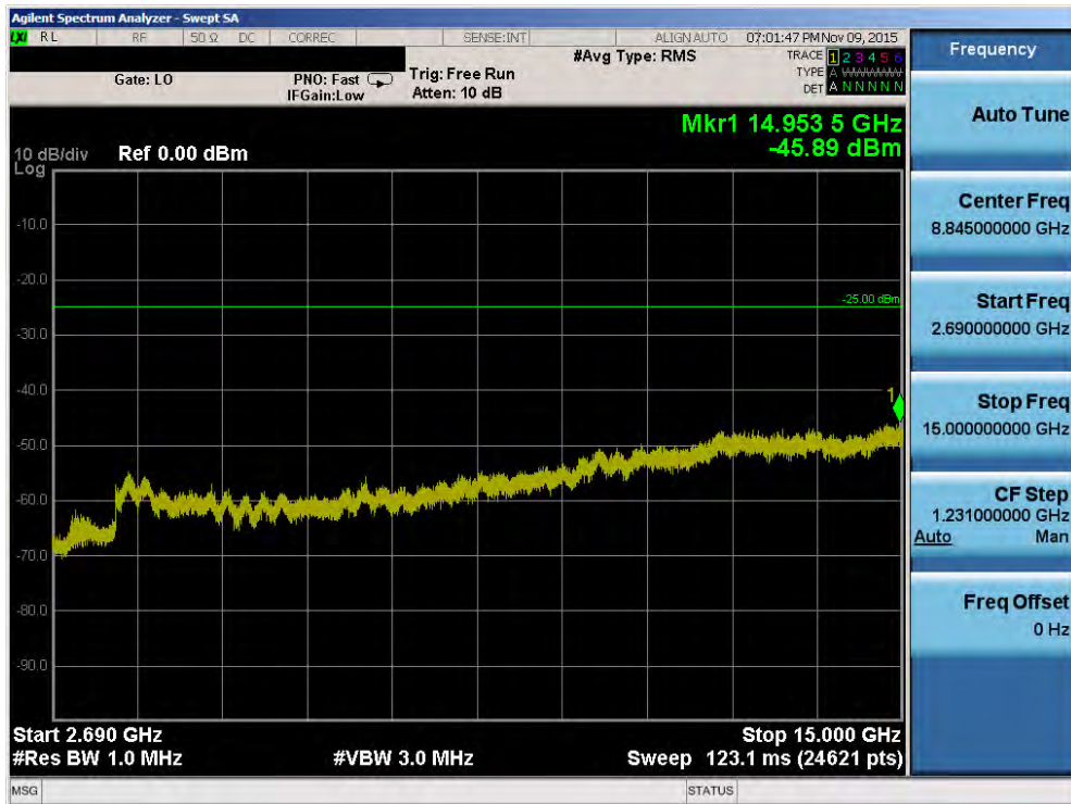
Plot 7-88. Conducted Spurious Plot (Band 41 – 5.0MHz QPSK – RB Size 1, RB Offset 0 – Low Channel)
