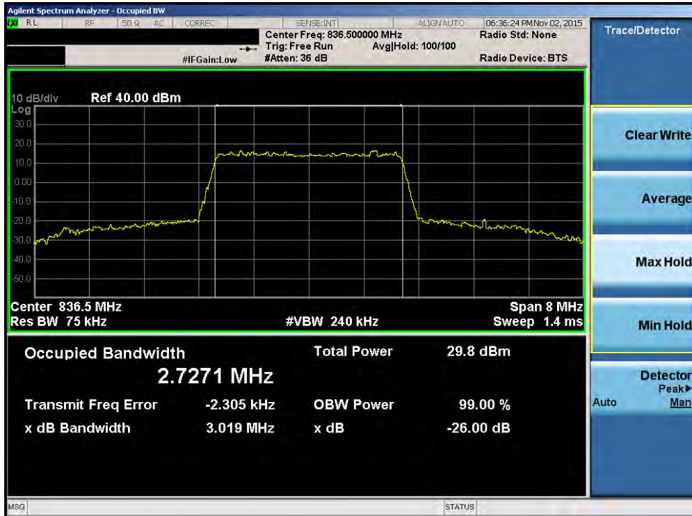
Plot 7-12. Occupied Bandwidth Plot (Band 5/26 – 3.0MHz 16-QAM – RB Size 15)
