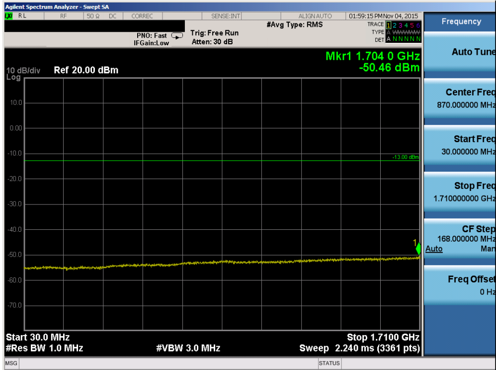
Plot 7-58. Conducted Spurious Plot (AWS WCDMA Mode – Ch. 1412)
