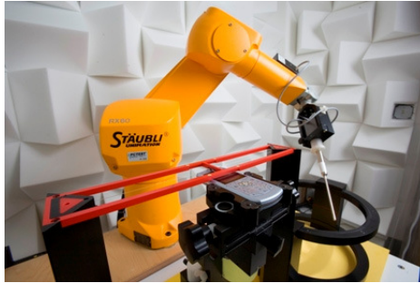
Figure 5-3 SPEAG Robotic System
