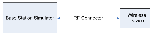
Figure 9-1 Power Measurement Setup
