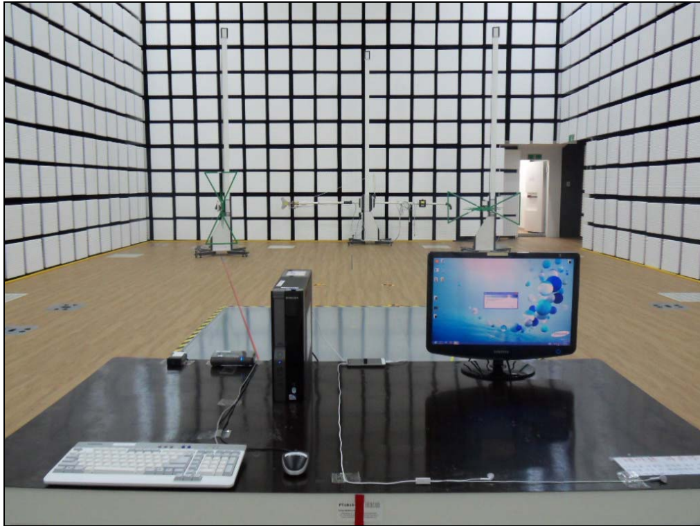
[ Radiated Disturbance for Below 1 GHz – Front ]
