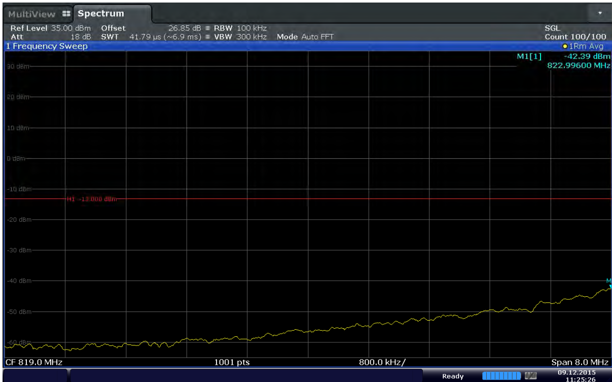
Plot 6-21. Lower Band Edge Plot (Band5 – 1.4MHz – QPSK – RB Size 6)
