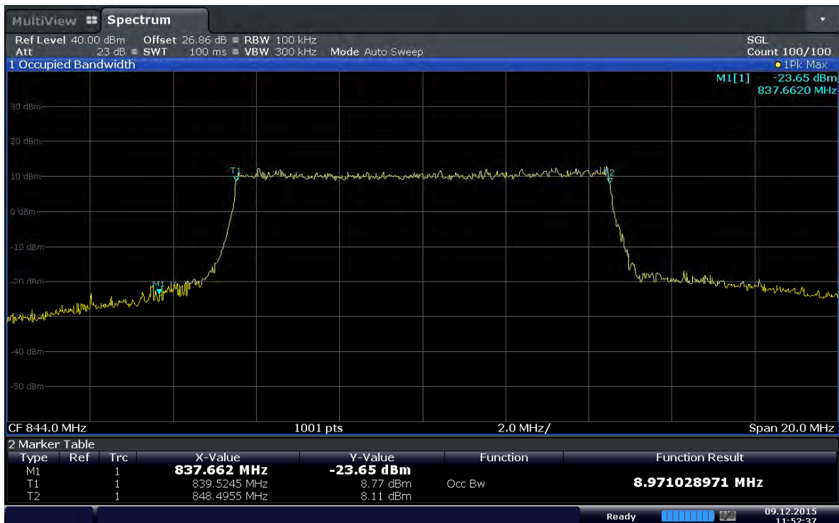
Plot 6-8. Occupied Bandwidth Plot (Band 5 - 10.0MHz 16QAM - RB Size 50)
