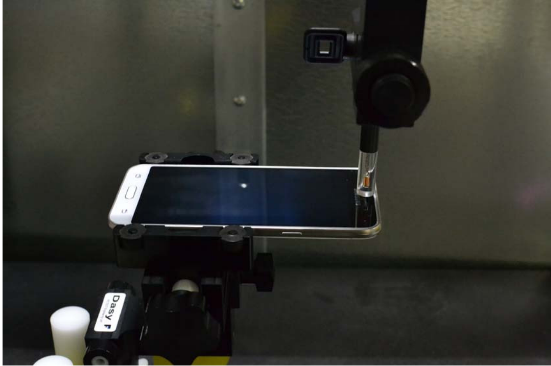
Figure 14-1 Test Setup for Wireless Device
