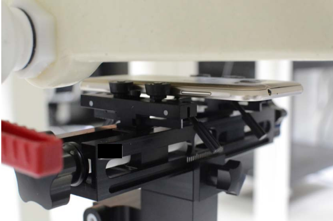
SAR Test Setup Photo 5 – Back Side at 1.5 cm (Body-Worn)
