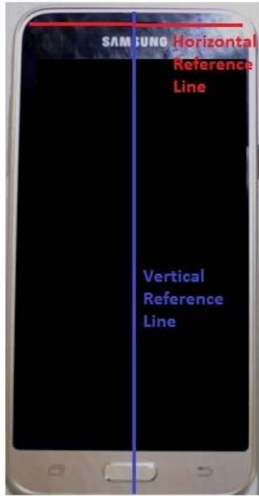
SAR Test Setup Photo 11 – DUT Reference Lines
