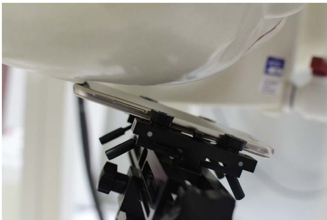
SAR Test Setup Photo 2 – Right Tilt
