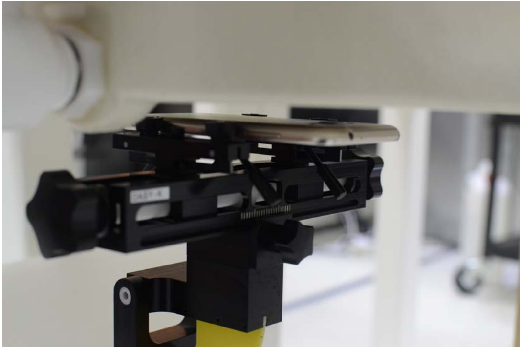
SAR Test Setup Photo 6 – Back Side at 1.0 cm (Hotspot)
