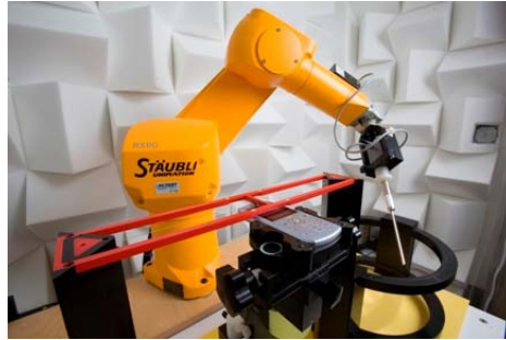
Figure 4-3 SPEAG Robotic System
