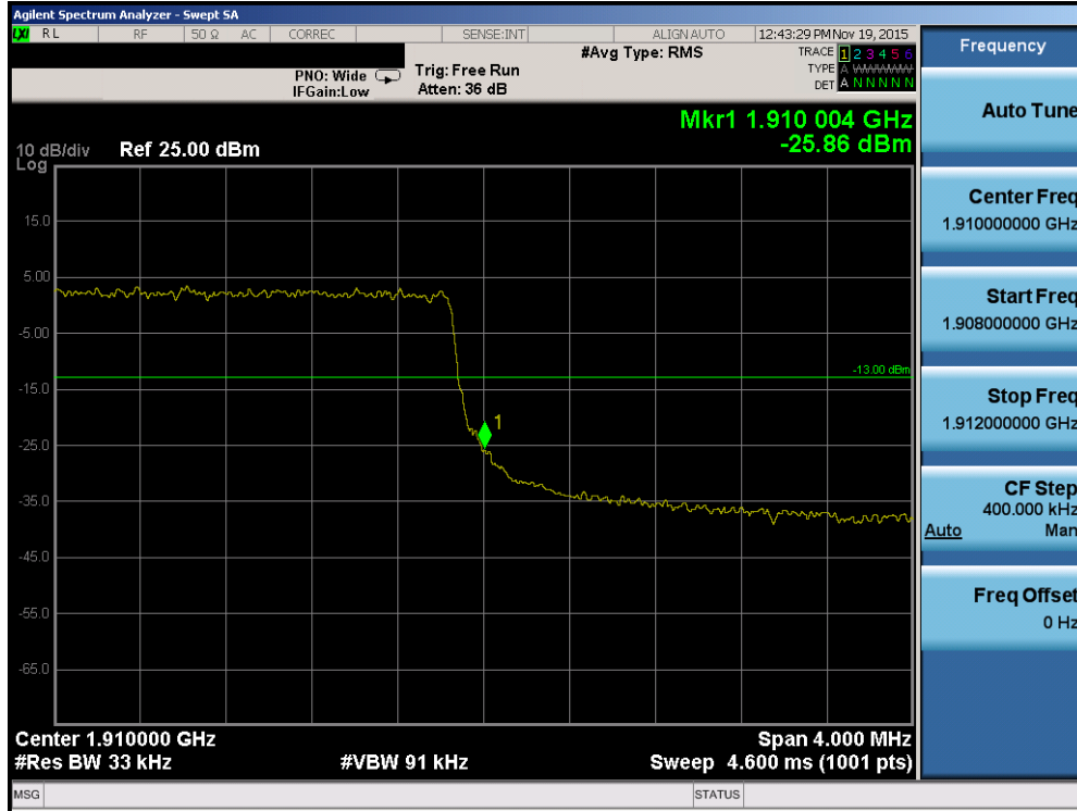
Plot 7-129. Upper Band Edge Plot (Band 2 – 3.0MHz QPSK – RB Size 15)
