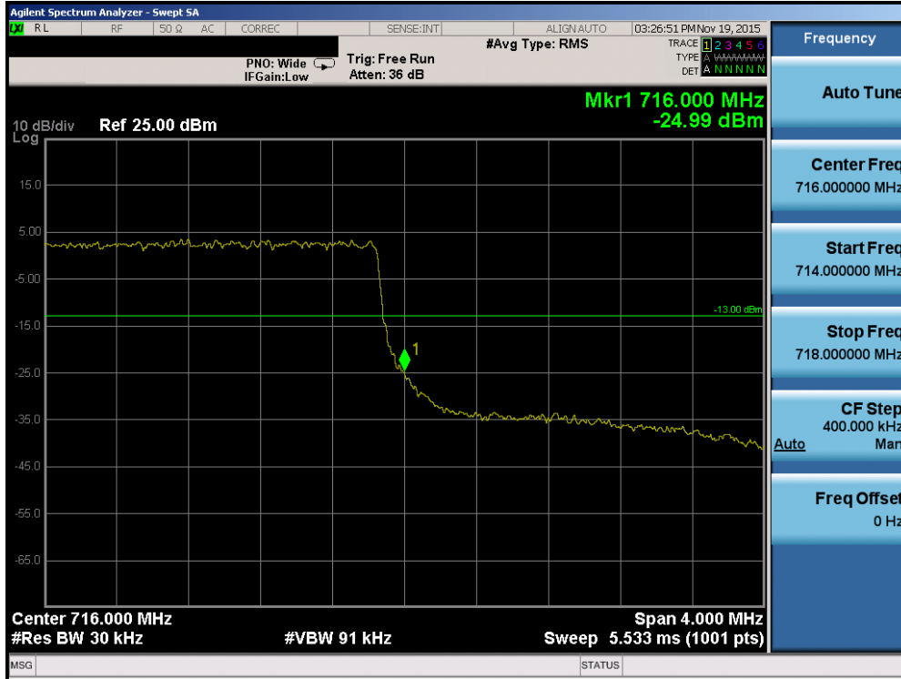
Plot 7-83. Upper Band Edge Plot (Band 12 – 3.0MHz QPSK – RB Size 15)
