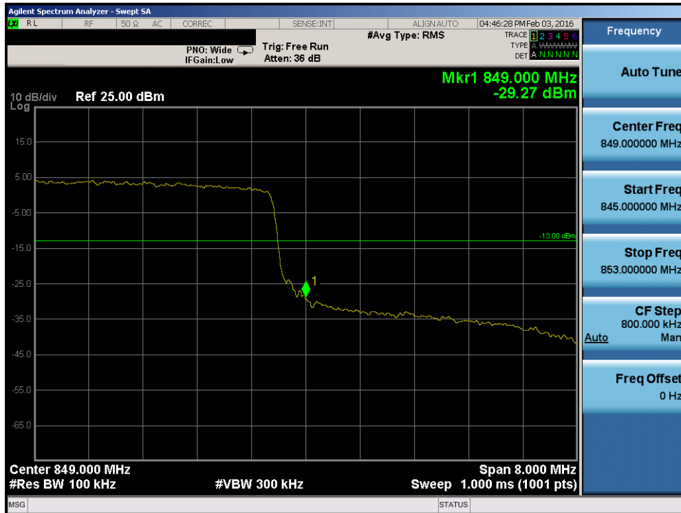
Plot 7-98. Upper Band Edge Plot (Band 5 – 10.0MHz QPSK – RB Size 50)
