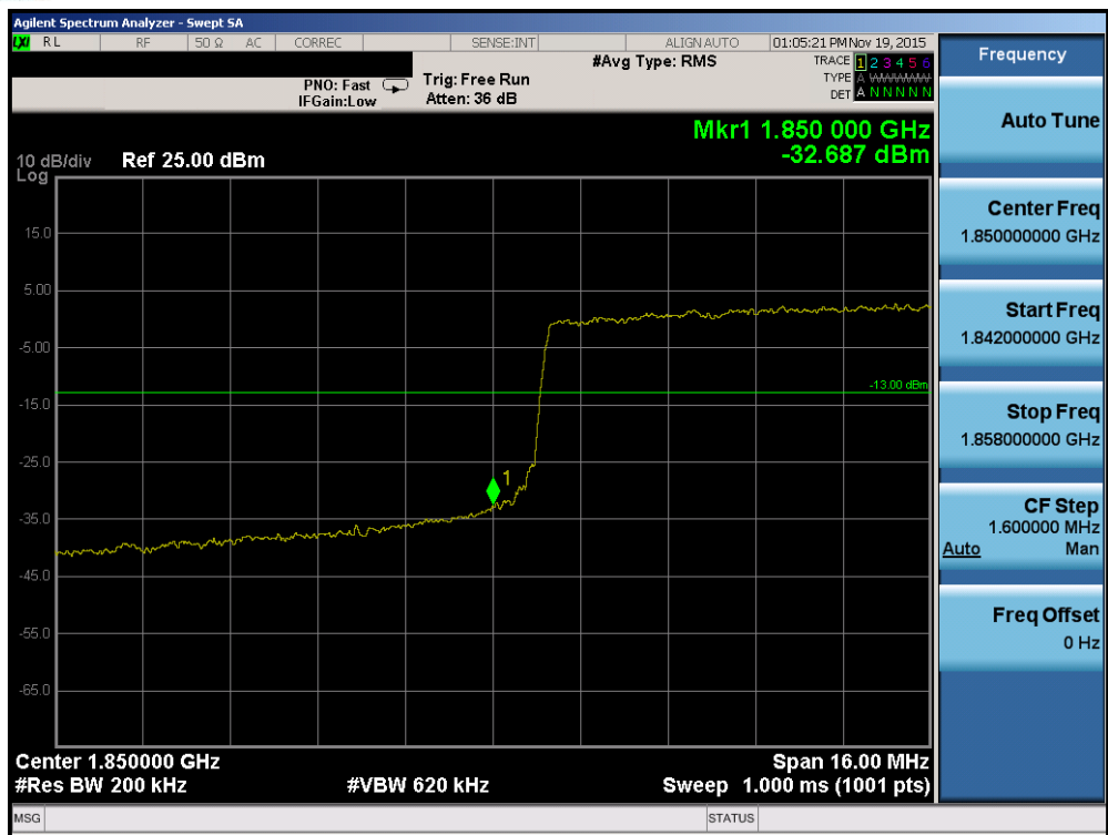
Plot 7-143. Lower Band Edge Plot (Band 2 – 20.0MHz QPSK – RB Size 100)
