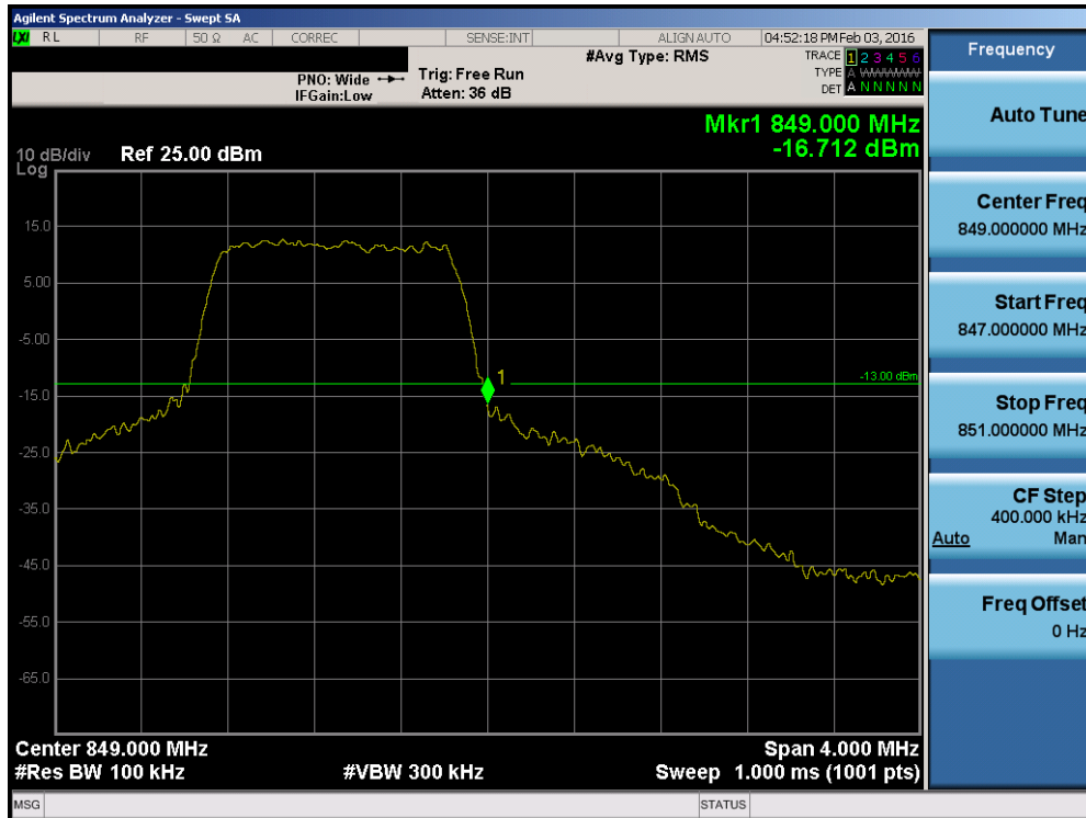
Plot 7-92. Upper Band Edge Plot (Band 5 – 1.4MHz QPSK – RB Size 6)
