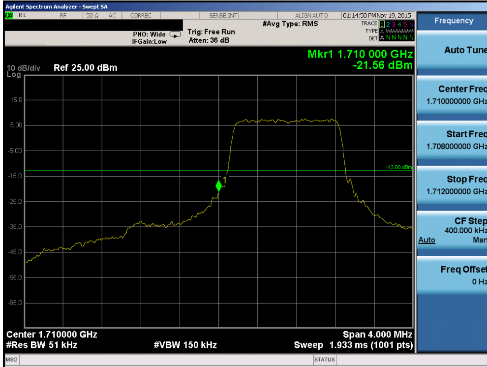
Plot 7-99. Lower Band Edge Plot (Band 4 – 1.4MHz QPSK – RB Size 6)
