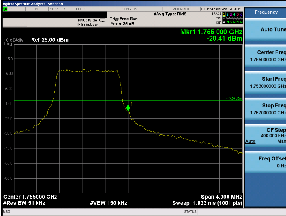
Plot 7-101. Upper Band Edge Plot (Band 4 – 1.4MHz QPSK – RB Size 6)
