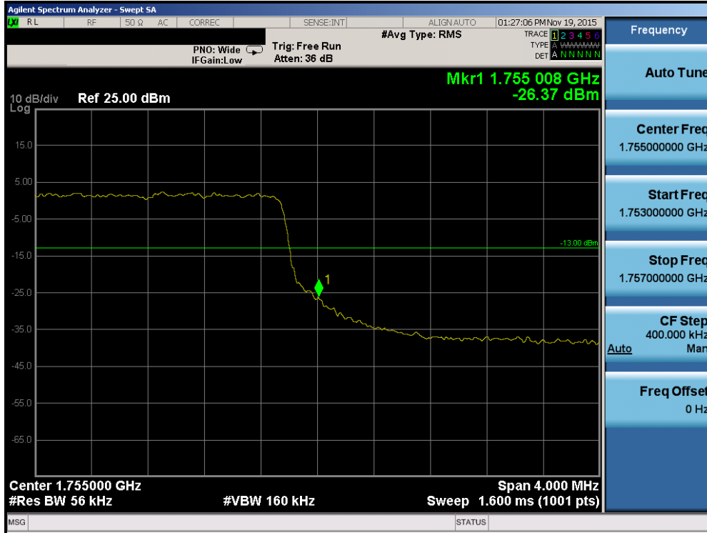
Plot 7-109. Upper Band Edge Plot (Band 4 – 5.0MHz QPSK – RB Size 25)
