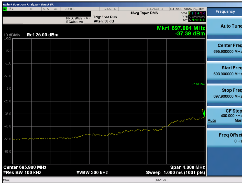
Plot 7-78. Lower Extended Band Edge Plot (Band 12 – 1.4MHz QPSK – RB Size 6)
