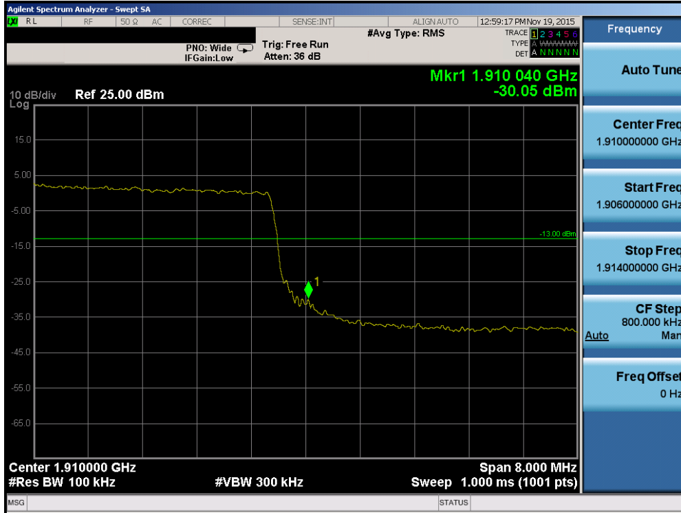
Plot 7-137. Upper Band Edge Plot (Band 2 – 10.0MHz QPSK – RB Size 50)
