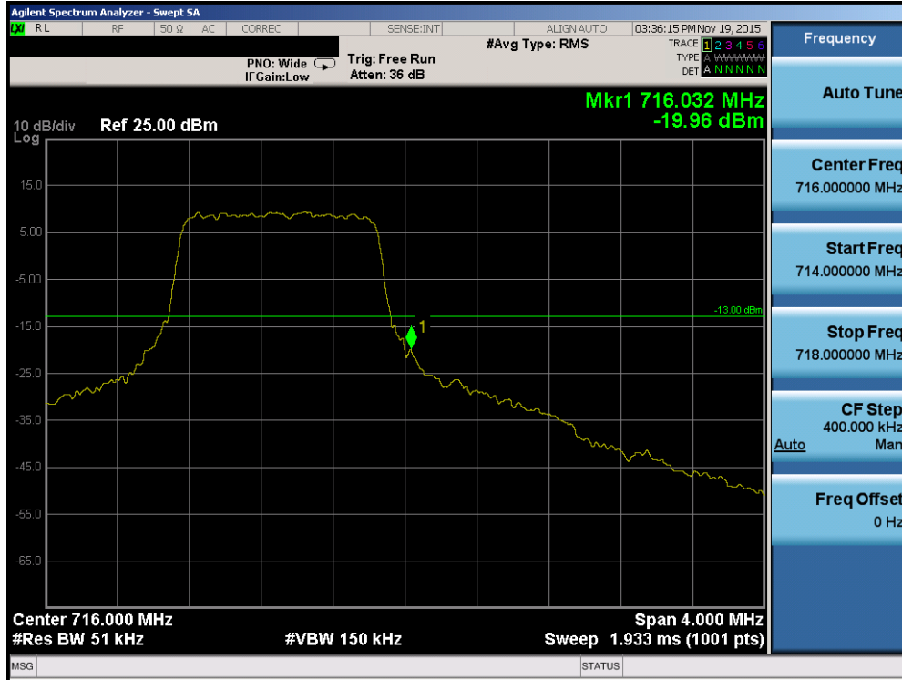
Plot 7-79. Upper Band Edge Plot (Band 12 – 1.4MHz QPSK – RB Size 6)
