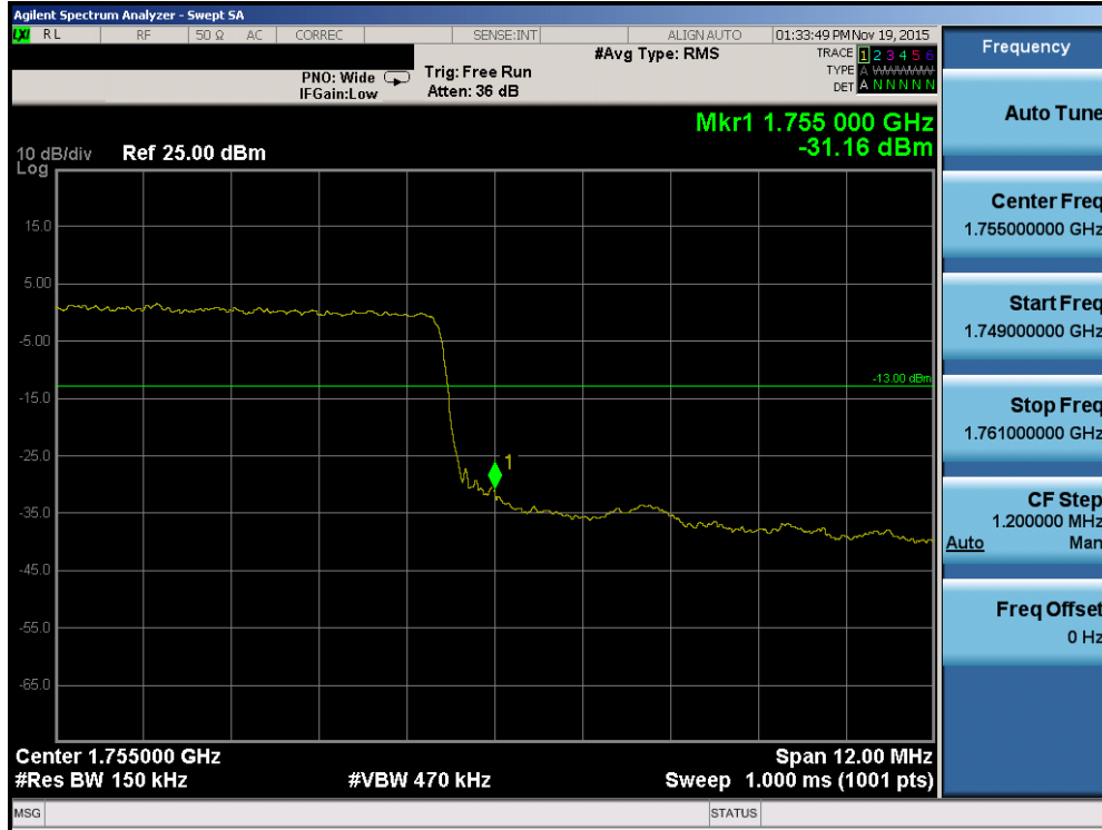
Plot 7-117. Upper Band Edge Plot (Band 4 – 15.0MHz QPSK – RB Size 75)
