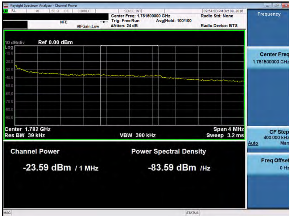
Plot 7-146. Upper Extended Band Edge Plot (Band 66 - 3.0MHz QPSK - Full RB Configuration)
