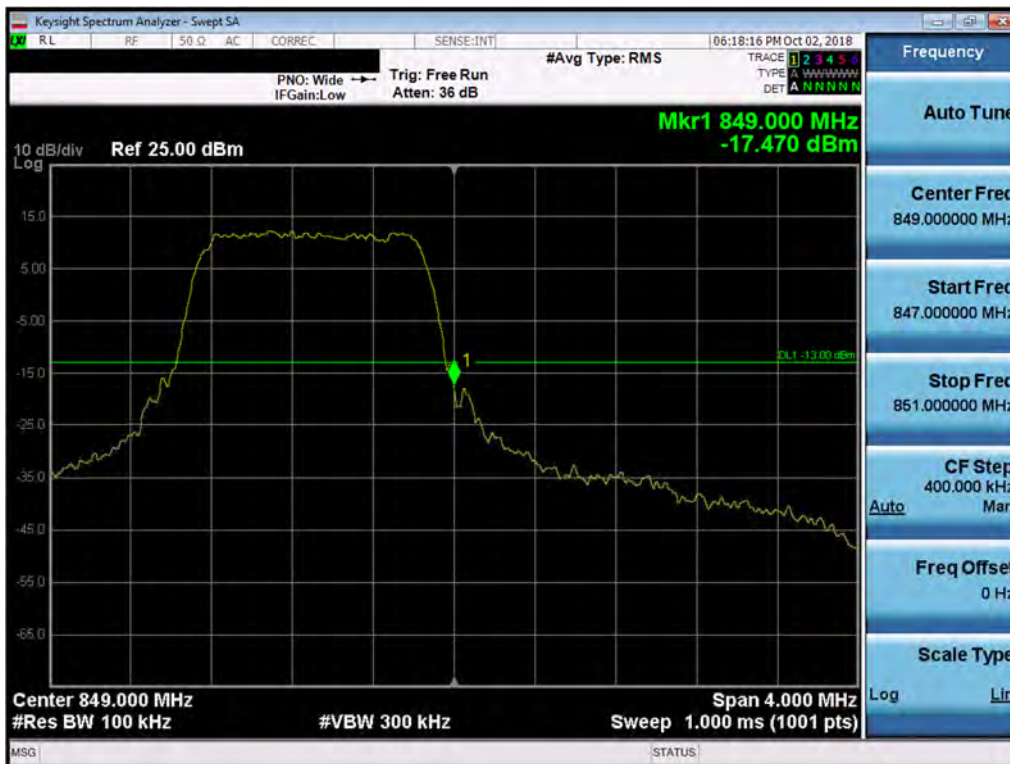
Plot 7-128. Upper Band Edge Plot (Band 5 - 1.4MHz QPSK - Full RB Configuration)
