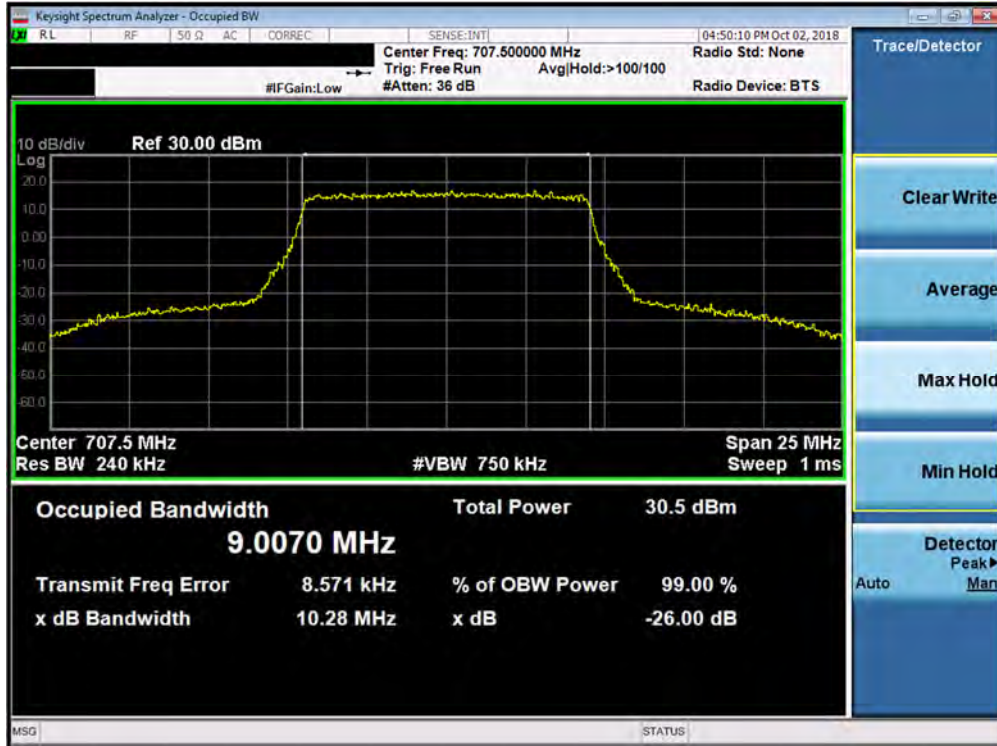
Plot 7-15. Occupied Bandwidth Plot (Band 12 - 10.0MHz QPSK - Full RB Configuration)
