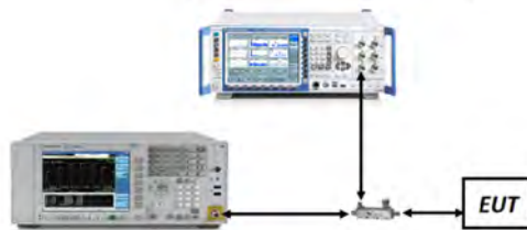
Figure 7-1. Test Instrument & Measurement Setup
