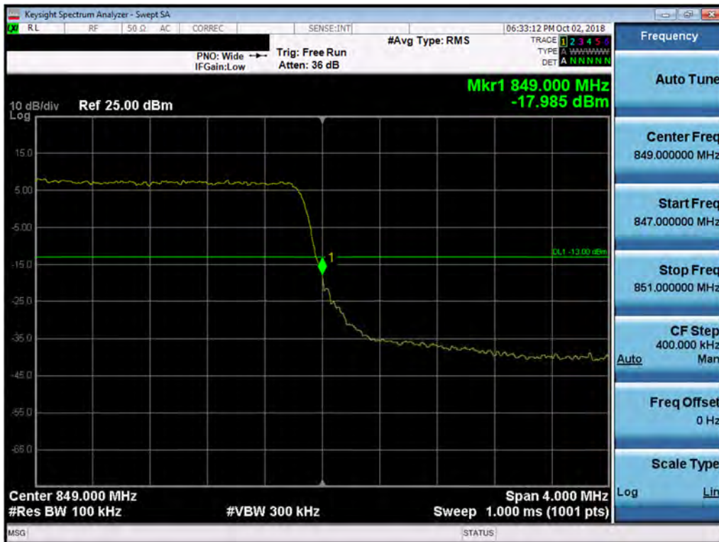
Plot 7-130. Upper Band Edge Plot (Band 5 - 3.0MHz QPSK - Full RB Configuration)
