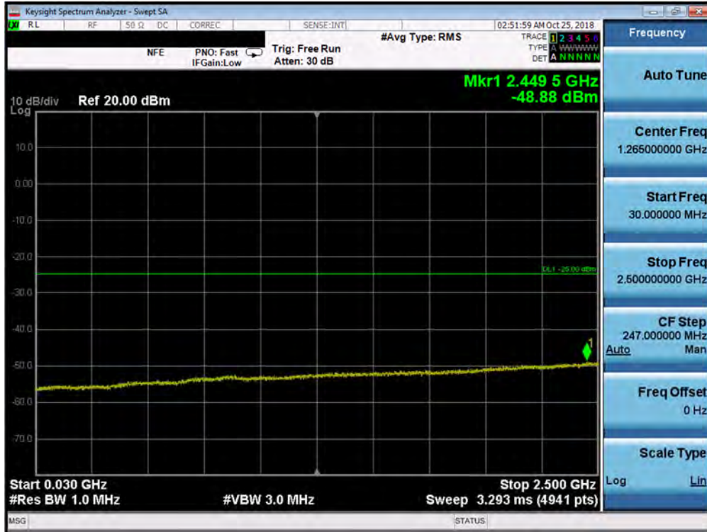
Plot 7-108. Conducted Spurious Plot (Band 7 - 20.0MHz QPSK - RB Size 1, RB Offset 0 - High Channel)
