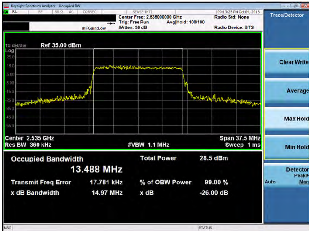
Plot 7-54. Occupied Bandwidth Plot (Band 7 - 15.0MHz 16-QAM - Full RB Configuration)
