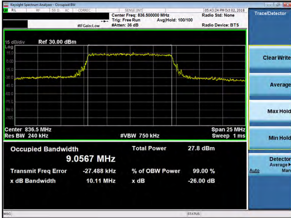
Plot 7-23. Occupied Bandwidth Plot (Band 5 - 10.0MHz QPSK - Full RB Configuration)
