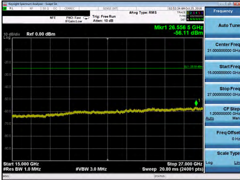
Plot 7-110. Conducted Spurious Plot (Band 7 - 20.0MHz QPSK - RB Size 1, RB Offset 0 - High Channel)
