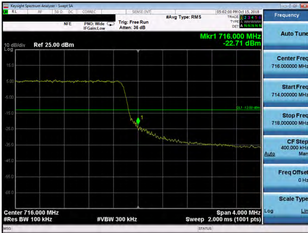
Plot 7-124. Upper Band Edge Plot (Band 12 - 5.0MHz QPSK - Full RB Configuration)
