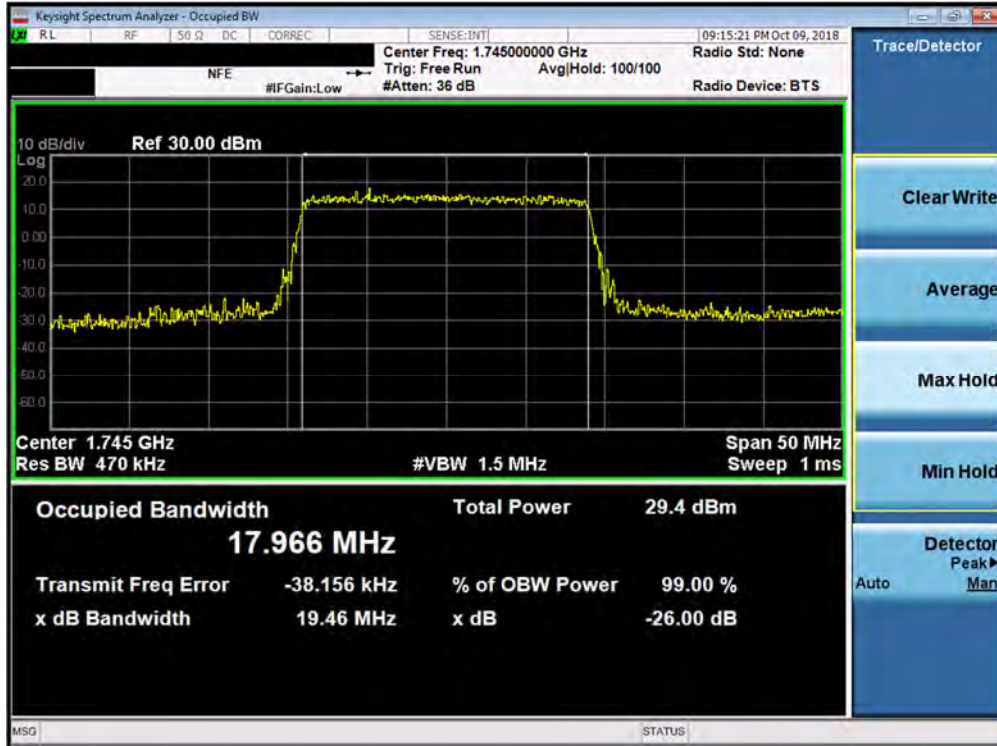
Plot 7-35. Occupied Bandwidth Plot (Band 66/4 - 20.0MHz QPSK - Full RB Configuration)
