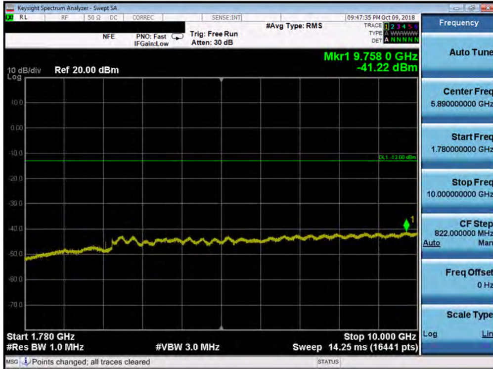
Plot 7-88. Conducted Spurious Plot (Band 66/4 - 20.0MHz QPSK - RB Size 1, RB Offset 0 - Mid Channel)
