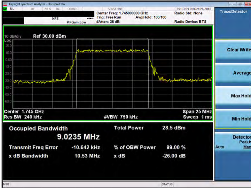
Plot 7-31. Occupied Bandwidth Plot (Band 66/4 - 10.0MHz QPSK - Full RB Configuration)
