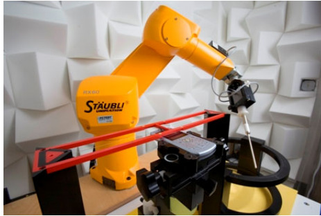
Figure 4-3 SPEAG Robotic System
