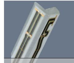
Figure 4-1 E-field Free-space Probe
