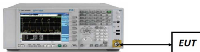
Figure 7-4. Test Instrument & Measurement Setup
