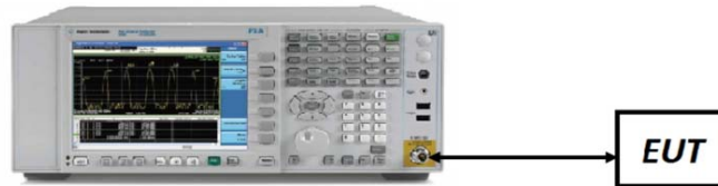
Figure 7-5. Test Instrument & Measurement Setup
