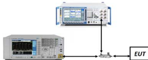
Figure 7-2. Test Instrument & Measurement Setup
