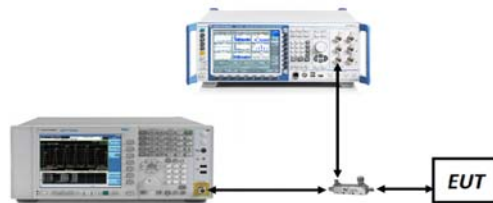
Figure 7-3. Test Instrument & Measurement Setup
