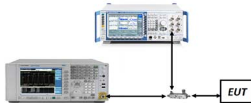
Figure 7-4. Test Instrument & Measurement Setup
