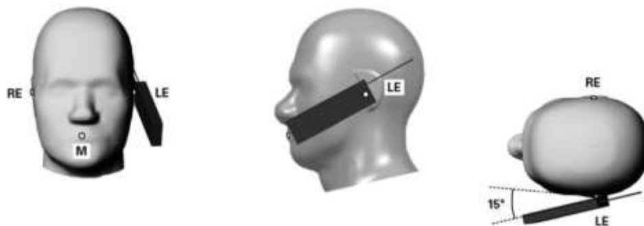
Figure 6.5. Tilt 15° position of the wireless device
