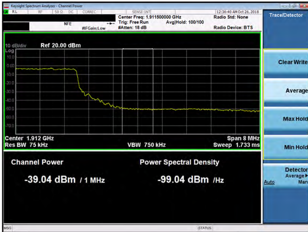
Plot 7-149. Upper Extended Band Edge Plot (Band 2 – 10.0MHz QPSK - Full RB Configuration)
