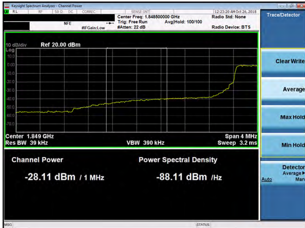
Plot 7-139. Lower Extended Band Edge Plot (Band 2 – 3.0MHz QPSK - Full RB Configuration)
