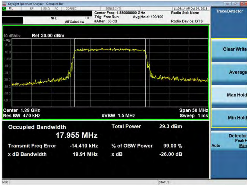
Plot 7-39. Occupied Bandwidth Plot (Band 2 - 20.0MHz QPSK - Full RB Configuration)
