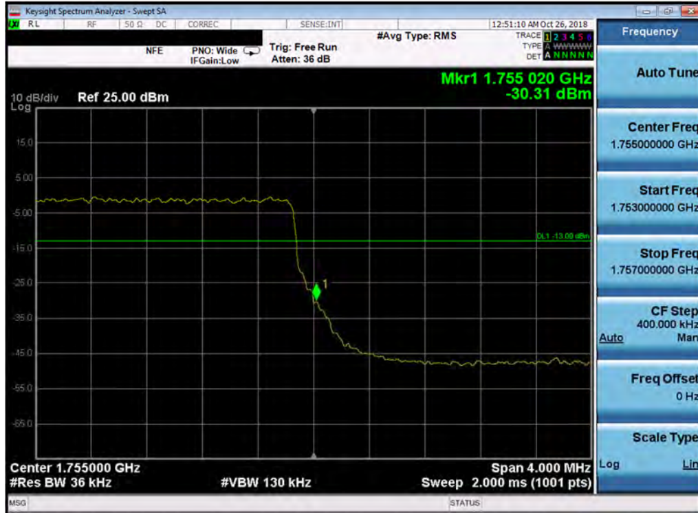
Plot 7-116. Upper Band Edge Plot (Band 4 - 3.0MHz QPSK - Full RB Configuration)
