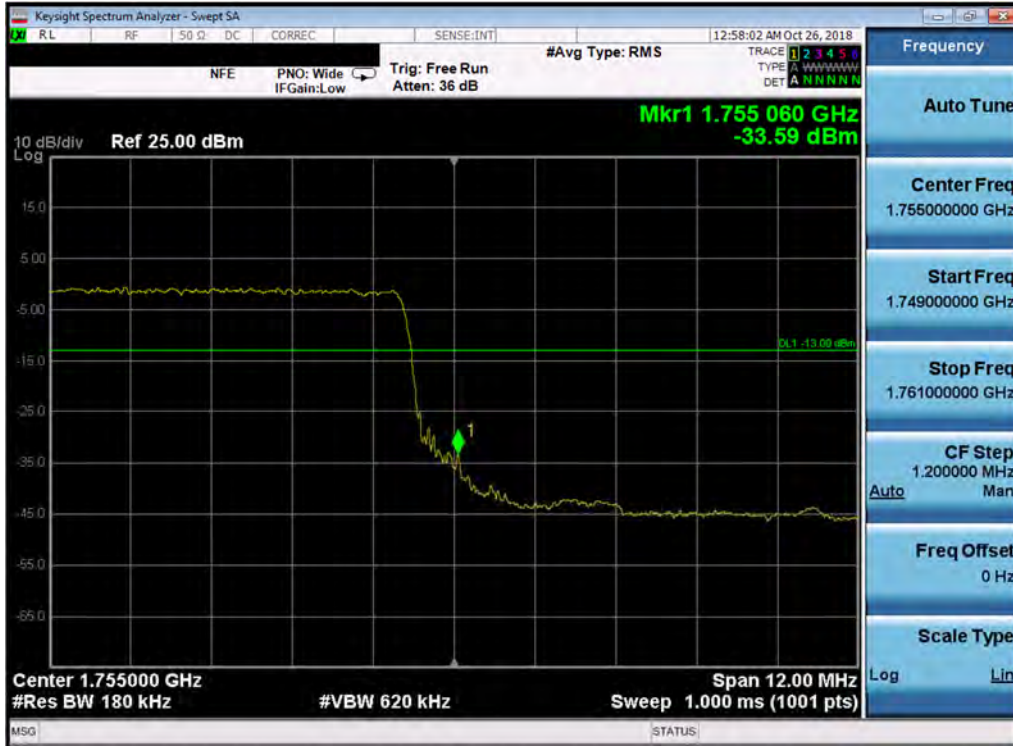
Plot 7-128. Upper Band Edge Plot (Band 4 - 15.0MHz QPSK - Full RB Configuration)
