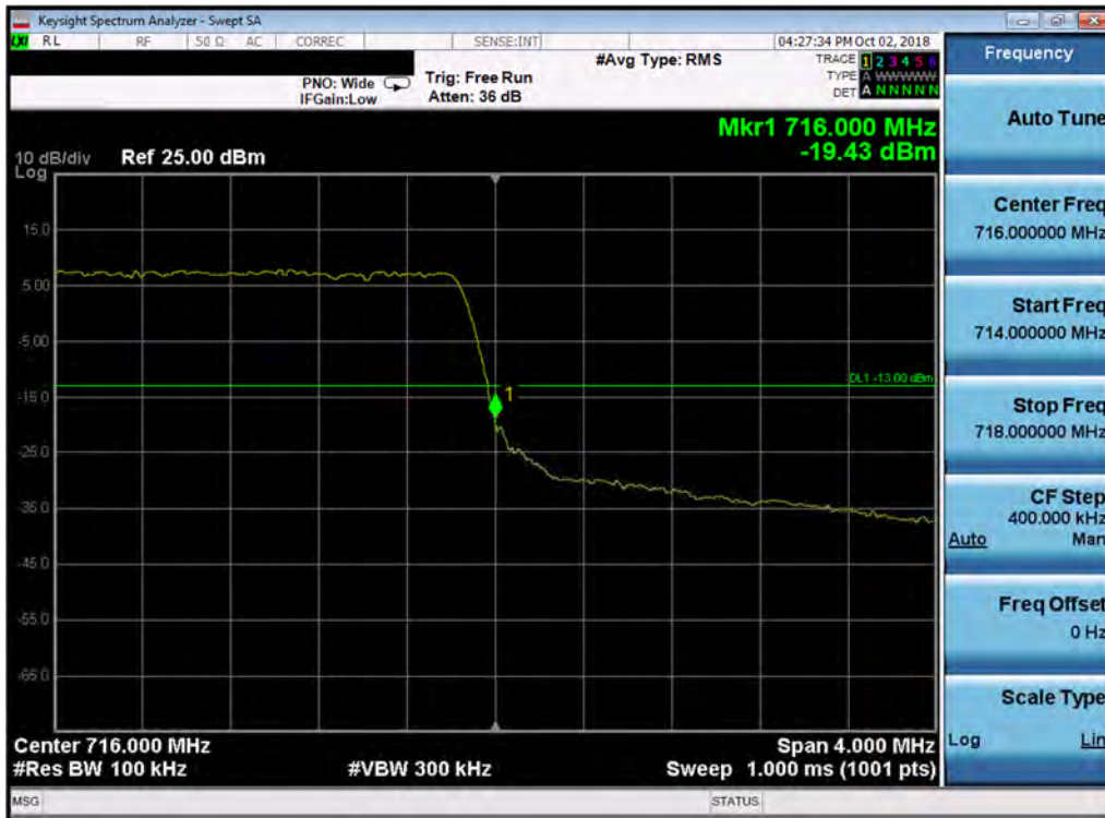
Plot 7-97. Upper Band Edge Plot (Band 12 - 3.0MHz QPSK - Full RB Configuration)
