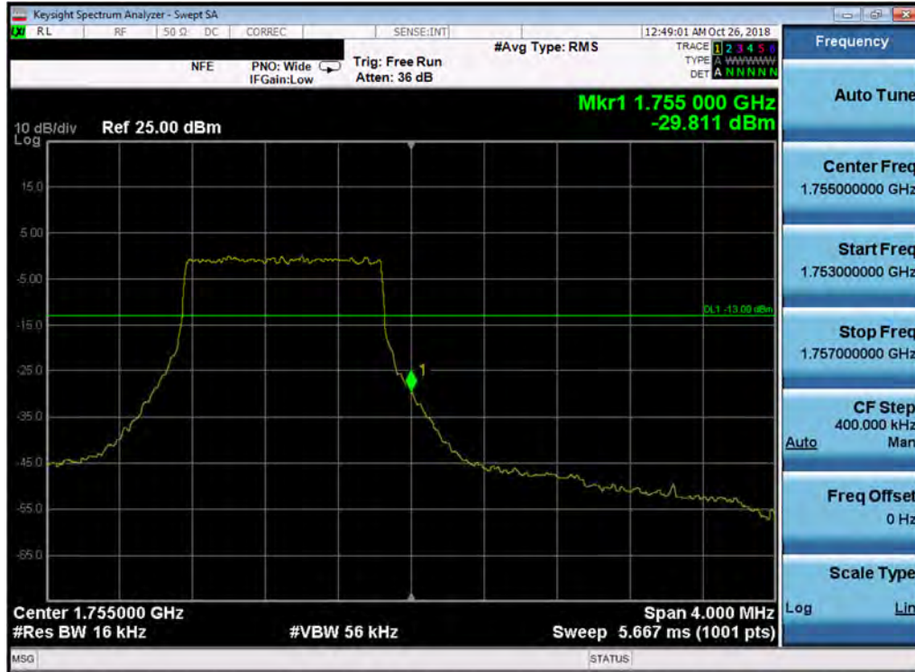
Plot 7-112. Upper Band Edge Plot (Band 4 - 1.4MHz QPSK - Full RB Configuration)
