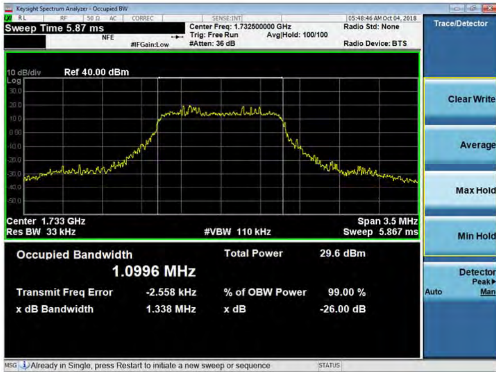
Plot 7-18. Occupied Bandwidth Plot (Band 4 - 1.4MHz 16-QAM - Full RB Configuration)
