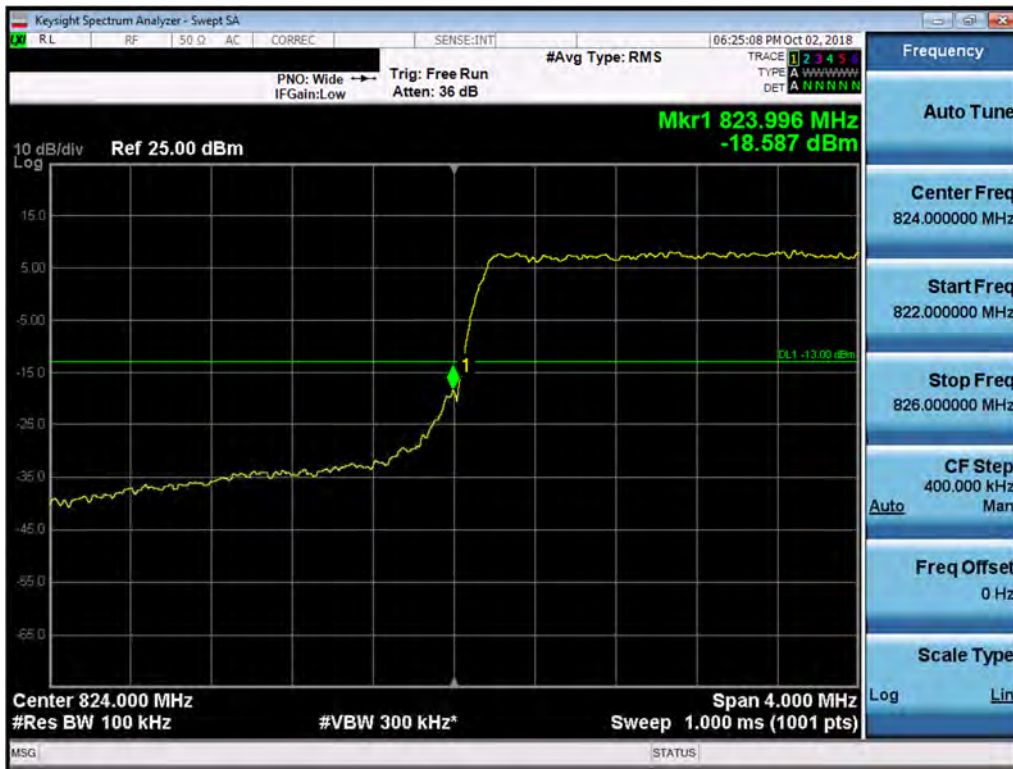
Plot 7-104. Lower Band Edge Plot (Band 5 - 3.0MHz QPSK - Full RB Configuration)
