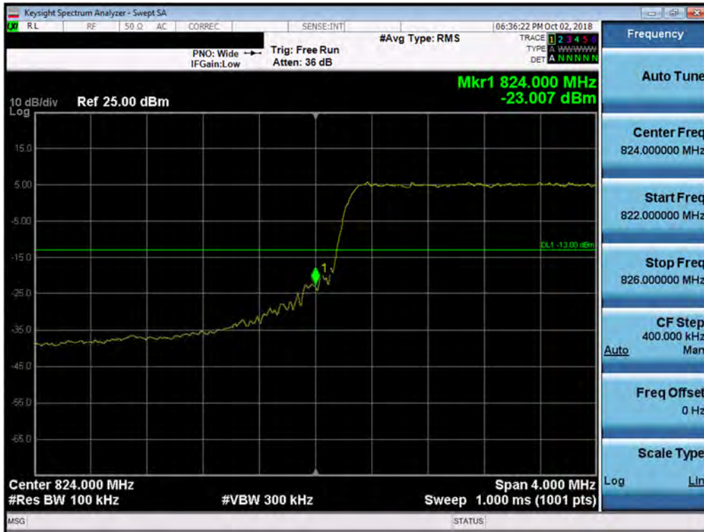
Plot 7-106. Lower Band Edge Plot (Band 5 - 5.0MHz QPSK - Full RB Configuration)
