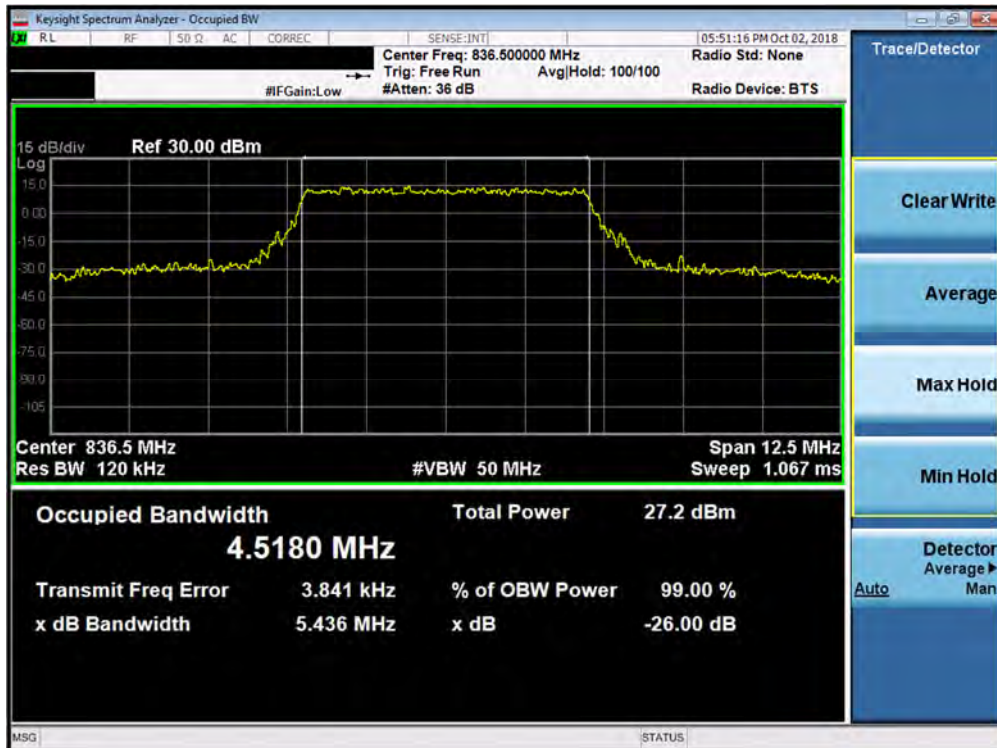
Plot 7-14. Occupied Bandwidth Plot (Band 5 - 5.0MHz 16-QAM - Full RB Configuration)
