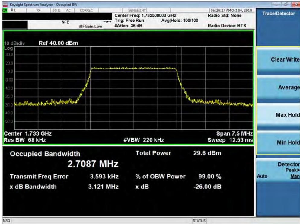
Plot 7-19. Occupied Bandwidth Plot (Band 4 - 3.0MHz QPSK - Full RB Configuration)
