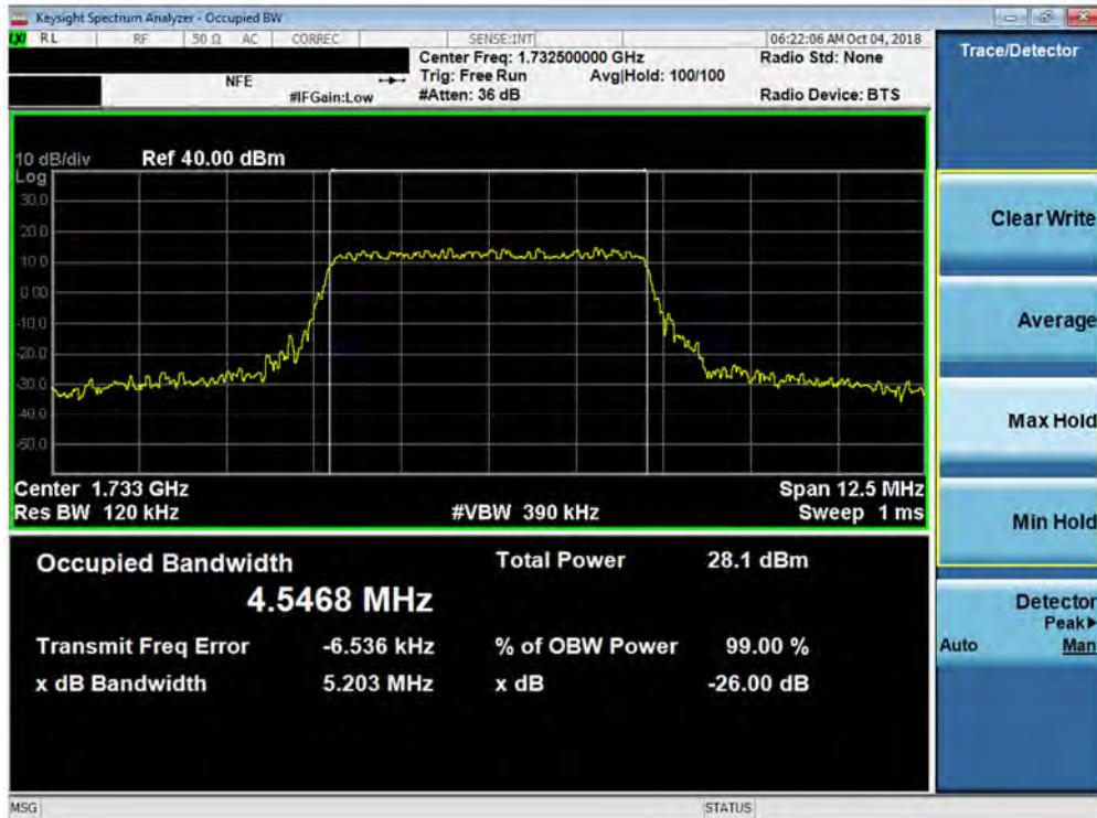
Plot 7-22. Occupied Bandwidth Plot (Band 4 - 5.0MHz 16-QAM - Full RB Configuration)
