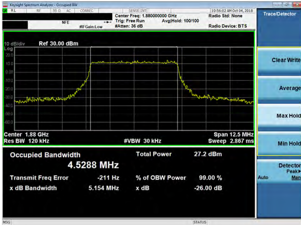
Plot 7-34. Occupied Bandwidth Plot (Band 2 - 5.0MHz 16-QAM - Full RB Configuration)
