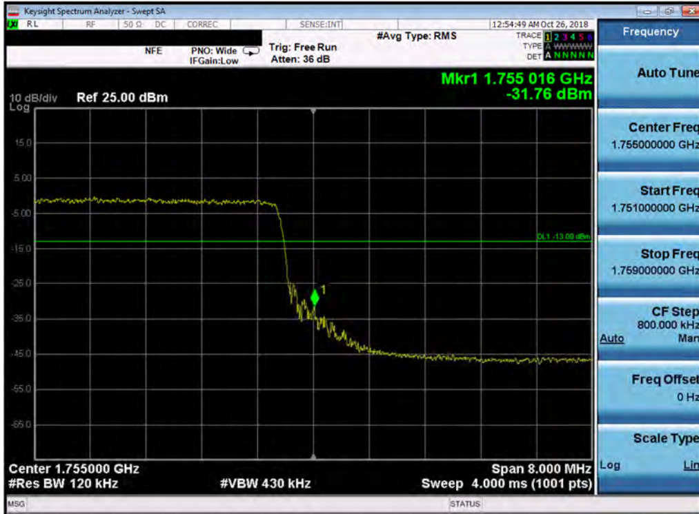
Plot 7-124. Upper Band Edge Plot (Band 4 - 10.0MHz QPSK - Full RB Configuration)
