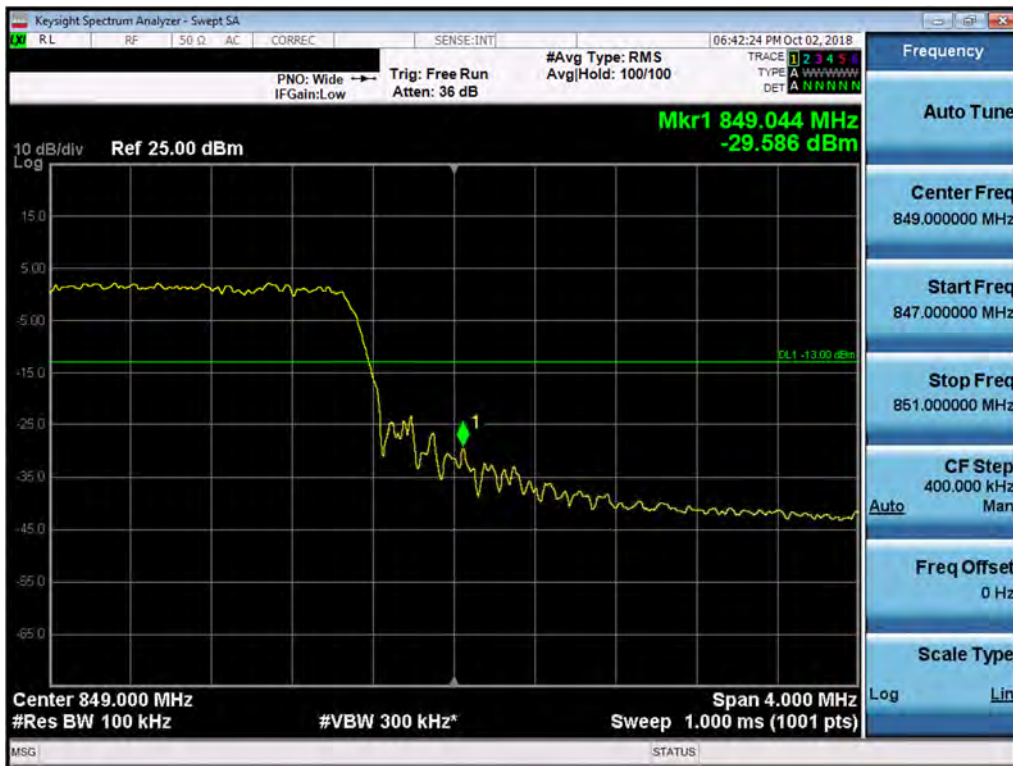
Plot 7-109. Upper Band Edge Plot (Band 5 - 10.0MHz QPSK - Full RB Configuration)
