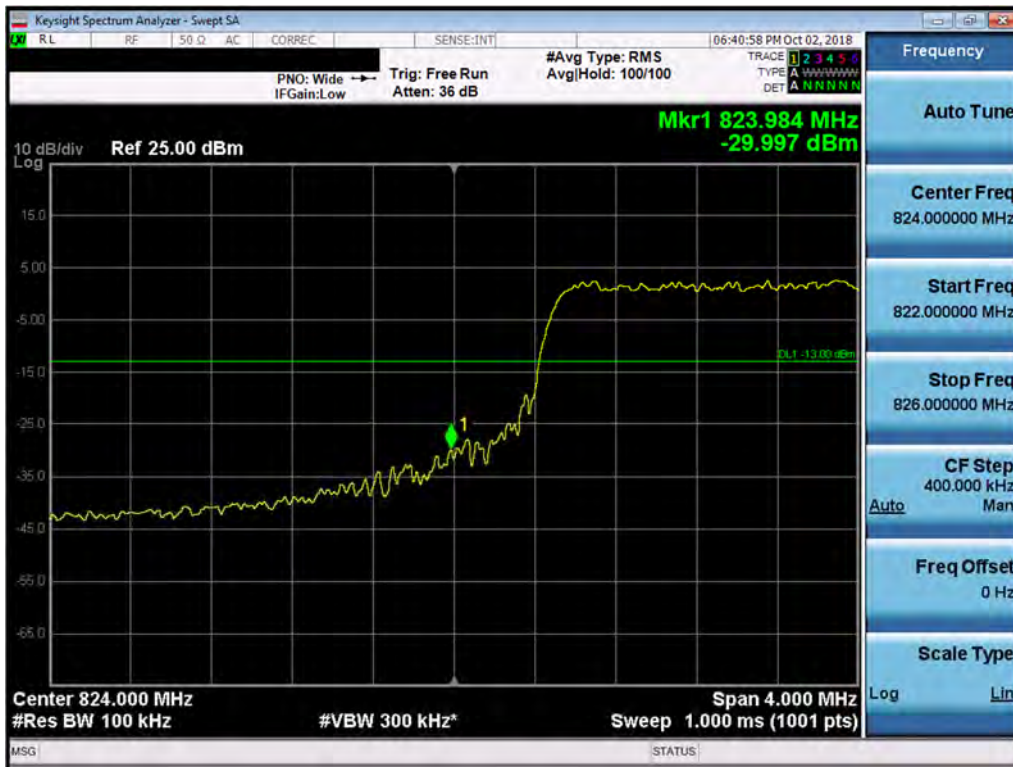
Plot 7-108. Lower Band Edge Plot (Band 5 - 10.0MHz QPSK - Full RB Configuration)
