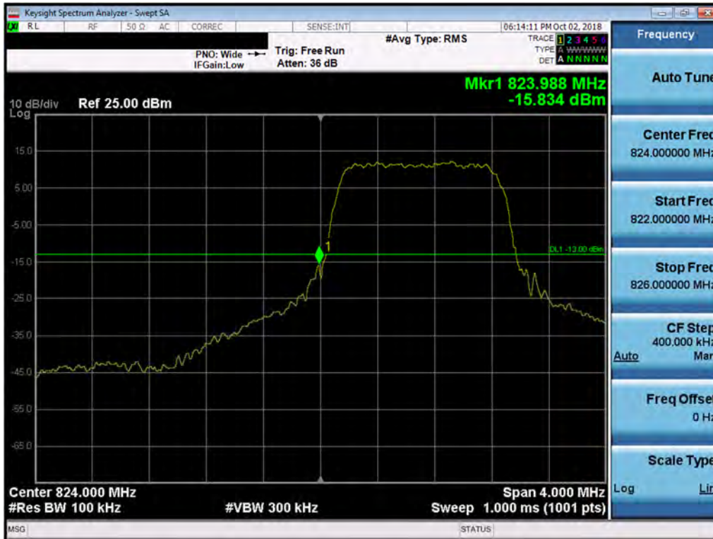
Plot 7-102. Lower Band Edge Plot (Band 5 - 1.4MHz QPSK - Full RB Configuration)
