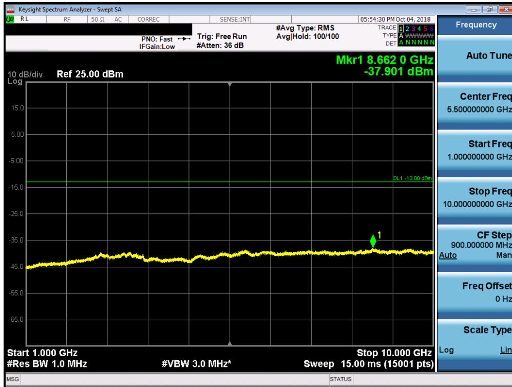
Plot 7-7. Conducted Spurious Plot (LTE Band 14, 10MHz QPSK – RB Size 1, RB Offset 0 – Mid Channel)
