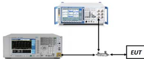
Figure 7-4. Test Instrument & Measurement Setup
