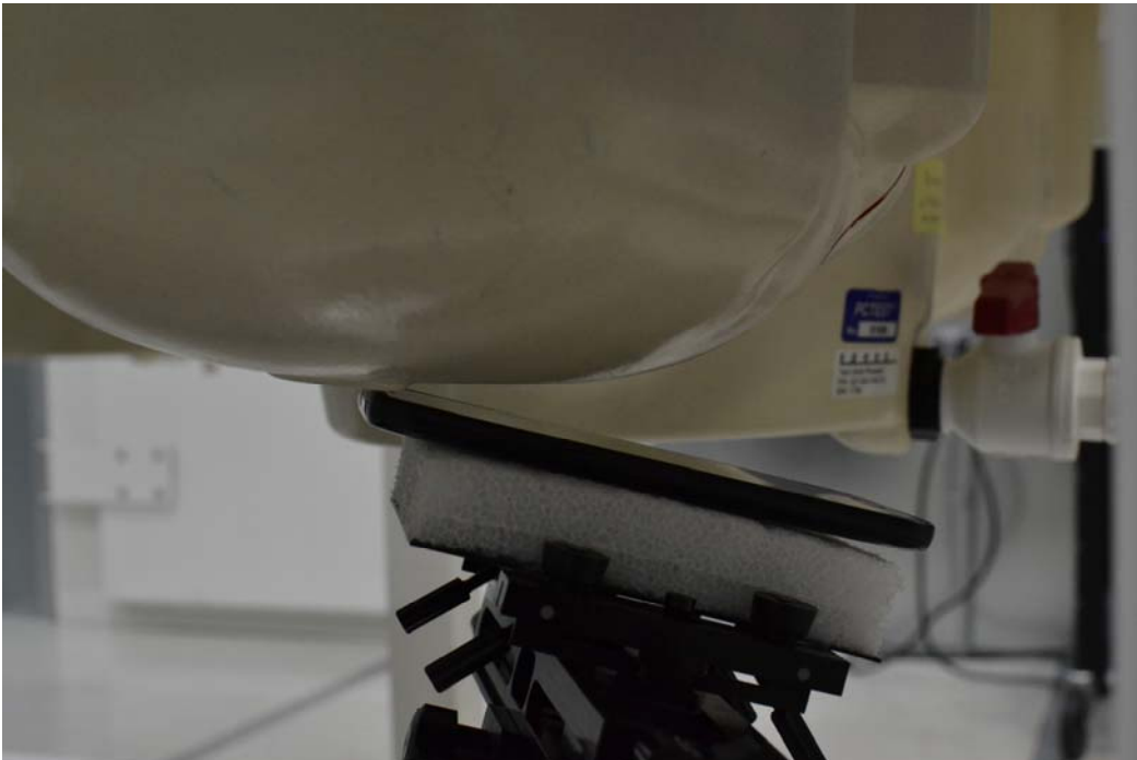
SAR Test Setup Photo 2 – Right Tilt
