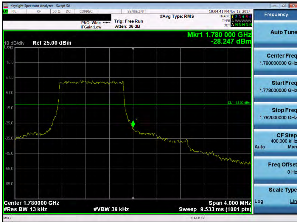
Plot 7-127. Upper Band Edge Plot (Band 66 - 1.4MHz QPSK - Full RB Configuration)
