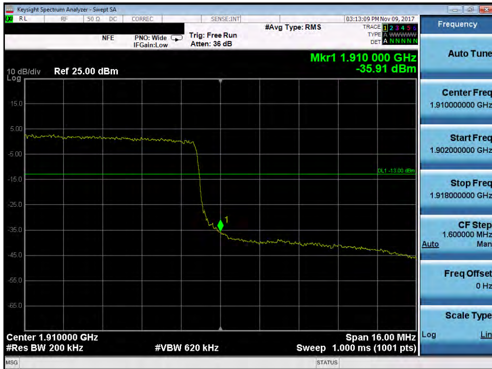
Plot 7-183. Upper Band Edge Plot (Band 2 - 20.0MHz QPSK - Full RB Configuration)
