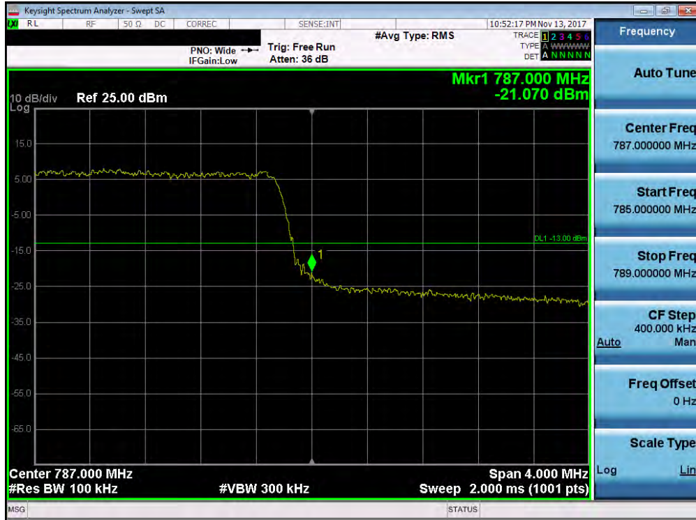
Plot 7-111. Upper Band Edge Plot (Band 13 - 5.0MHz QPSK - Full RB Configuration)
