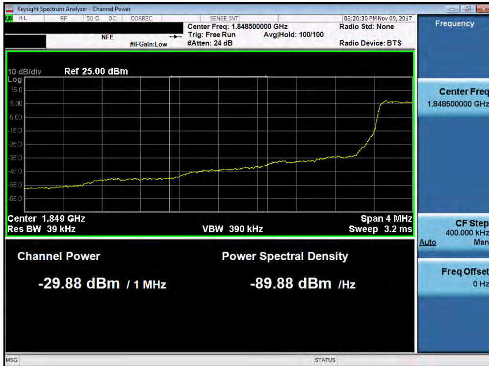
Plot 7-162. . Lower Extended Band Edge Plot (Band 2 - 1.4MHz QPSK - Full RB Configuration)
