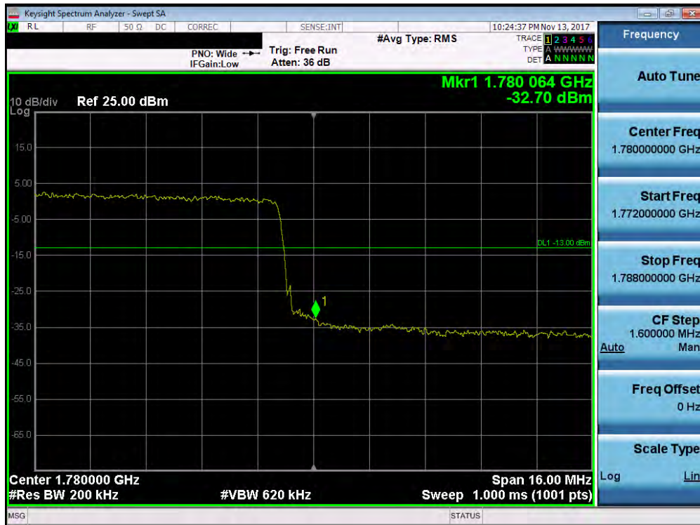
Plot 7-157. Upper Band Edge Plot (Band 66 - 20.0MHz QPSK - Full RB Configuration)
