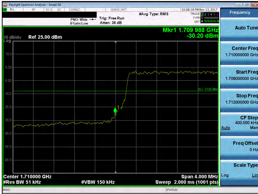
Plot 7-137. Lower Band Edge Plot (Band 66/4 - 5.0MHz QPSK - Full RB Configuration)
