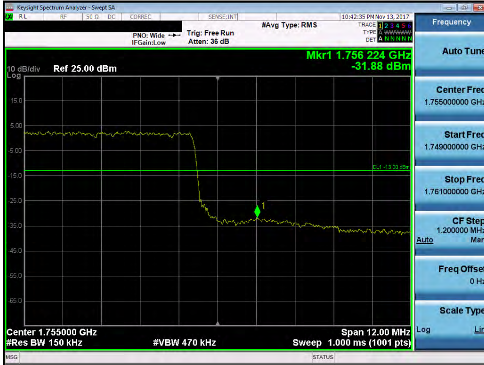
Plot 7-153. Upper Band Edge Plot (Band 4 - 15.0MHz QPSK - Full RB Configuration)
