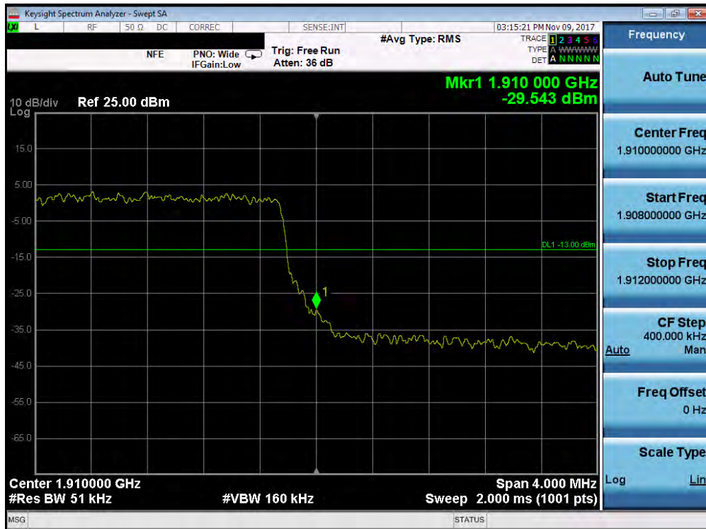
Plot 7-171. Upper Band Edge Plot (Band 2 - 5.0MHz QPSK - Full RB Configuration)
