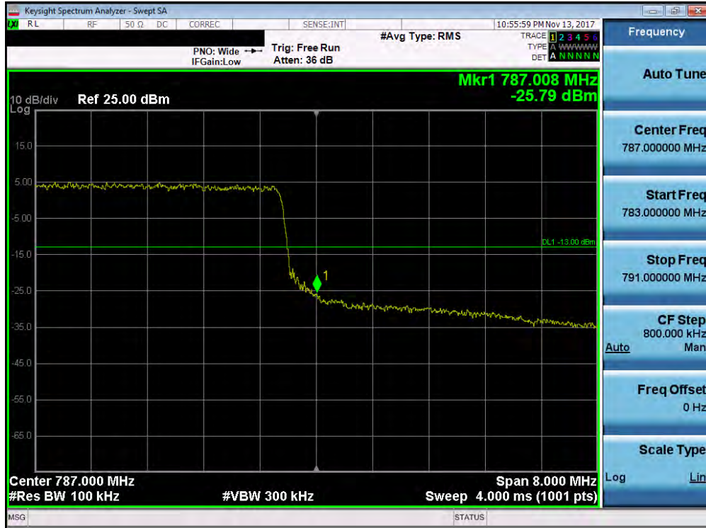
Plot 7-115. Upper Band Edge Plot (Band 13 - 10.0MHz QPSK - Full RB Configuration)
