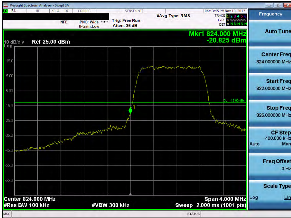
Plot 7-117. Lower Band Edge Plot (Band 5 - 1.4MHz QPSK - Full RB Configuration)
