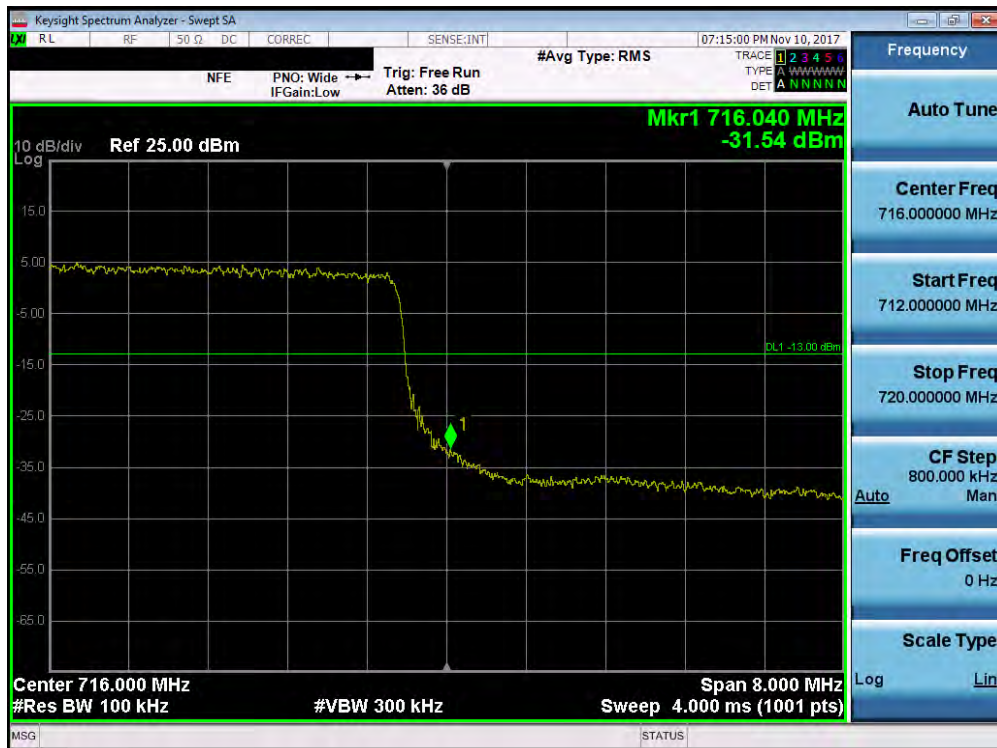
Plot 7-108. Upper Band Edge Plot (Band 12/17 - 10.0MHz QPSK - Full RB Configuration)
