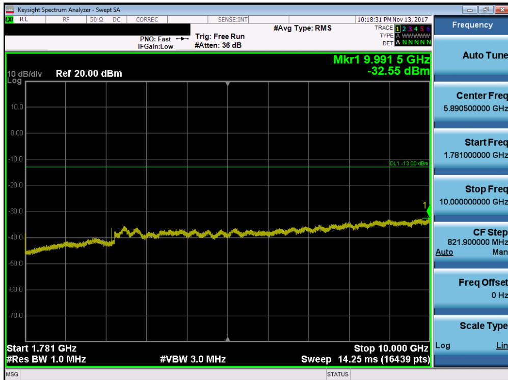
Plot 7-81. Conducted Spurious Plot (Band 66/4 - 15.0MHz QPSK - RB Size 1, RB Offset 0 - High Channel)
