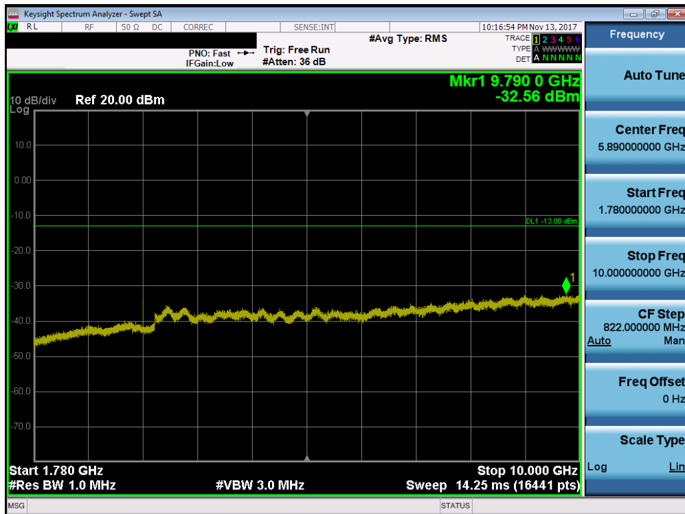
Plot 7-75. Conducted Spurious Plot (Band 66/4 - 15.0MHz QPSK - RB Size 1, RB Offset 0 - Low Channel)
