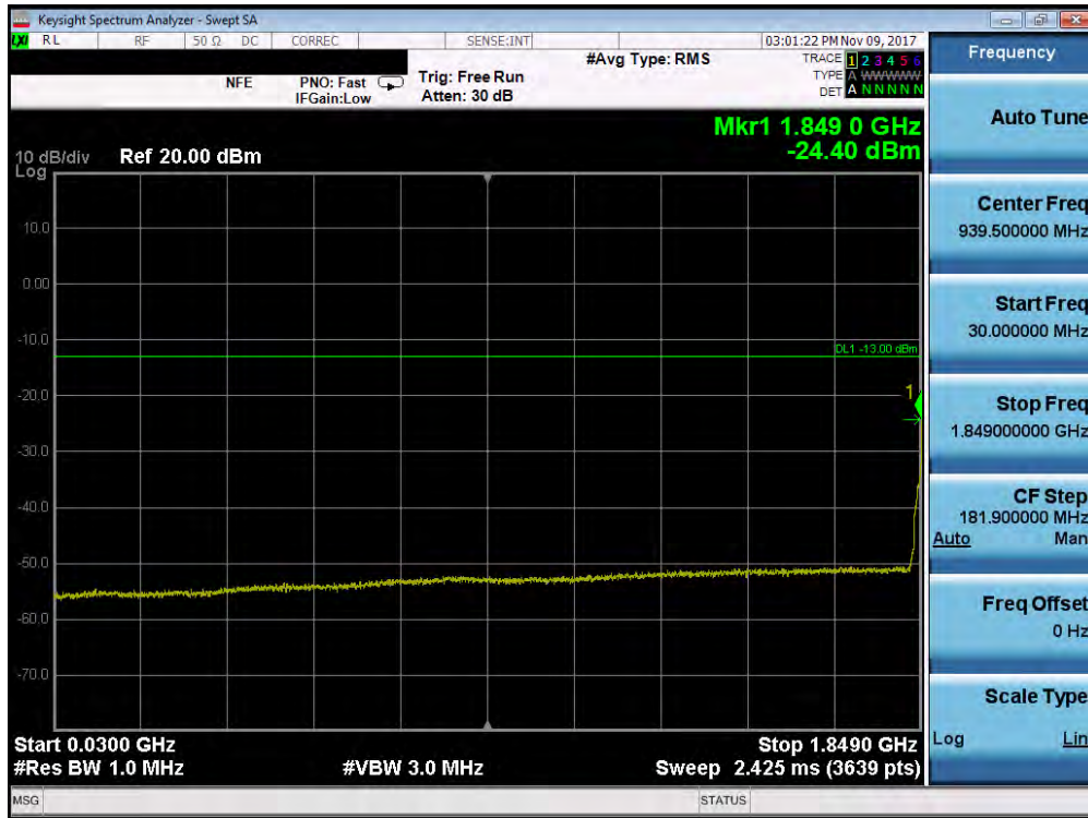
Plot 7-83. Conducted Spurious Plot (Band 2 - 10.0MHz QPSK - RB Size 1, RB Offset 0 - Low Channel)
