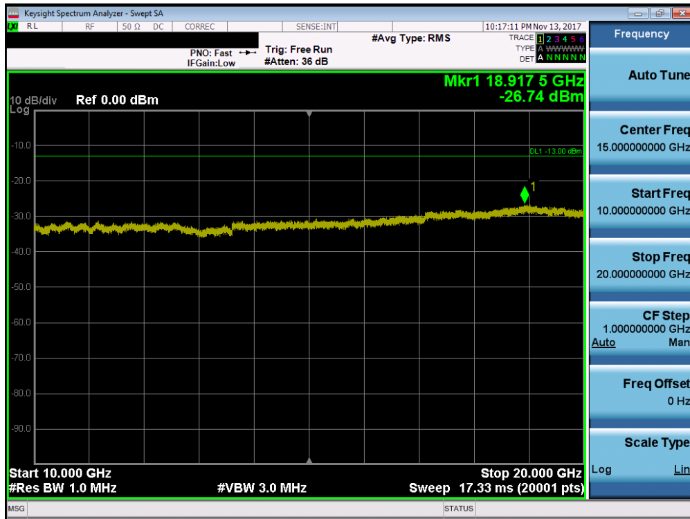
Plot 7-76. Conducted Spurious Plot (Band 66/4 - 15.0MHz QPSK - RB Size 1, RB Offset 0 - Low Channel)
