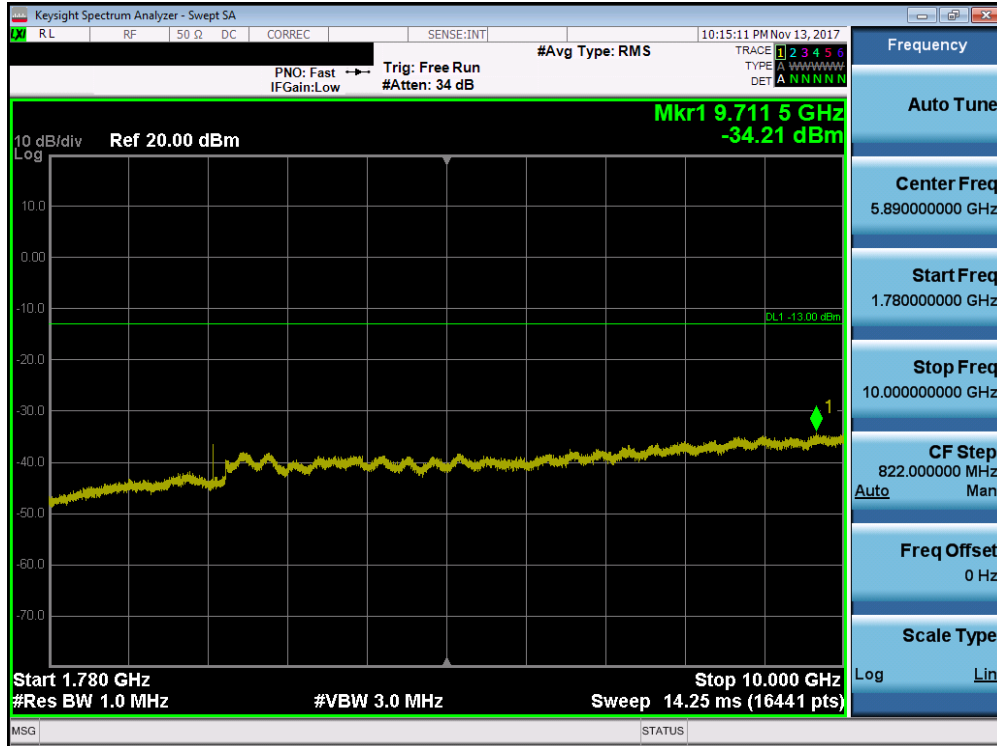
Plot 7-78. Conducted Spurious Plot (Band 66/4 - 15.0MHz QPSK - RB Size 1, RB Offset 0 - Mid Channel)
