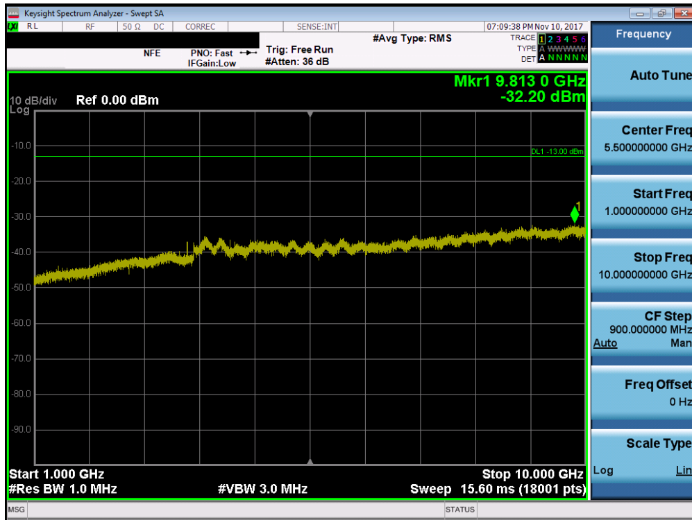
Plot 7-55. Conducted Spurious Plot (Band 12/17 - 5.0MHz QPSK - RB Size 1, RB Offset 0 - Low Channel)
