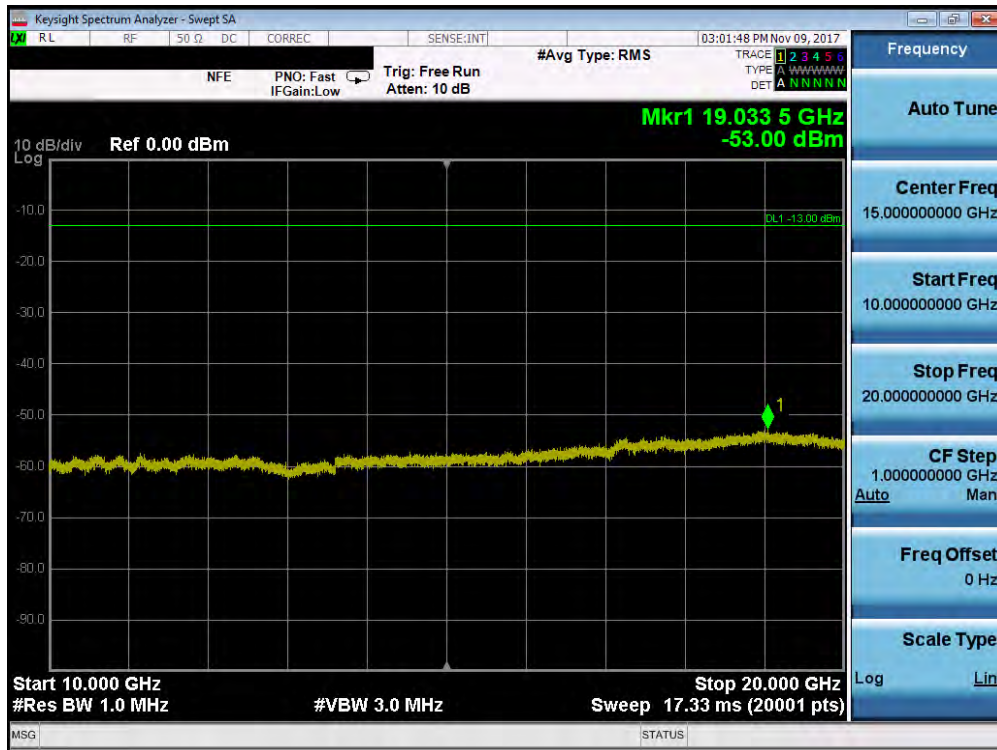
Plot 7-85. Conducted Spurious Plot (Band 2 - 10.0MHz QPSK - RB Size 1, RB Offset 0 - Low Channel)
