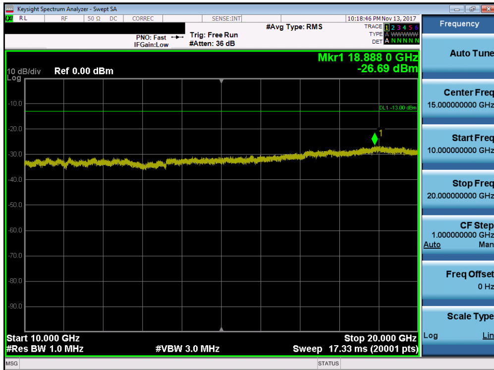
Plot 7-82. Conducted Spurious Plot (Band 66/4 - 15.0MHz QPSK - RB Size 1, RB Offset 0 - High Channel)
