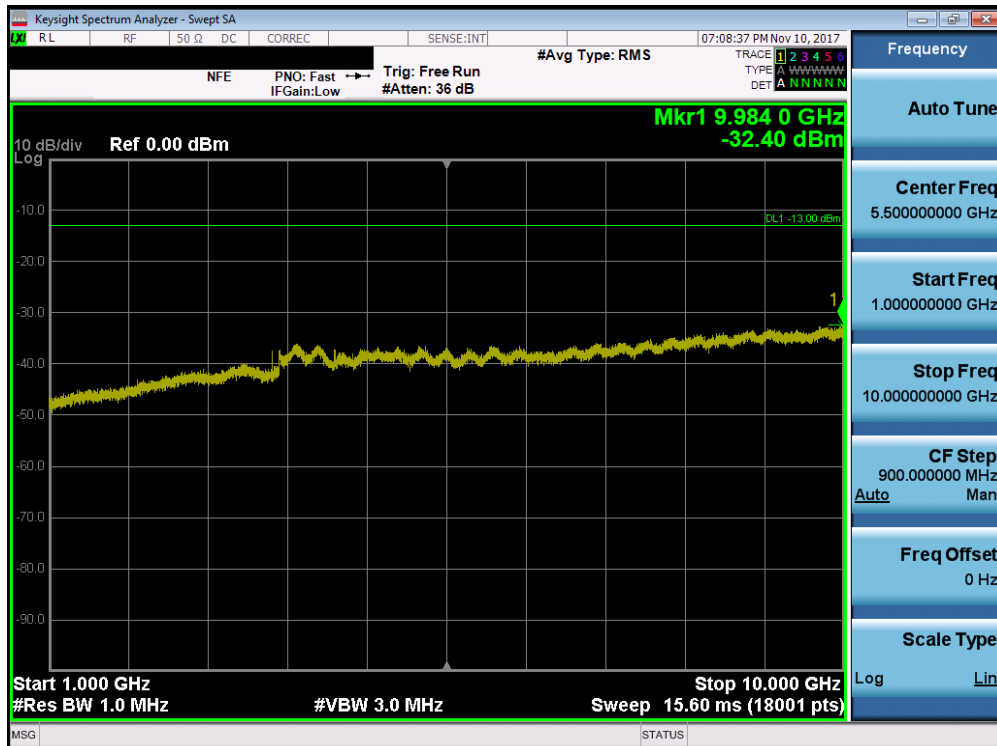
Plot 7-58. Conducted Spurious Plot (Band 12/17 - 5.0MHz QPSK - RB Size 1, RB Offset 0 - Mid Channel)
