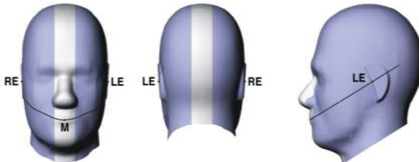
Figure 6-2 Front, back and side views of SAM Twin Phantom
