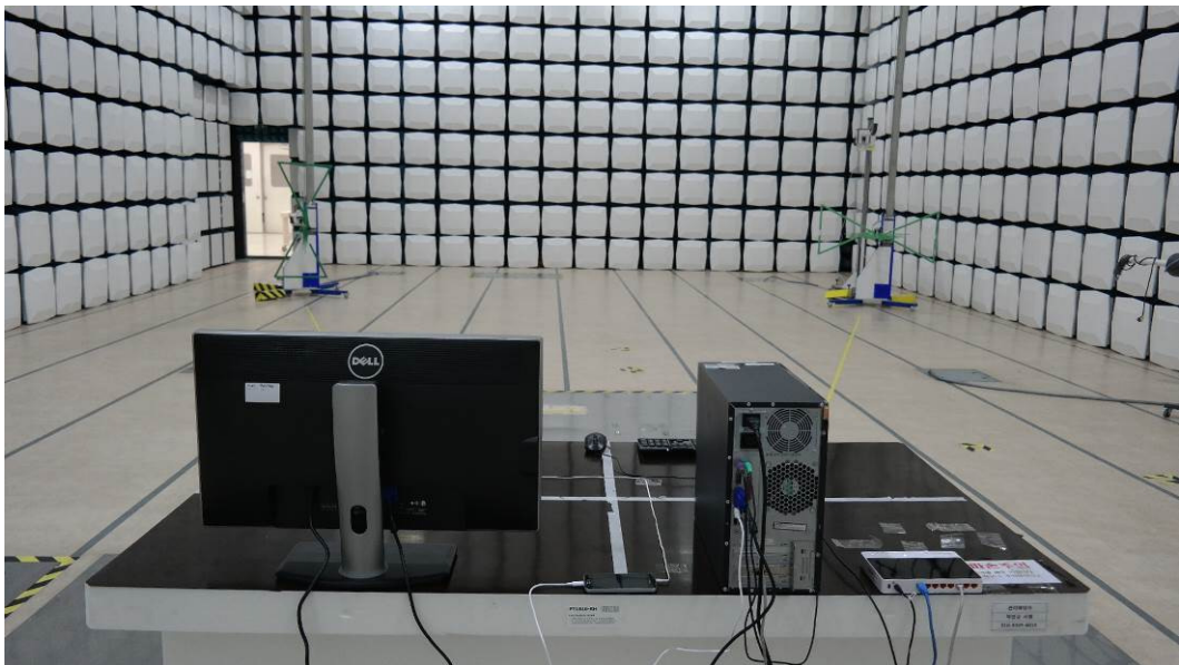
[ Radiated Disturbance for Below 1 GHz – Rear ]
