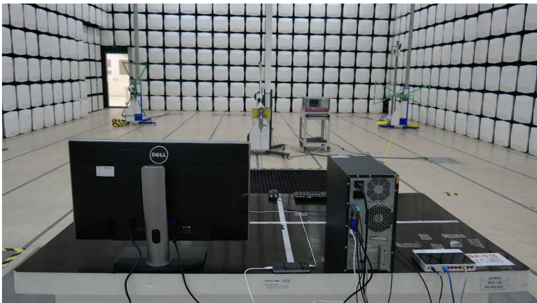
[ Radiated Disturbance for Above 1 GHz – Rear ]
