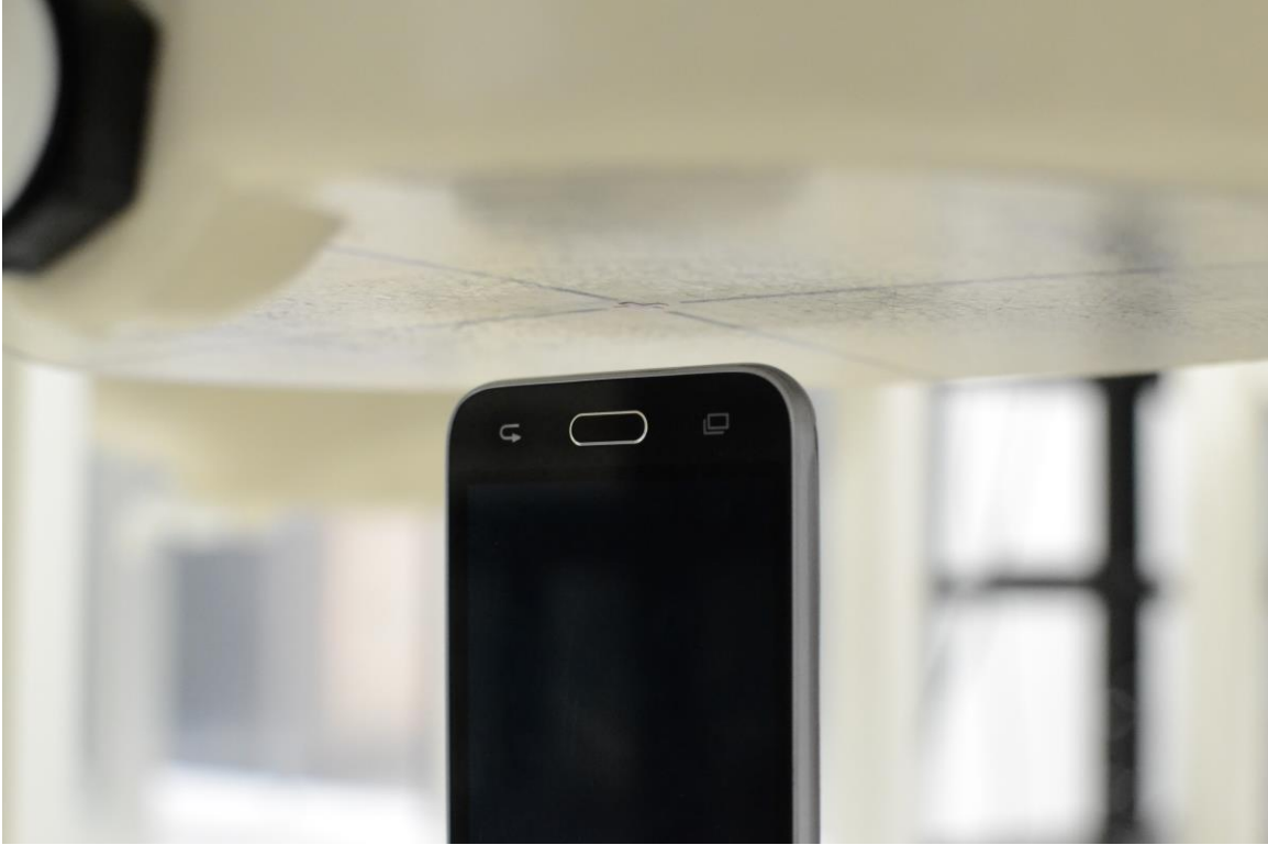
SAR Test Setup Photo 9 – Bottom Edge (10 mm)
