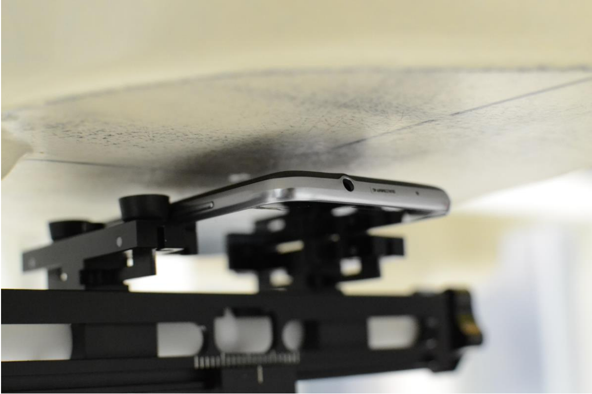
SAR Test Setup Photo 5 – Back Side (10 mm)
