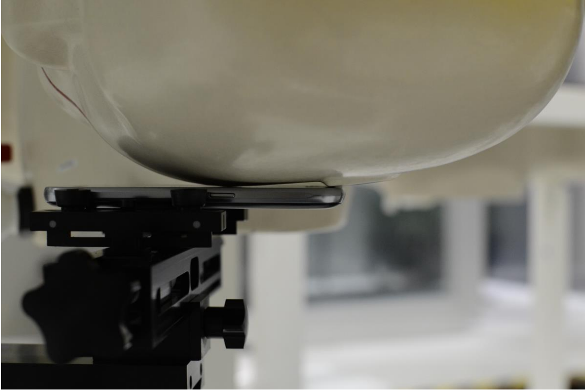
SAR Test Setup Photo 3 – Left Cheek
