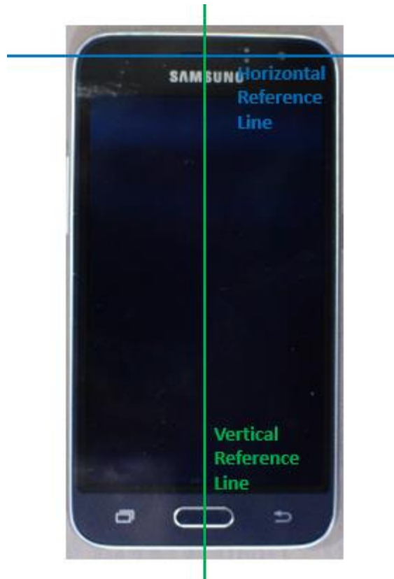
SAR Test Setup Photo 12 – Horizontal and Vertical Reference Lines
