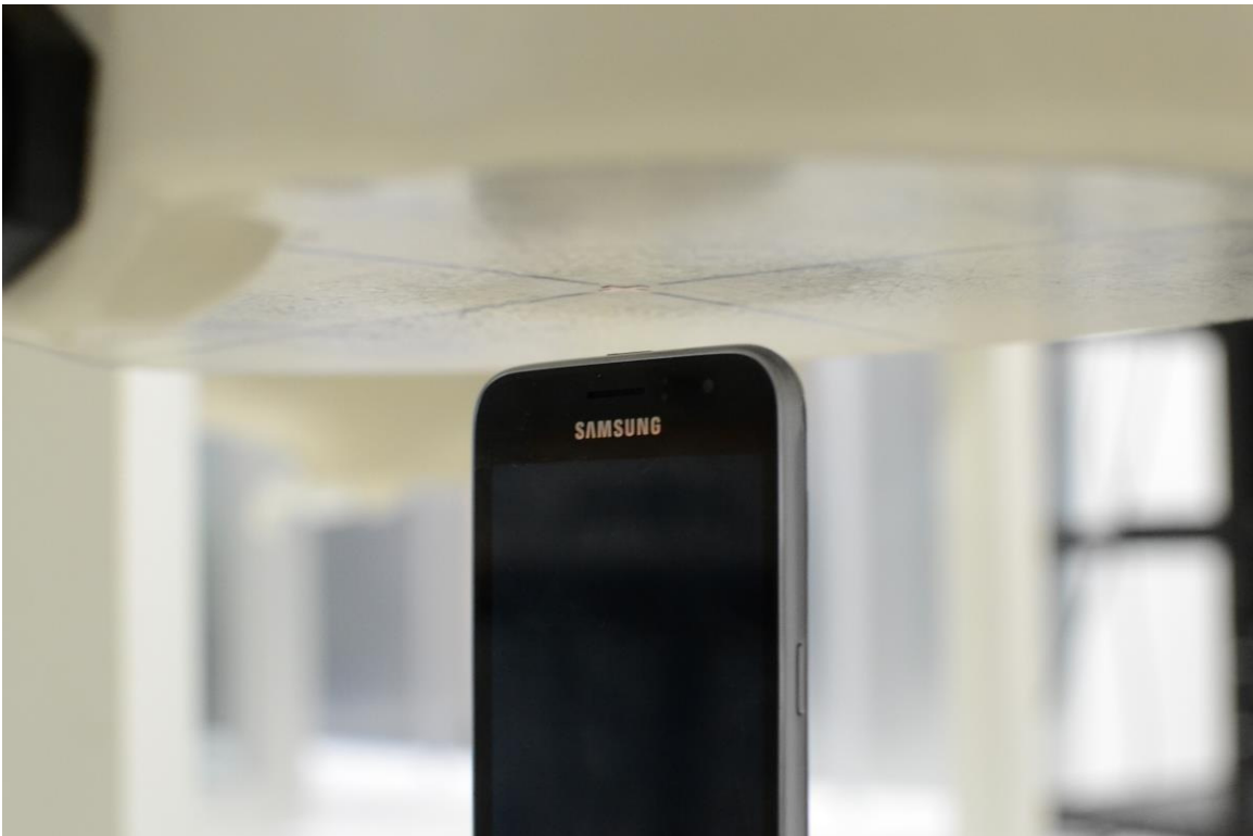
SAR Test Setup Photo 8 – Top Edge (10 mm)
