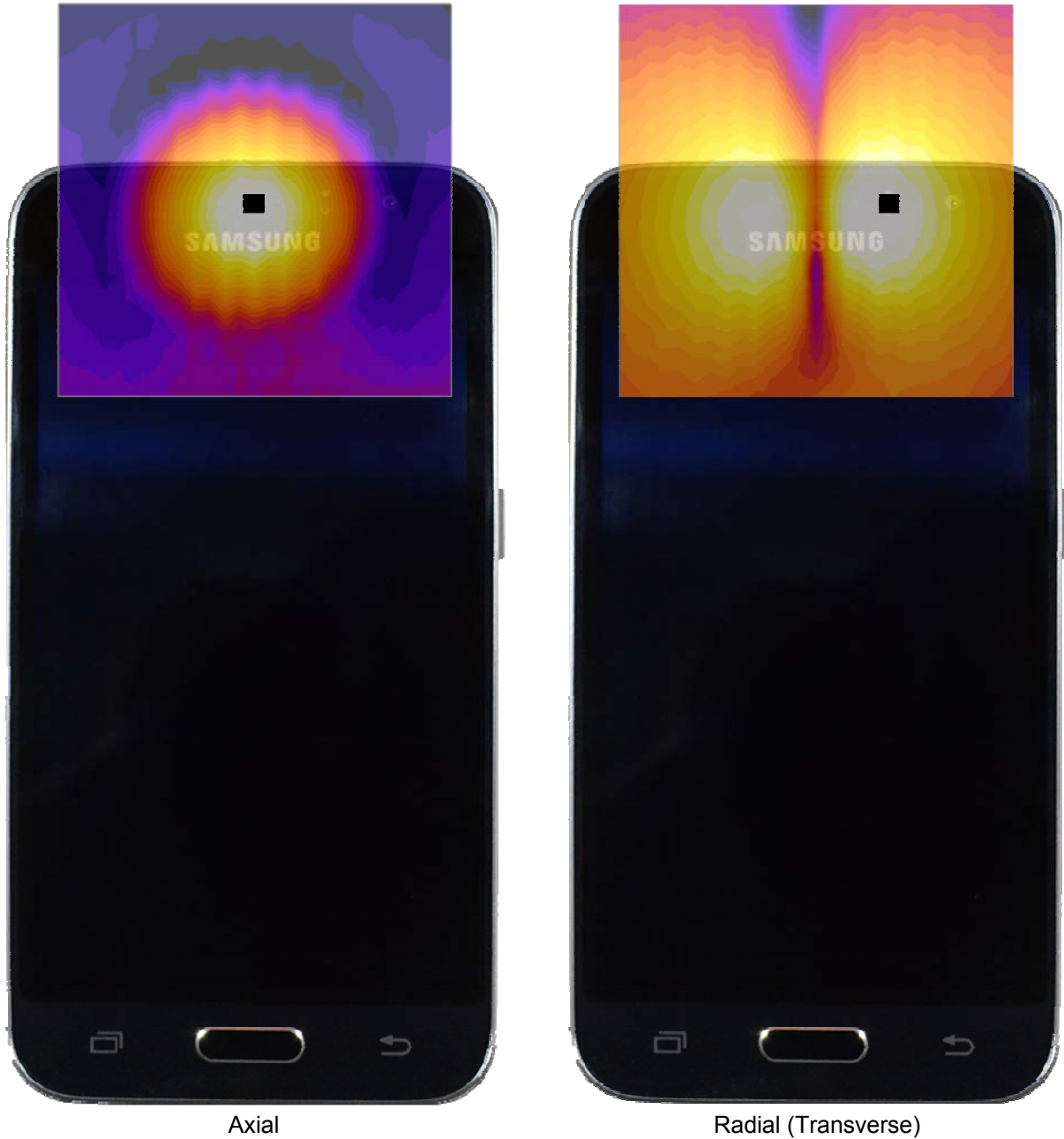
Figure 14-3 T-Coil Scan Overlay Magnetic Field Distributions
