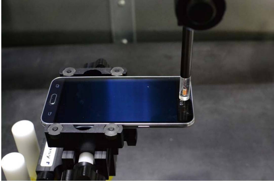
Figure 14-1 Test Setup for Wireless Device
