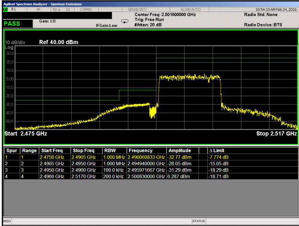
Plot 7-94. Lower ACP Plot (Band 41 – 10.0MHz QPSK – RB Size 50)
