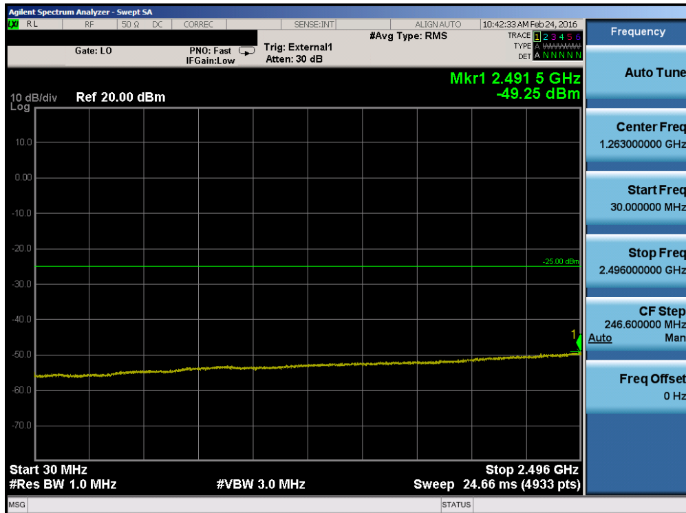
Plot 7-52. Conducted Spurious Plot (Band 41 – 5.0MHz QPSK – RB Size 1, RB Offset 0 – Mid Channel)
