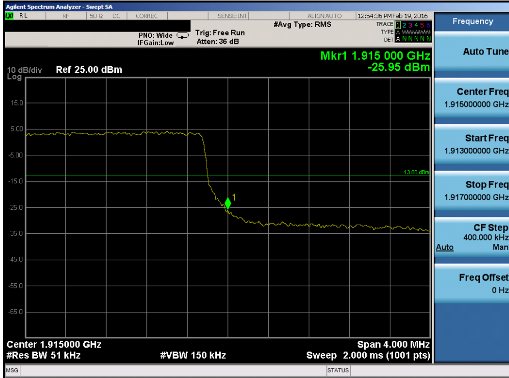
Plot 7-78. Upper Band Edge Plot (Band 25 – 5.0MHz QPSK – RB Size 25)
