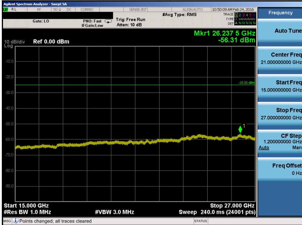
Plot 7-57. Conducted Spurious Plot (Band 41 – 5.0MHz QPSK – RB Size 1, RB Offset 0 – High Channel)
