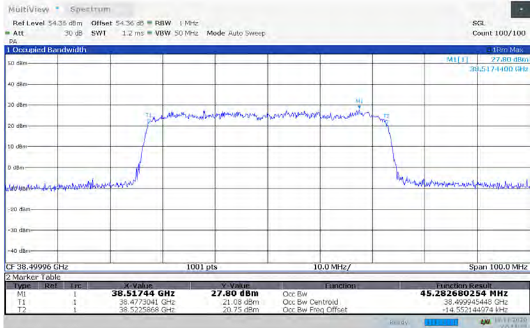
Plot 7-27. Occupied Bandwidth Plot (50MHz-1CC – 16QAM – Mid Channel)
