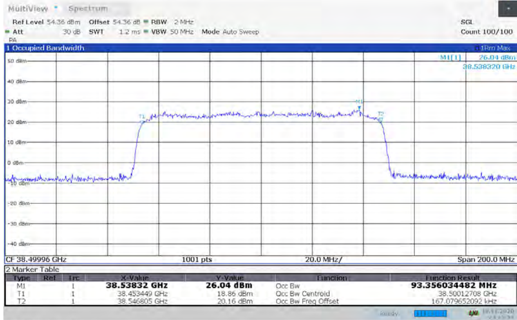
Plot 7-18. Occupied Bandwidth Plot (100MHz-1CC – QPSK – Mid Channel)
