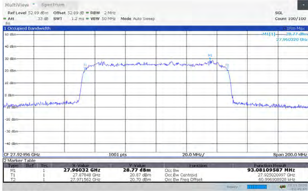
Plot 7-2. Occupied Bandwidth Plot (100MHz-1CC – QPSK – Mid Channel)
