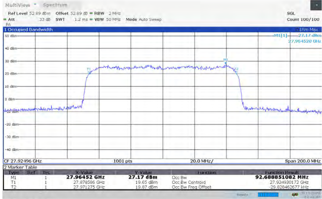
Plot 7-4. Occupied Bandwidth Plot (100MHz-1CC – 64QAM – Mid Channel)
