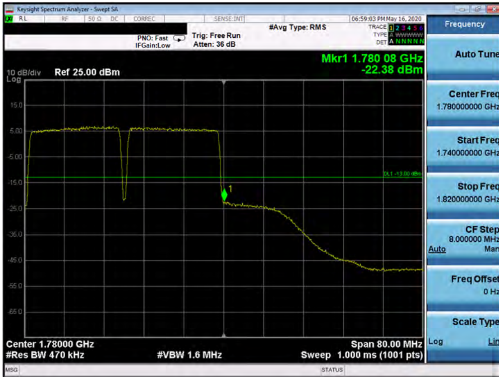
Plot 7-388. Upper Band Edge Plot (Band 66 QPSK – PCC:20 MHz SCC:20 MHz – Full RB)
