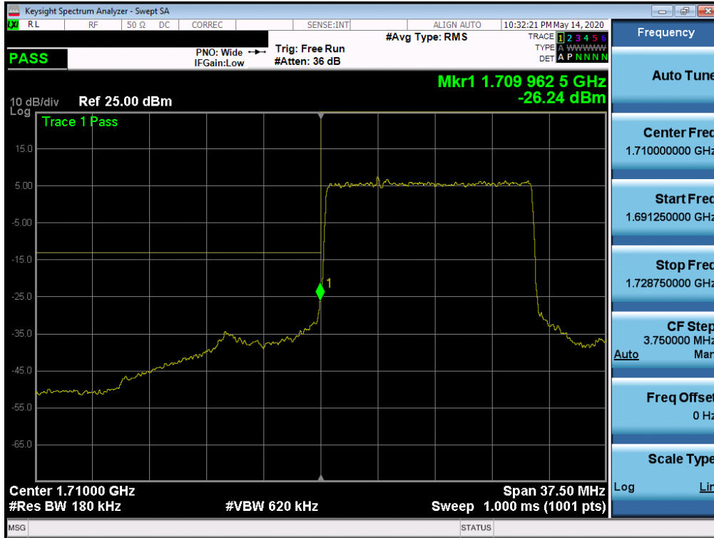
Plot 7-264. Lower Band Edge Plot (NR Band n66 – 15.0MHz - Full RB)
