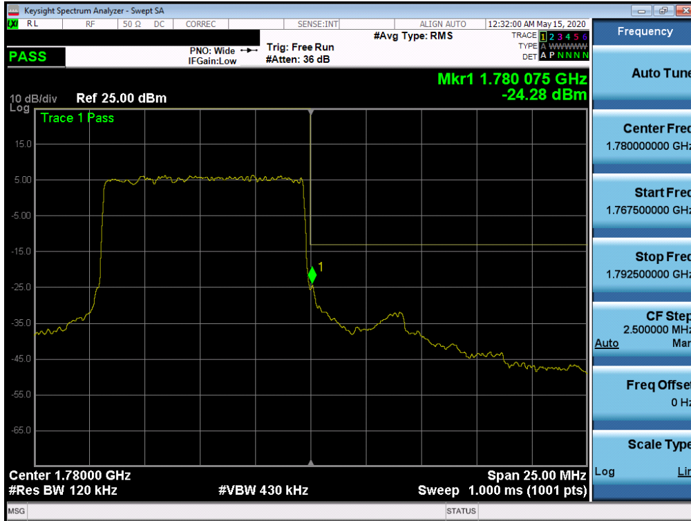
Plot 7-262. Upper Band Edge Plot (NR Band n66 – 10.0MHz - Full RB)
