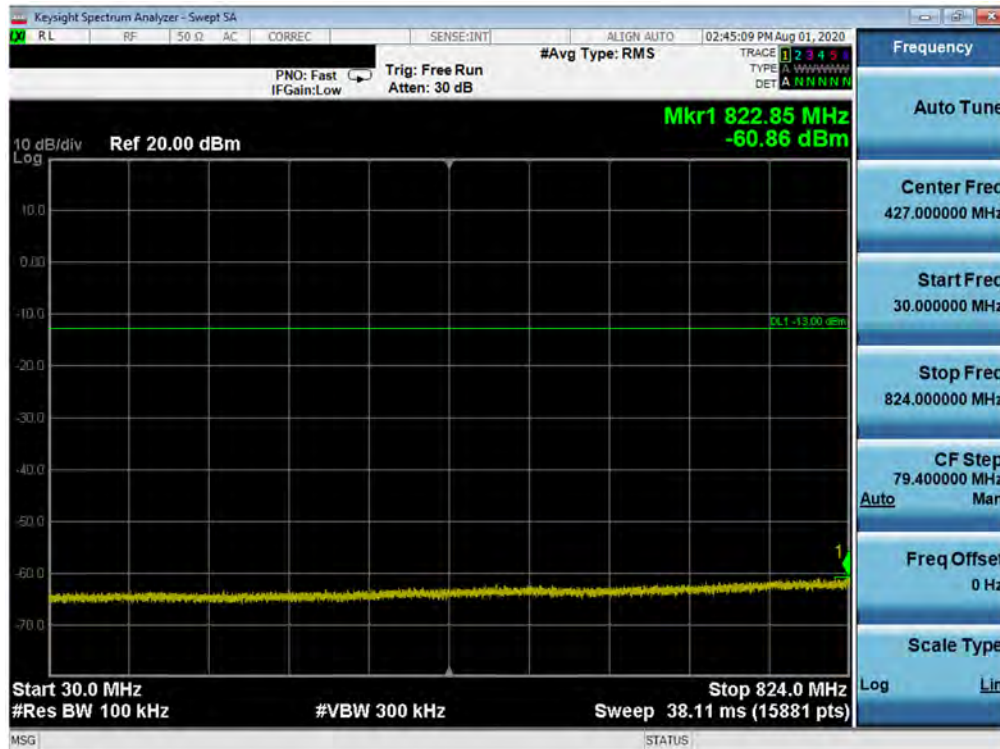
Plot 7-121. Conducted Spurious Plot (Band 5 - 10.0MHz QPSK - RB Size 1, RB Offset 0 - Mid Channel)
