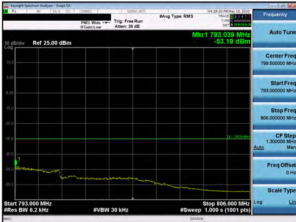
Plot 7-179. Upper Emission Mask Plot (Band 13 - 10.0MHz QPSK - Full RB Configuration)
