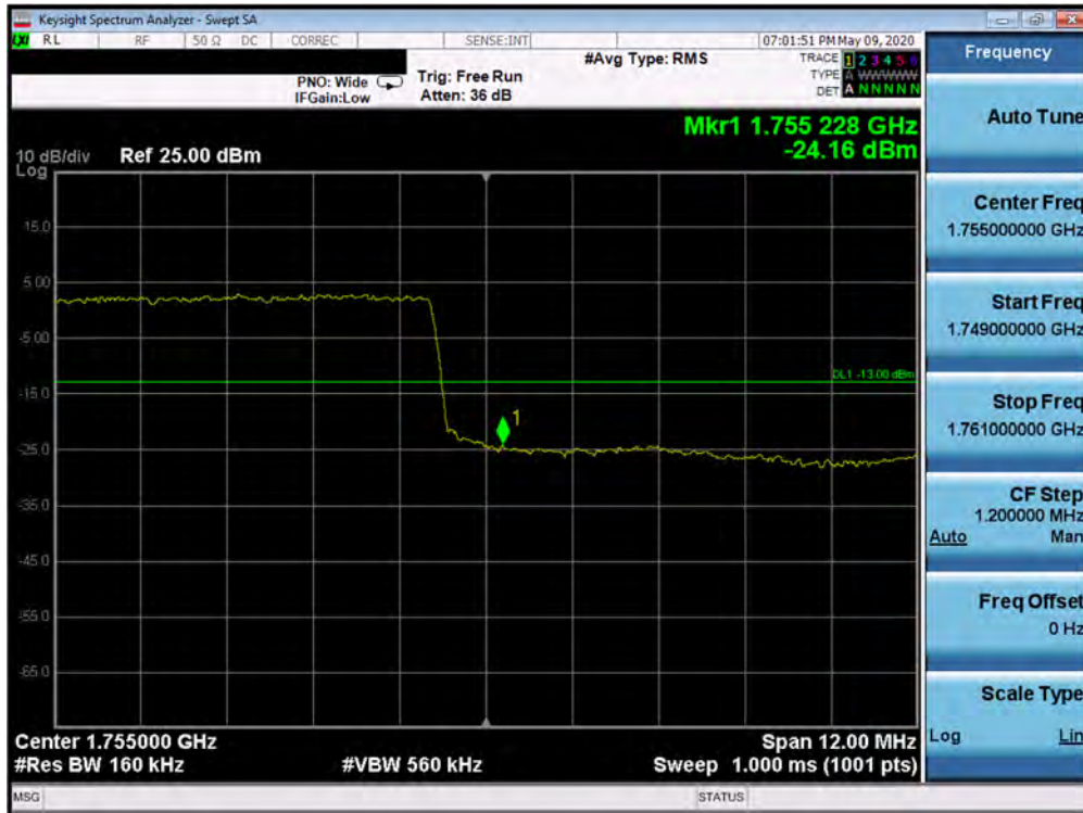
Plot 7-214. Upper Band Edge Plot (Band 4 - 15.0MHz QPSK - Full RB Configuration)
