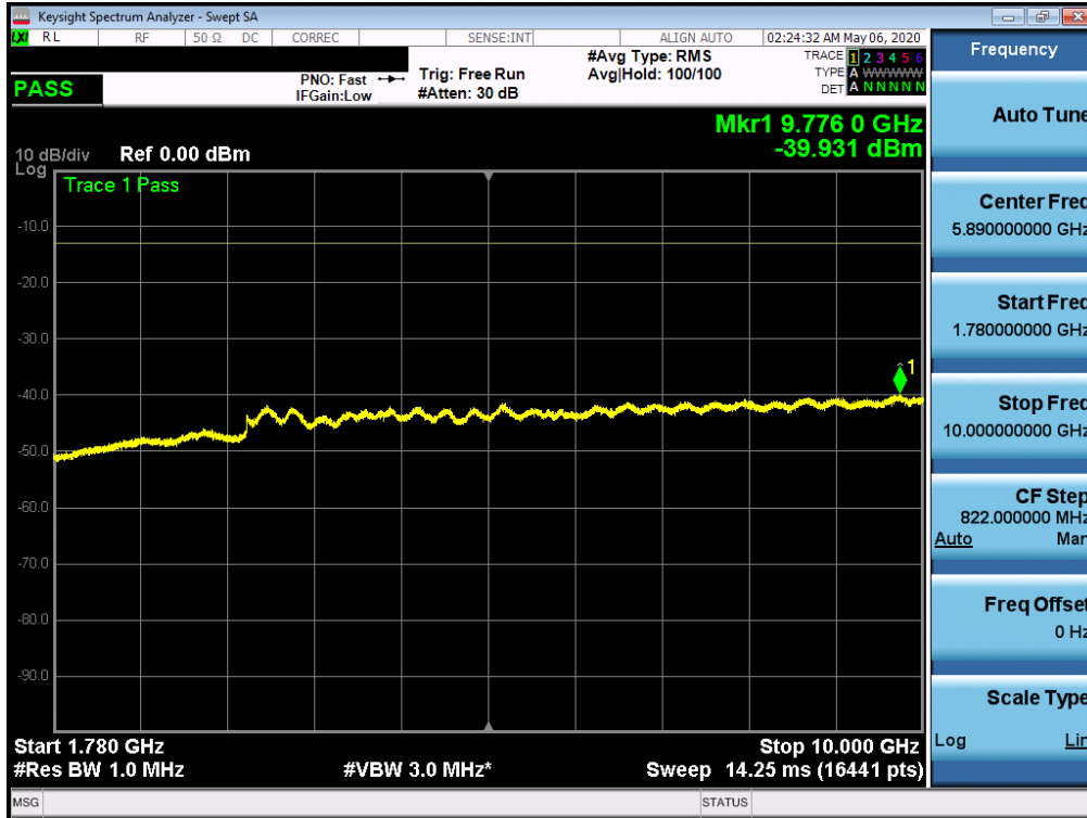
Plot 7-158. Conducted Spurious Plot (NR Band n66 - 20.0MHz - RB Size 1, RB Offset 0 - Mid Channel)
