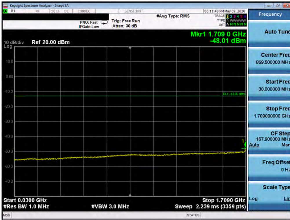
Plot 7-127. Conducted Spurious Plot (Band 66/4 - 20.0MHz QPSK - RB Size 1, RB Offset 0 - Low Channel)
