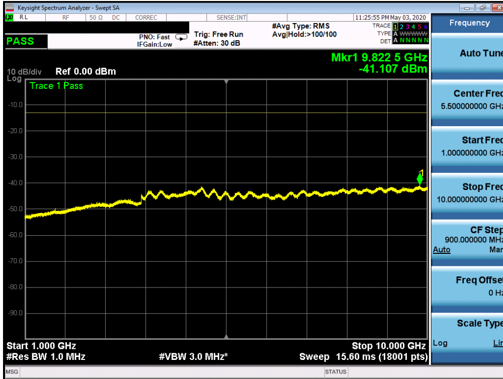
Plot 7-153. Conducted Spurious Plot (NR Band n5 - 20.0MHz - RB Size 1, RB Offset 0 - High Channel)
