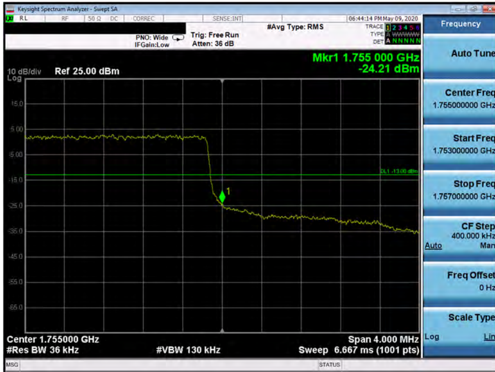
Plot 7-196. Upper Band Edge Plot (Band 4 - 3.0MHz QPSK - Full RB Configuration)
