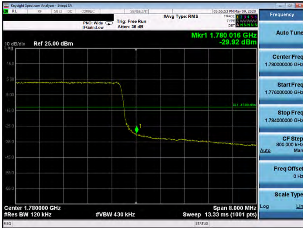
Plot 7-210. Upper Band Edge Plot (Band 66 - 10.0MHz QPSK - Full RB Configuration)
