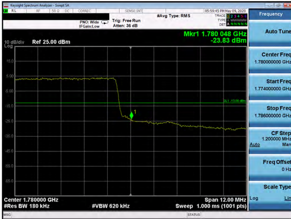
Plot 7-216. Upper Band Edge Plot (Band 66 - 15.0MHz QPSK - Full RB Configuration)
