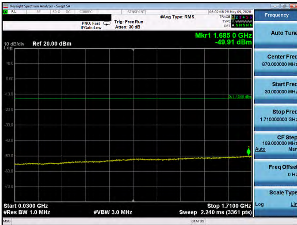
Plot 7-130. Conducted Spurious Plot (Band 66/4 - 20.0MHz QPSK - RB Size 1, RB Offset 0 - Mid Channel)
