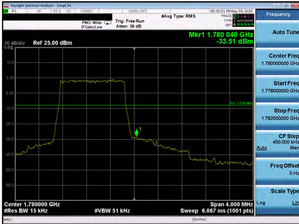
Plot 7-192. Upper Band Edge Plot (Band 66 - 1.4MHz QPSK - Full RB Configuration)
