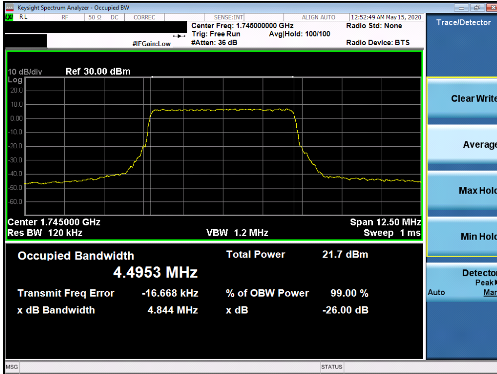
Plot 7-93. Occupied Bandwidth Plot (NR Band n66 - 5MHz CP-OFDM 64-QAM - Full RB Configuration)
