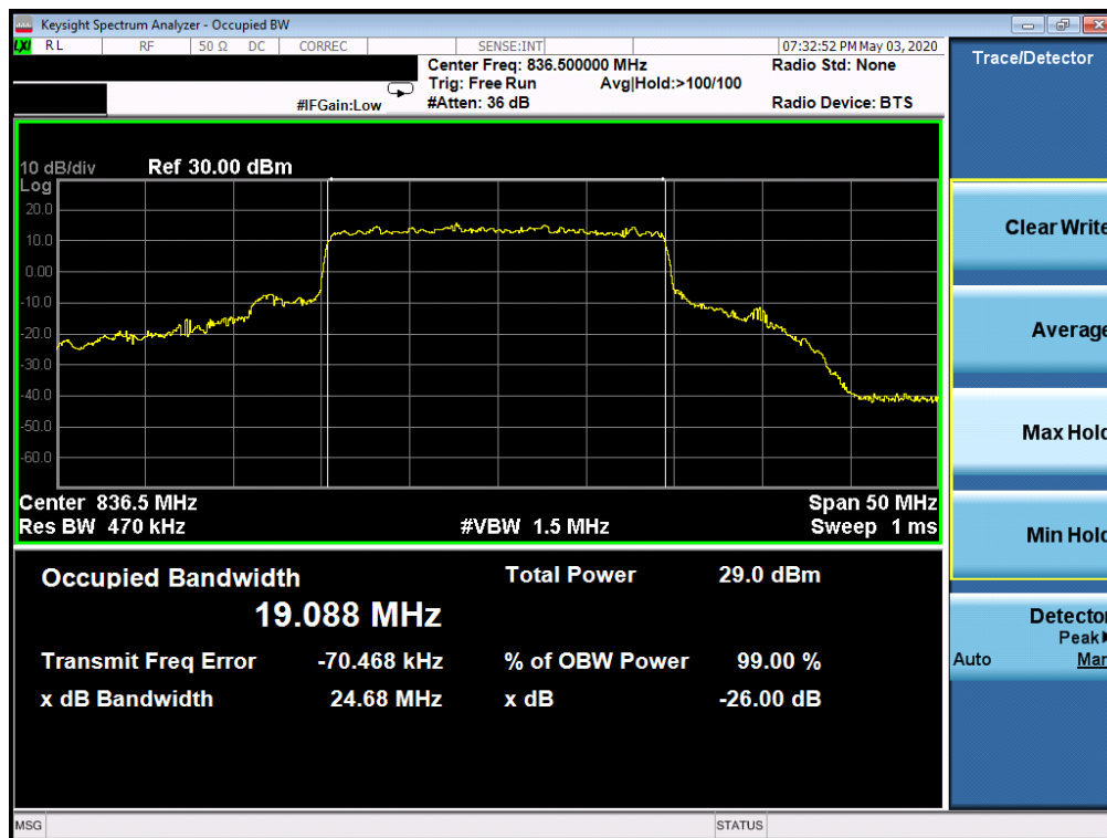
Plot 7-58. Occupied Bandwidth Plot (NR Band n5 - 20MHz CP-OFDM 64-QAM - Full RB Configuration)
