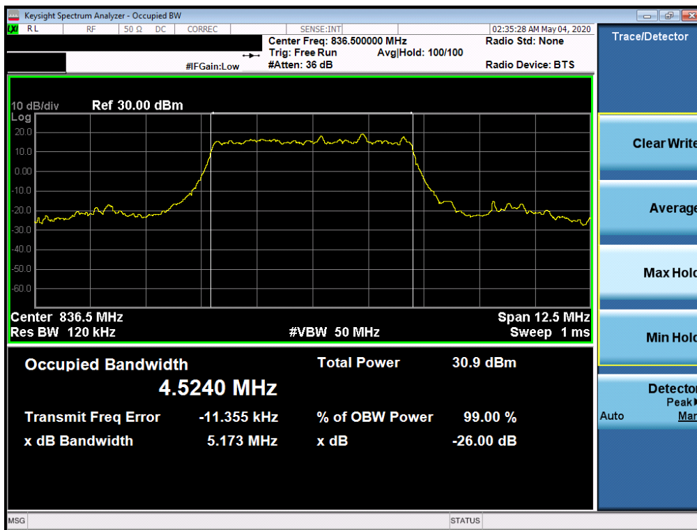
Plot 7-70. Occupied Bandwidth Plot (NR Band n5 - 5MHz DFT-s-OFDM \pi/2 BPSK - Full RB Configuration)
