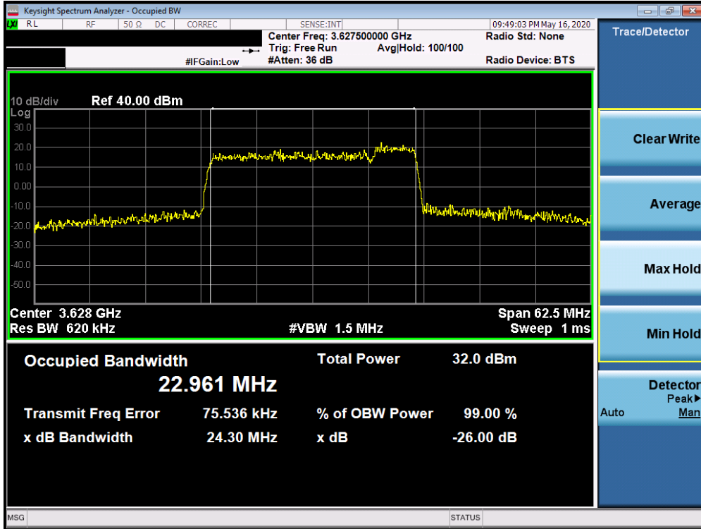
Plot 7-15. Occupied Bandwidth Plot (LTE Band 48 ULCA - 25.0MHz 64-QAM - Full RB Configuration)
