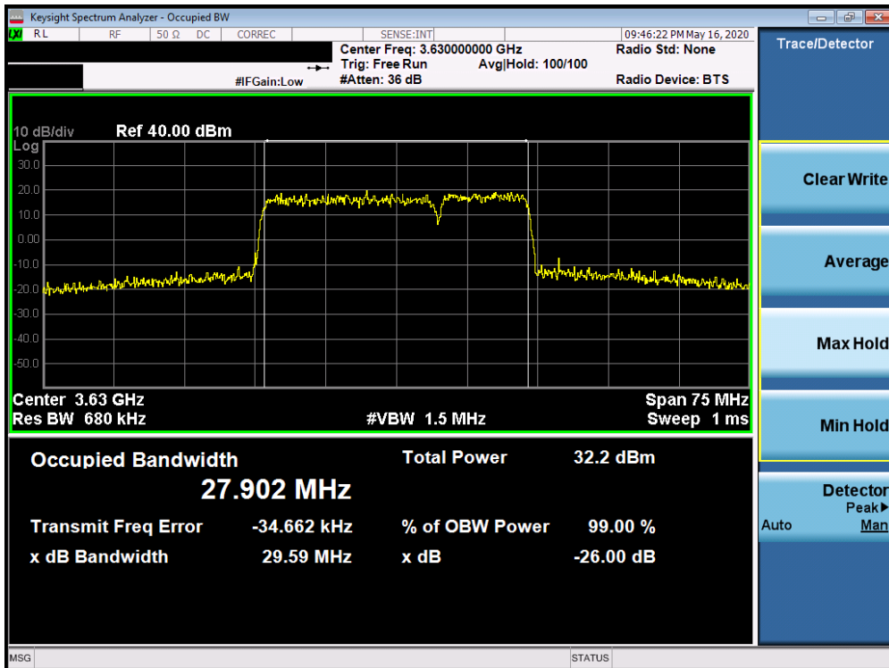
Plot 7-18. Occupied Bandwidth Plot (LTE Band 48 ULCA - 30.0MHz 64-QAM - Full RB Configuration)
