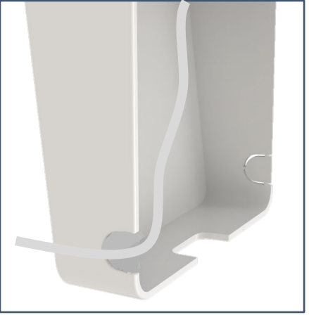
Pass the cable through the hole
