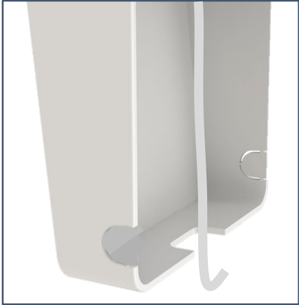
Pass the cable through the hole
