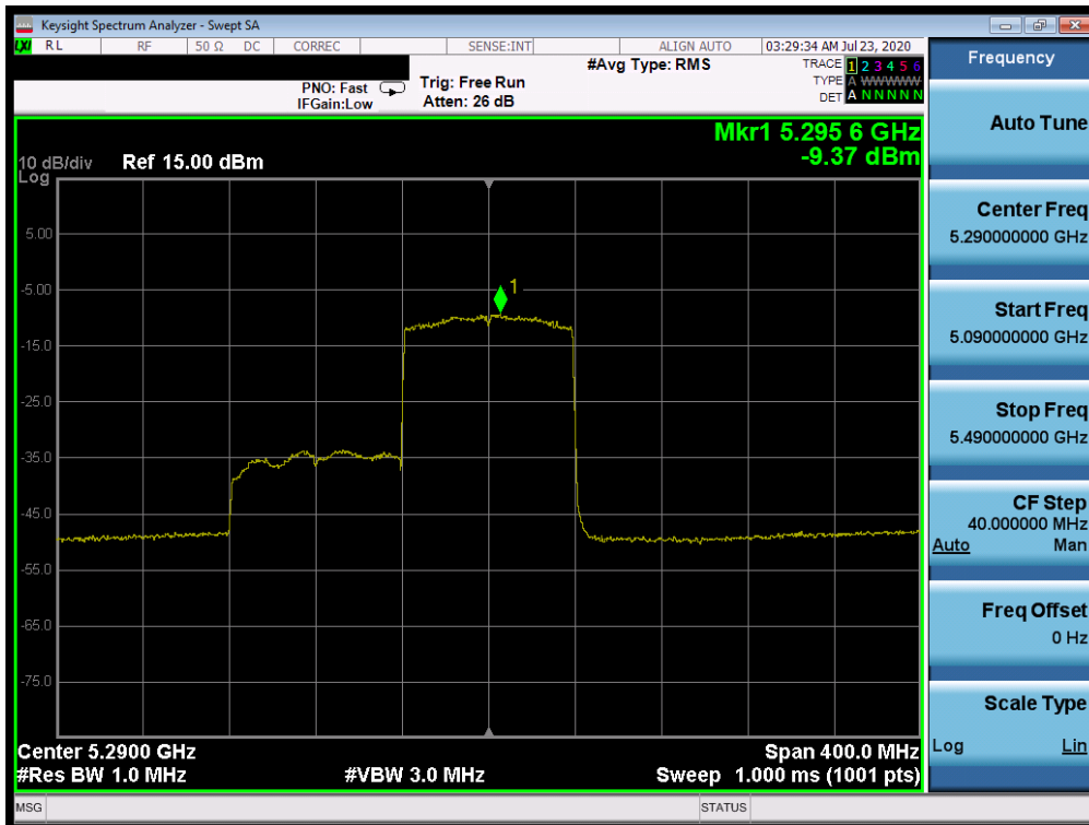
Plot 7-484. Power Spectral Density Plot SISO ANT6 (80MHz BW 802.11ax (UNII Band 2A) – Ch. 58)
