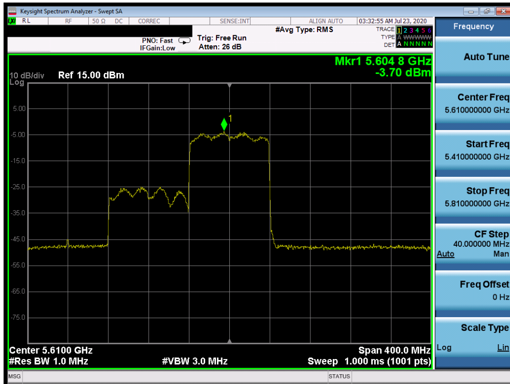
Plot 7-487. Power Spectral Density Plot SISO ANT5 (80MHz BW 802.11ax (UNII Band 2A) – Ch. 122)
