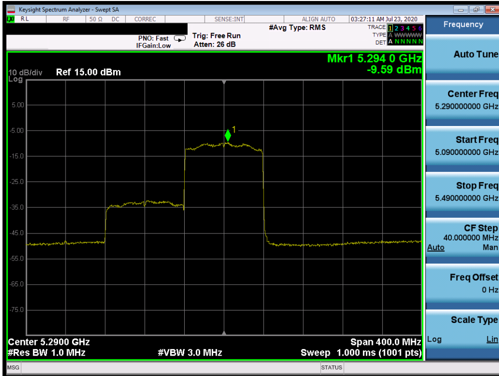
Plot 7-483. Power Spectral Density Plot SISO ANT5 (80MHz BW 802.11ax (UNII Band 2A) – Ch. 58)
