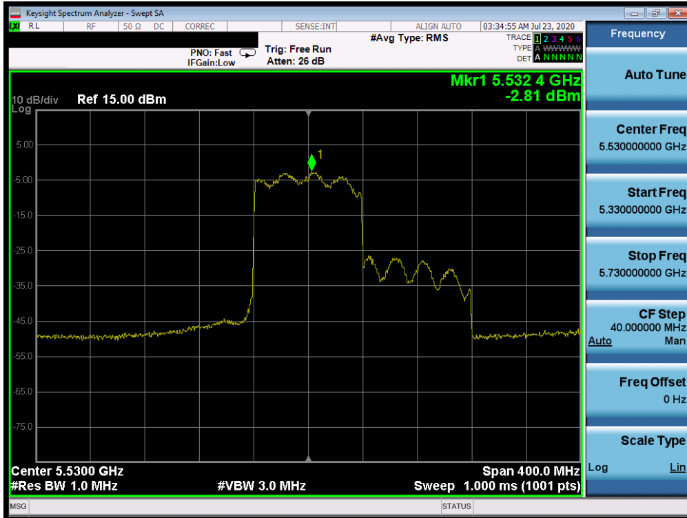
Plot 7-485. Power Spectral Density Plot SISO ANT3 (80MHz BW 802.11ax (UNII Band 1) – Ch. 106)
