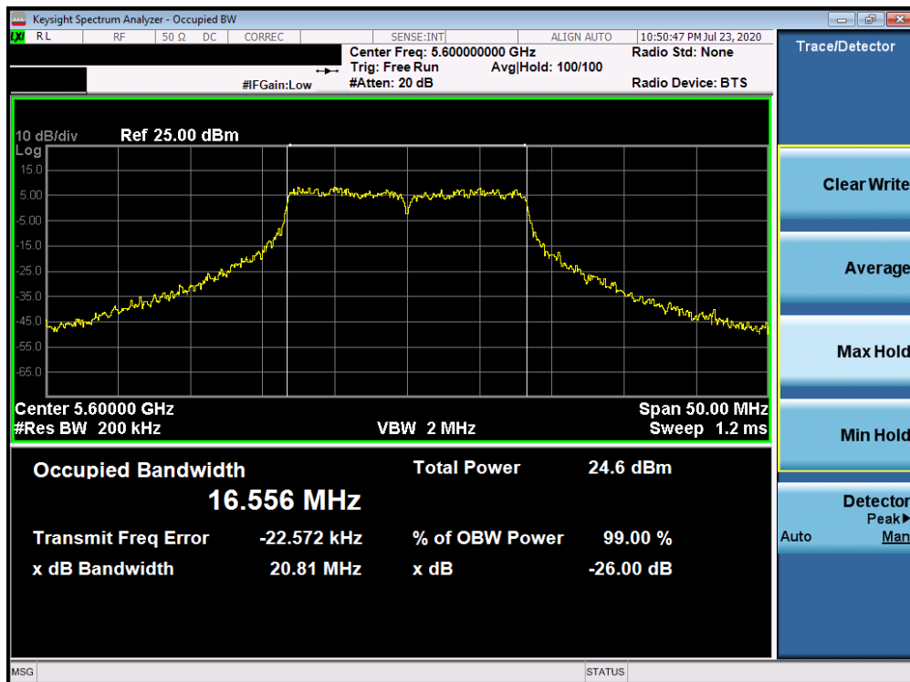
Plot 7-83. 26dB Bandwidth Plot ANT4 (802.11a (UNII Band 2C) – Ch. 120)
