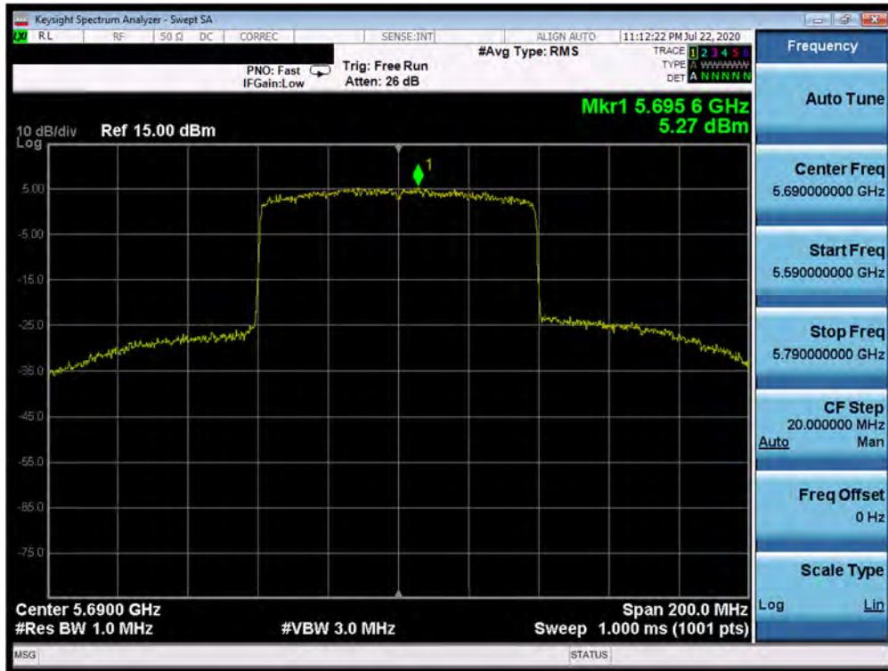
Plot 7-131. Power Spectral Density Plot MIMO ANT3 (80MHz BW 802.11ax – Full Tones (UNII Band 2C) – Ch. 138)
