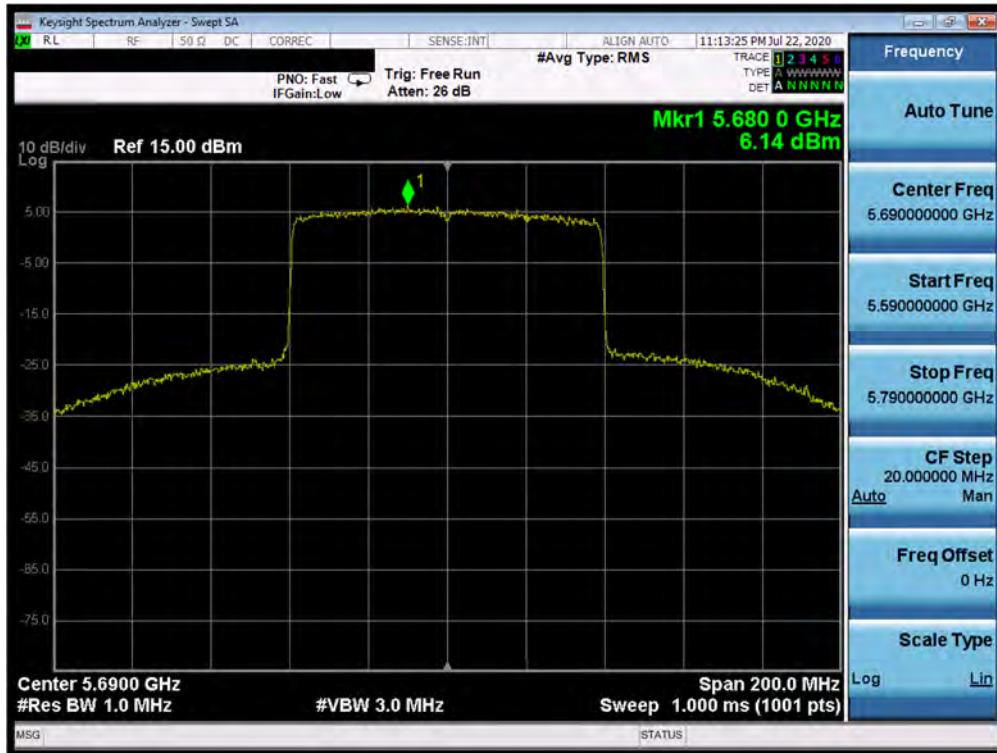
Plot 7-158. Power Spectral Density Plot MIMO ANT4 (80MHz BW 802.11ax – Full Tones (UNII Band 2C) – Ch. 138)
