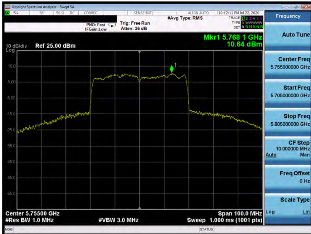
Plot 7-135. Power Spectral Density Plot MIMO ANT3 (40MHz BW 802.11ax – Full Tones (UNII Band 3) – Ch. 151)
