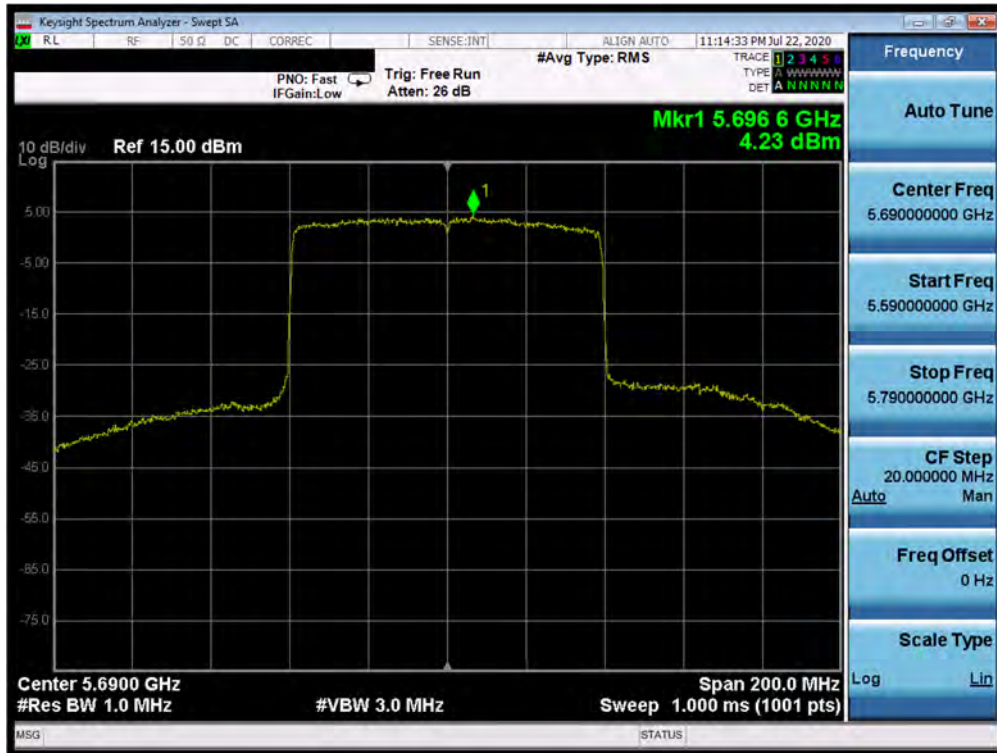
Plot 7-185. Power Spectral Density Plot MIMO ANT5 (80MHz BW 802.11ax – Full Tones (UNII Band 2C) – Ch. 138)
