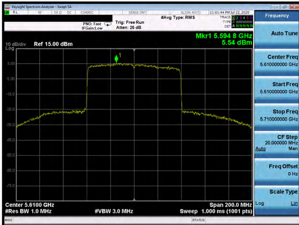
Plot 7-157. Power Spectral Density Plot MIMO ANT4 (80MHz BW 802.11ax – Full Tones (UNII Band 2C) – Ch. 122)
