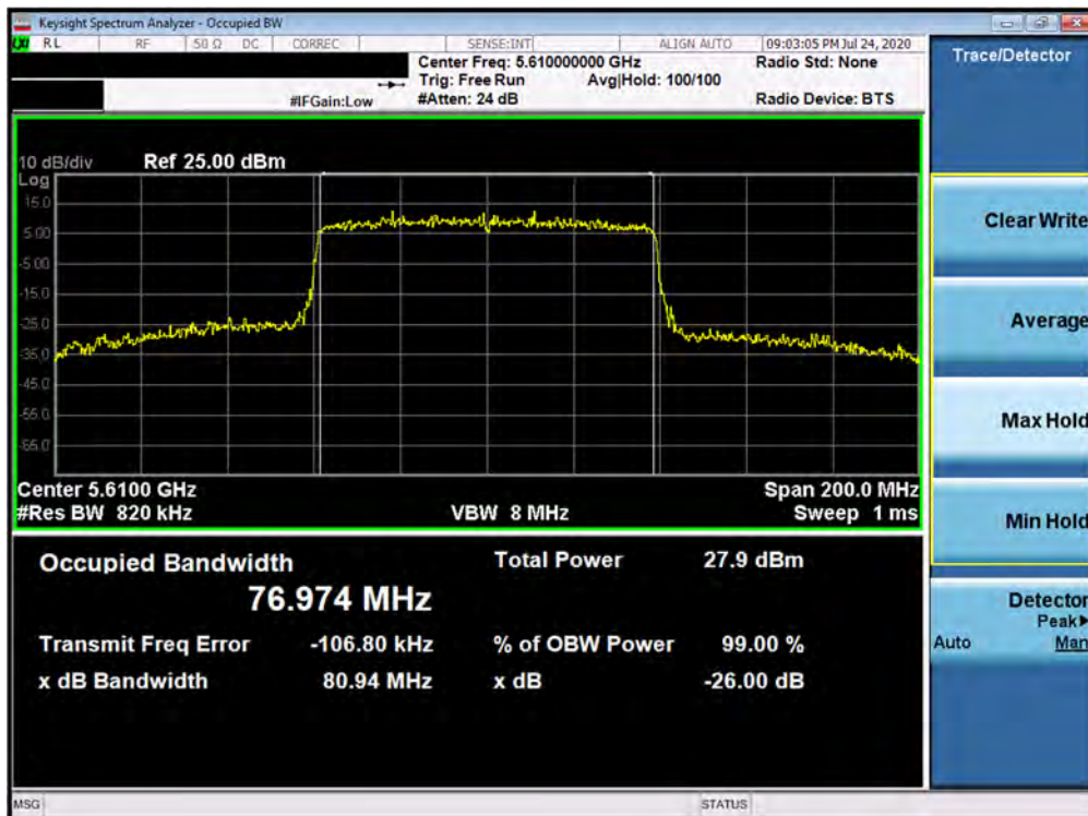
Plot 7-83. 26dB Bandwidth Plot ANT6 (80MHz BW 802.11ax – 996 Tones (UNII Band 2C) – Ch. 122)
