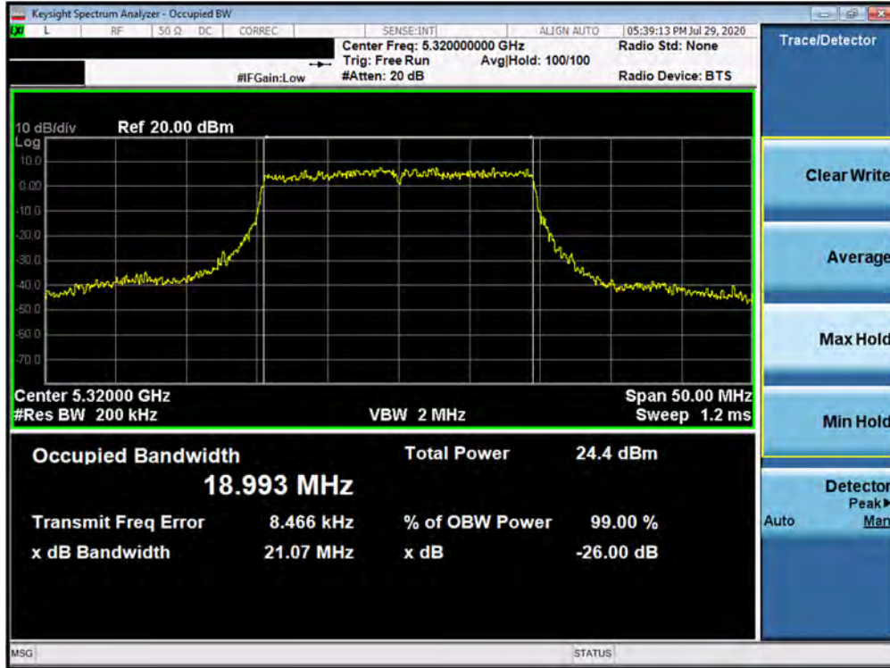
Plot 7-9. 26dB Bandwidth Plot ANT3 (20MHz BW 802.11ax – 242 Tones (UNII Band 2A) – Ch. 64)
