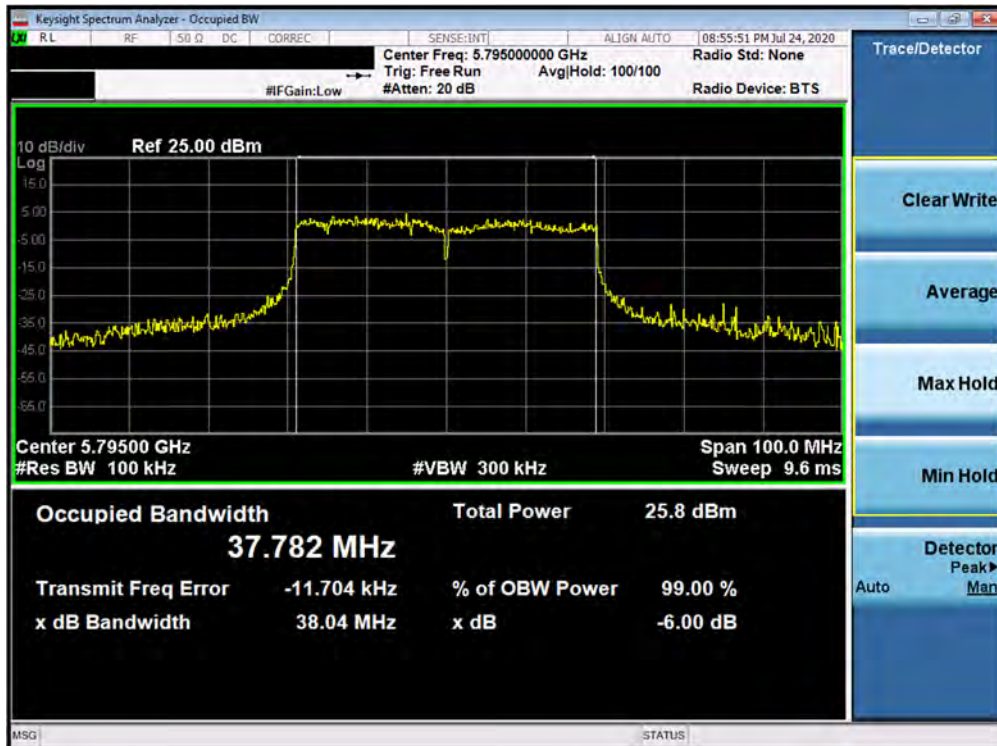
Plot 7-109. 6dB Bandwidth Plot ANT6 (40MHz BW 802.11ax – 484 Tones (UNII Band 3) – Ch. 159)
