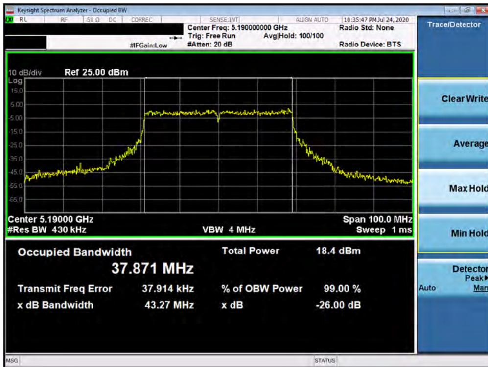
Plot 7-25. 26dB Bandwidth Plot ANT4 (40MHz BW 802.11ax – 484 Tones (UNII Band 1) – Ch. 38)
