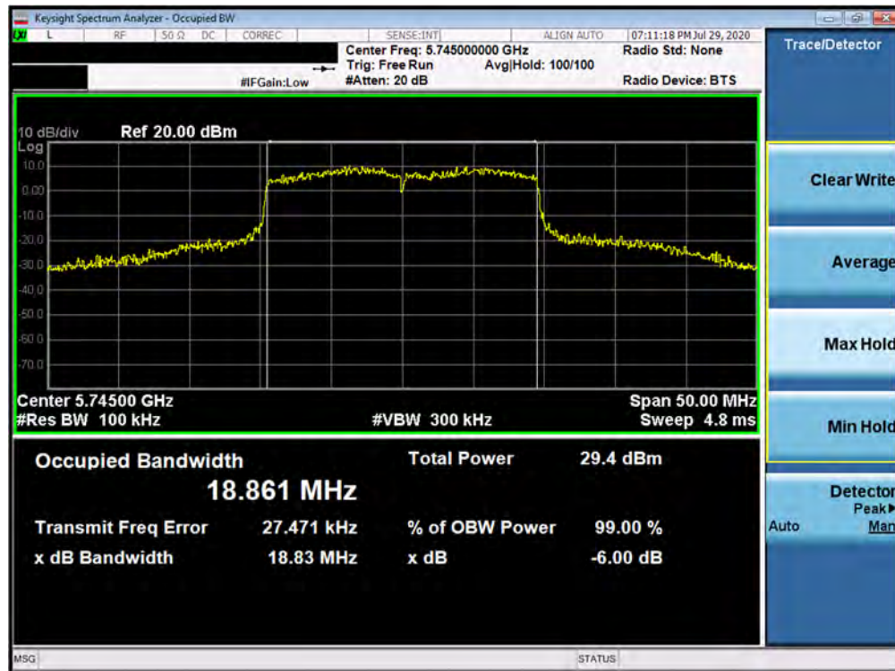
Plot 7-87. 6dB Bandwidth Plot ANT3 (20MHz BW 802.11ax – 242 Tones (UNII Band 3) – Ch. 149)
