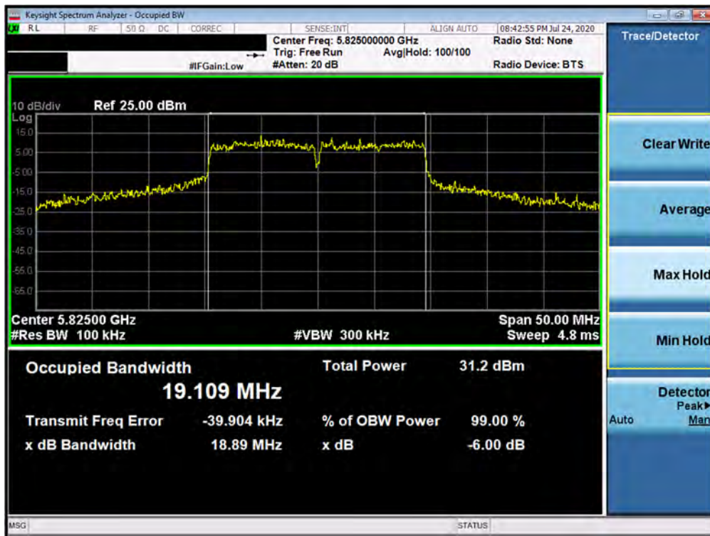
Plot 7-107. 6dB Bandwidth Plot ANT6 (20MHz BW 802.11ax – 242 Tones (UNII Band 3) – Ch. 165)
