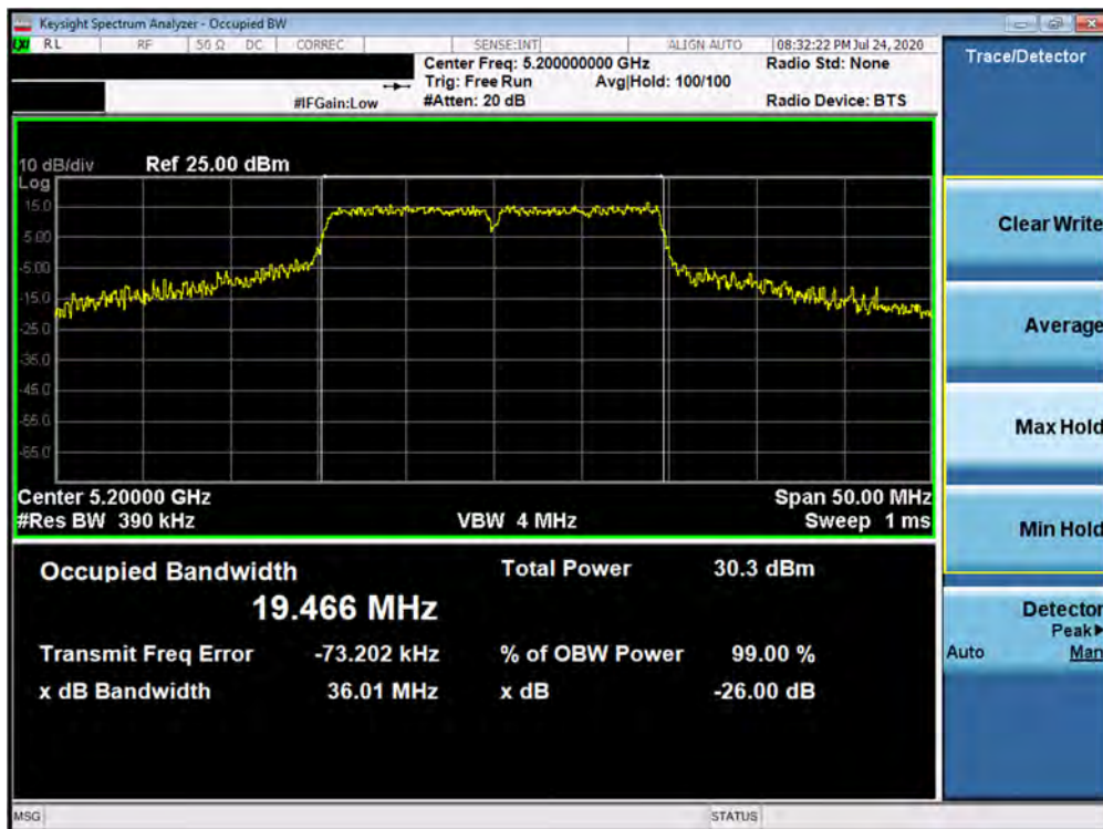
Plot 7-65. 26dB Bandwidth Plot ANT6 (20MHz BW 802.11ax – 242 Tones (UNII Band 1) – Ch. 40)
