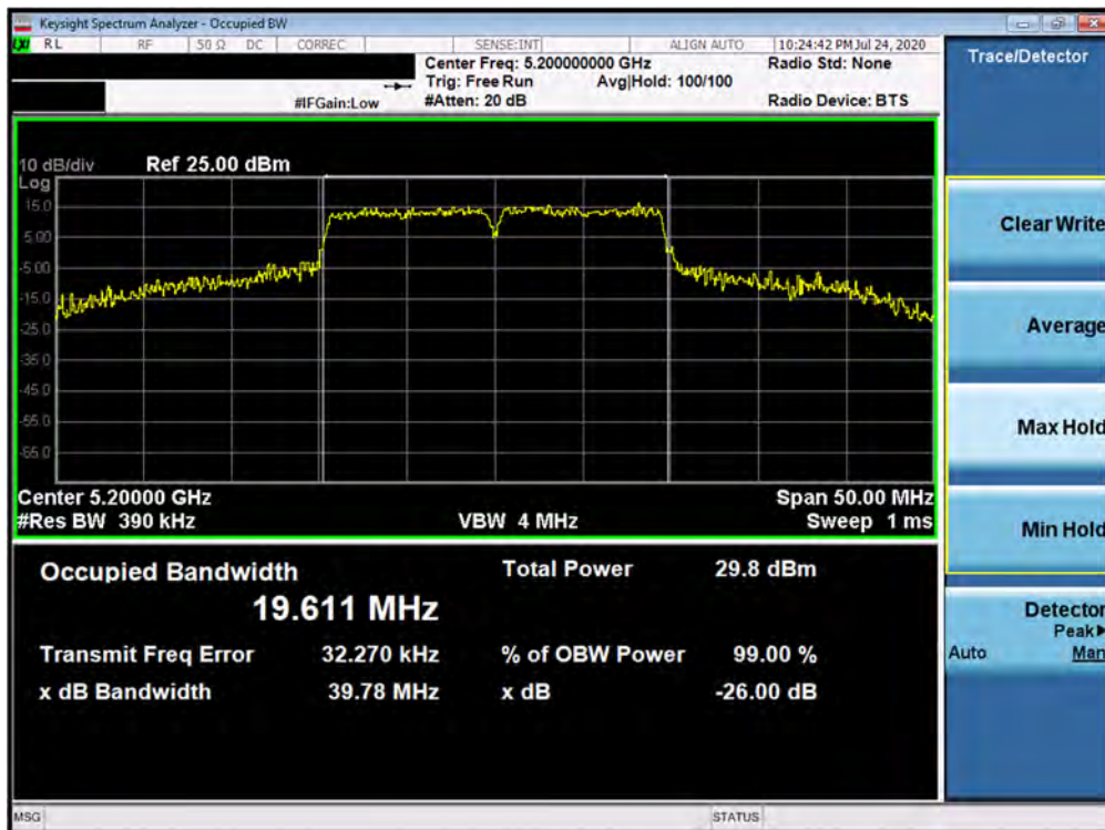
Plot 7-23. 26dB Bandwidth Plot ANT4 (20MHz BW 802.11ax – 242 Tones (UNII Band 1) – Ch. 40)
