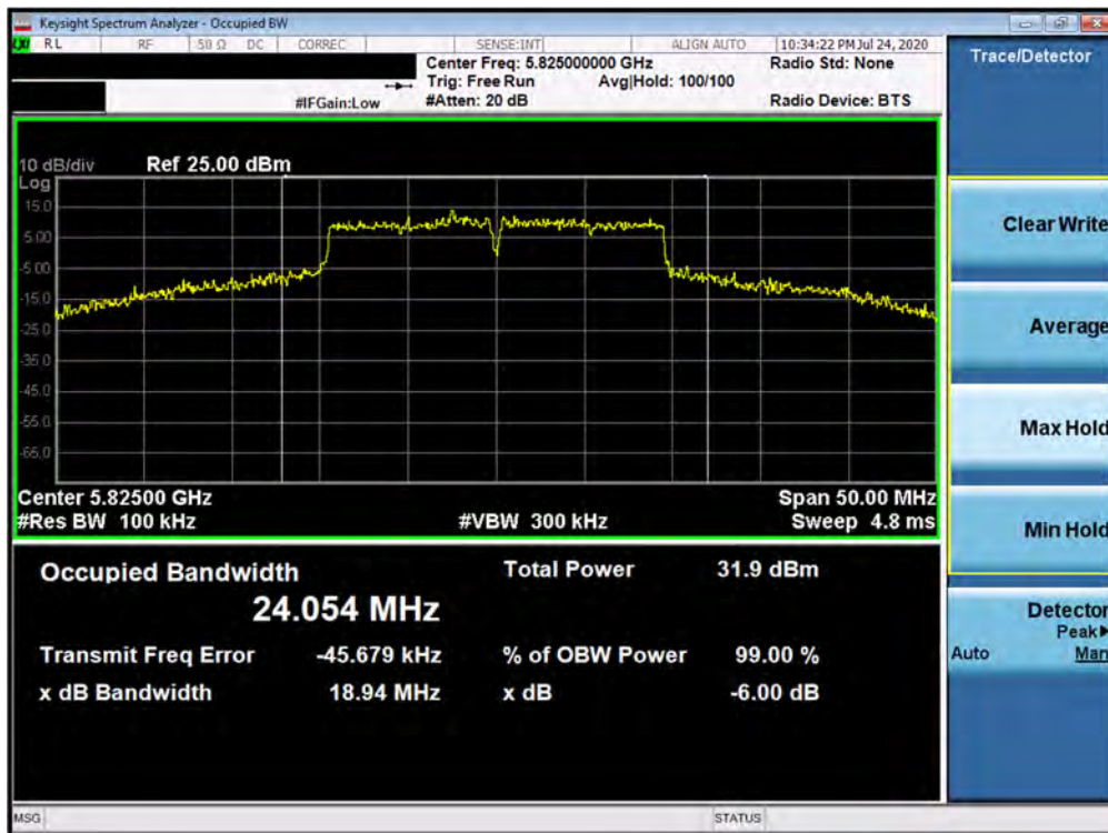
Plot 7-95. 6dB Bandwidth Plot ANT4 (20MHz BW 802.11ax – 242 Tones (UNII Band 3) – Ch. 165)
