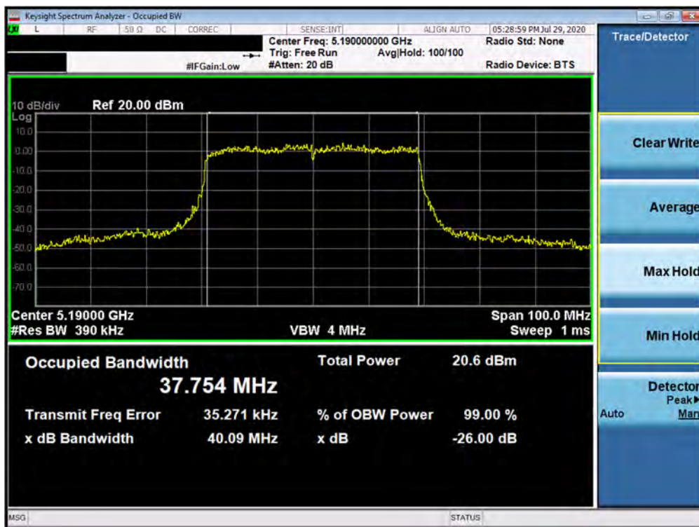
Plot 7-4. 26dB Bandwidth Plot ANT3 (40MHz BW 802.11ax – 484 Tones (UNII Band 1) – Ch. 38)
