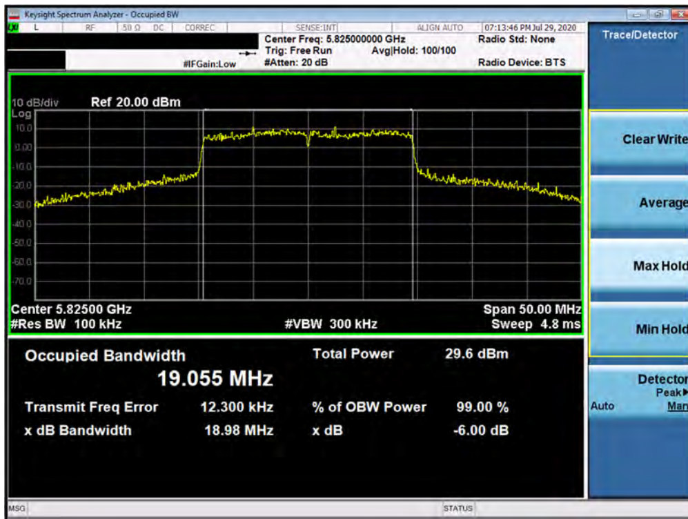
Plot 7-89. 6dB Bandwidth Plot ANT3 (20MHz BW 802.11ax – 242 Tones (UNII Band 3) – Ch. 165)
