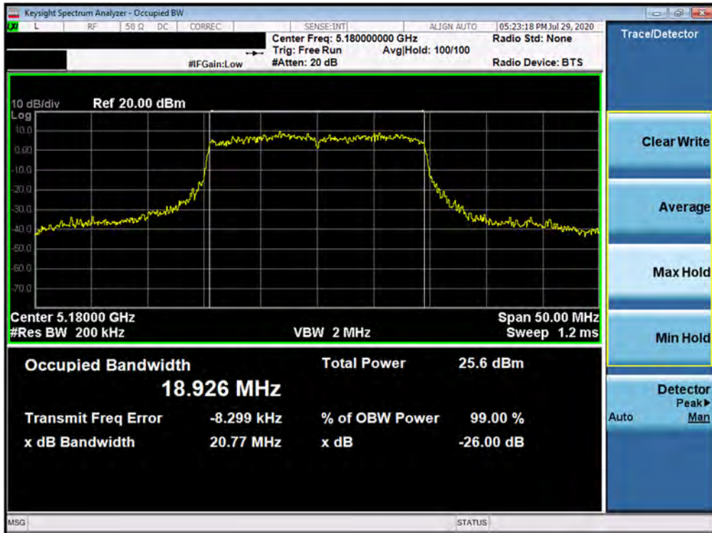
Plot 7-1. 26dB Bandwidth Plot ANT3 (20MHz BW 802.11ax – 242 Tones (UNII Band 1) – Ch. 36)
