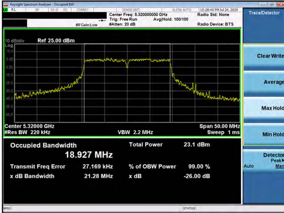
Plot 7-30. 26dB Bandwidth Plot ANT4 (20MHz BW 802.11ax – 242 Tones (UNII Band 2A) – Ch. 64)
