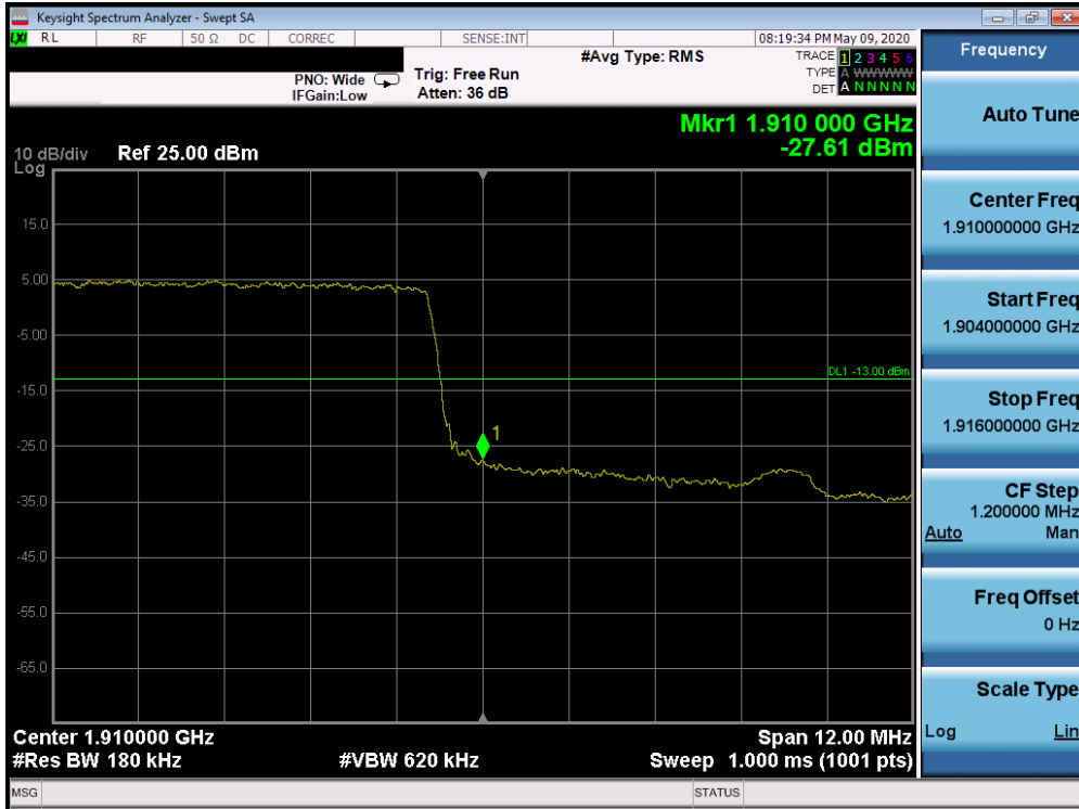
Plot 7-242. Upper Band Edge Plot (Band 2 - 15.0MHz QPSK - Full RB Configuration)
