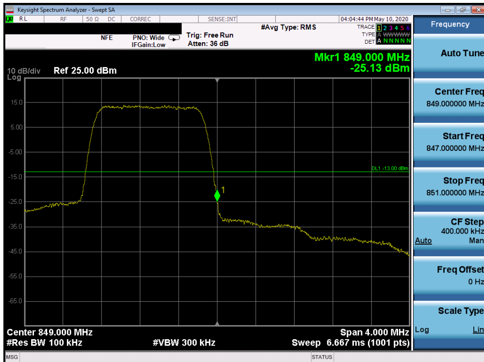
Plot 7-181. Upper Band Edge Plot (Band 5 - 1.4MHz QPSK - Full RB Configuration)
