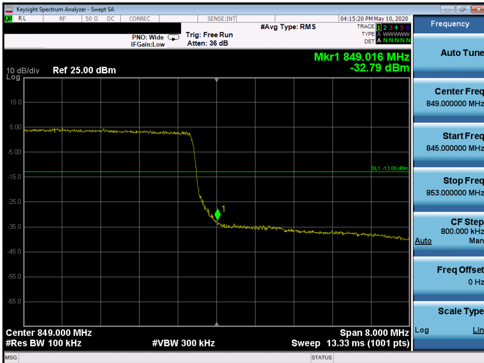
Plot 7-187. Upper Band Edge Plot (Band 5 - 10.0MHz QPSK - Full RB Configuration)
