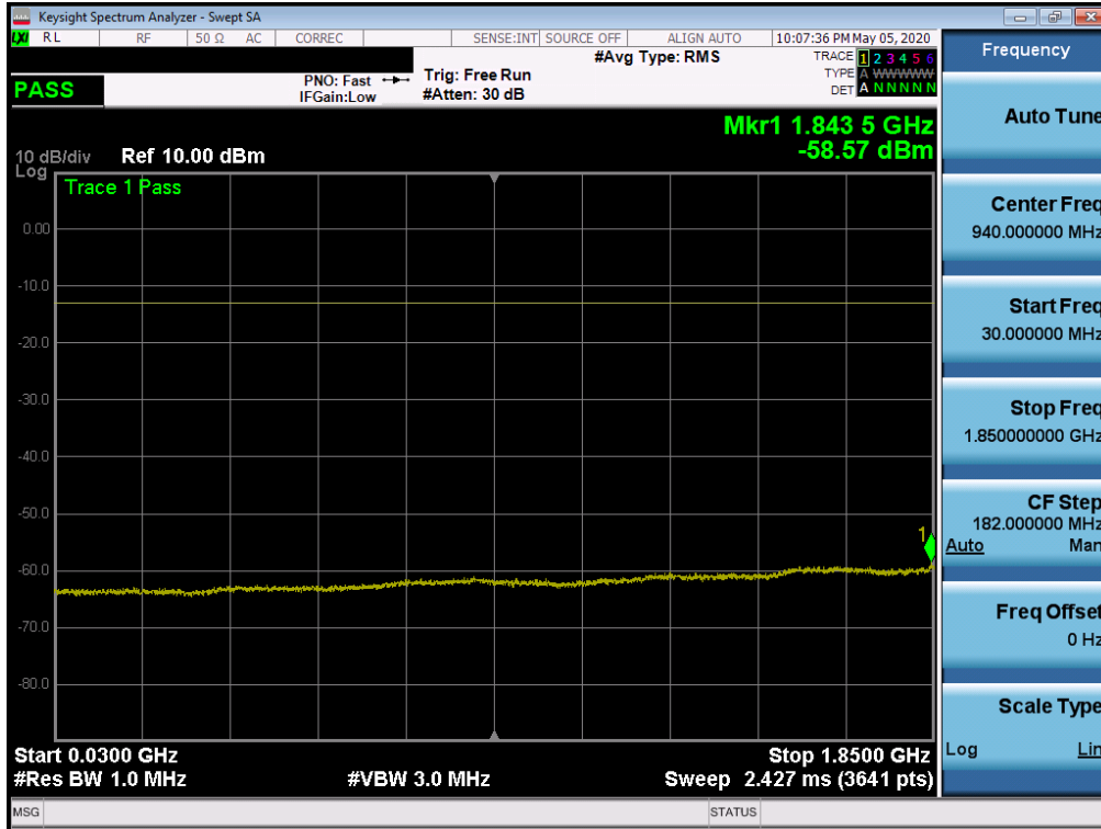
Plot 7-169. Conducted Spurious Plot (NR Band n2 - 20.0MHz - RB Size 1, RB Offset 0 - High Channel)
