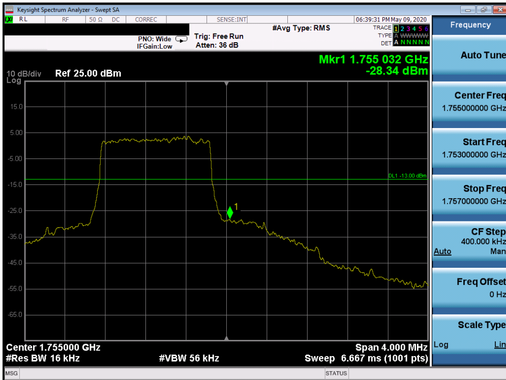
Plot 7-190. Upper Band Edge Plot (Band 4 - 1.4MHz QPSK - Full RB Configuration)
