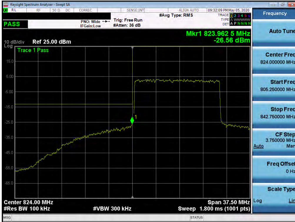
Plot 7-252. Lower Band Edge Plot (NR Band n5 – 15.0MHz - Full RB)
