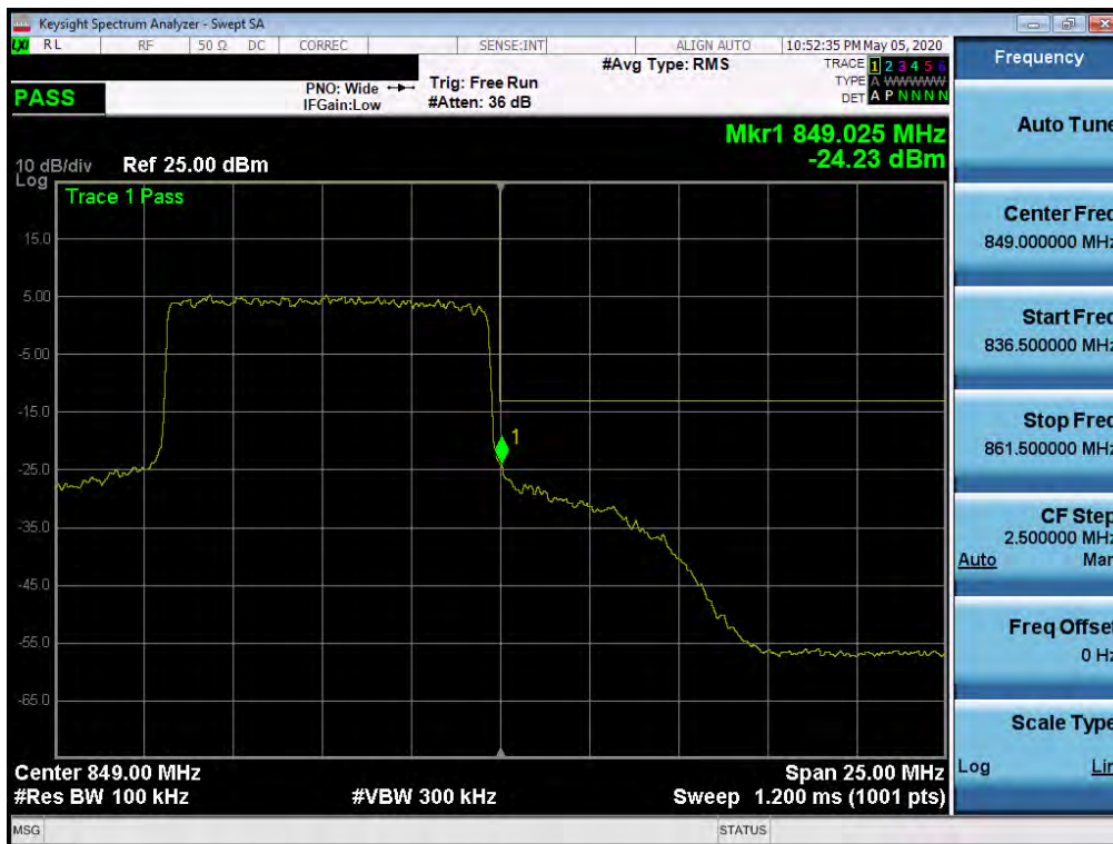
Plot 7-251. Upper Band Edge Plot (NR Band n5 – 10.0MHz - Full RB)
