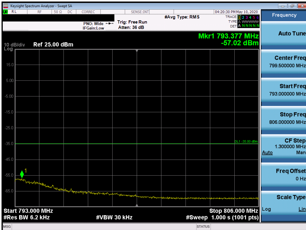
Plot 7-175. Upper Emission Mask Plot (Band 13 - 5.0MHz QPSK - Full RB Configuration)
