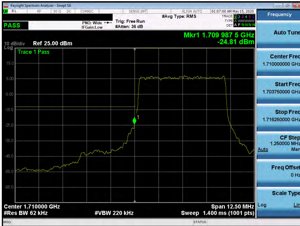
Plot 7-256. Lower Band Edge Plot (NR Band n66 – 5.0MHz - Full RB)
