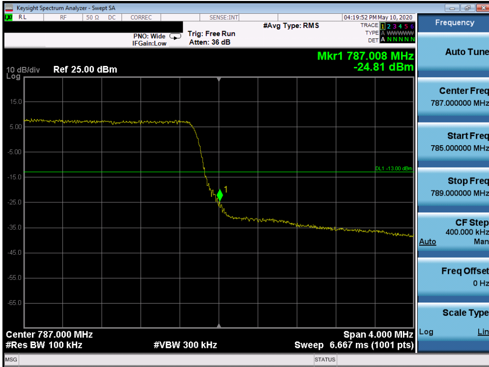
Plot 7-174. Upper Band Edge Plot (Band 13 - 5.0MHz QPSK - Full RB Configuration)
