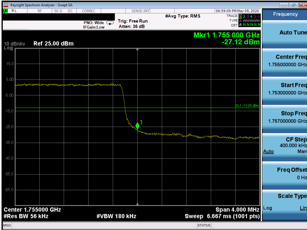
Plot 7-202. Upper Band Edge Plot (Band 4 - 5.0MHz QPSK - Full RB Configuration)
