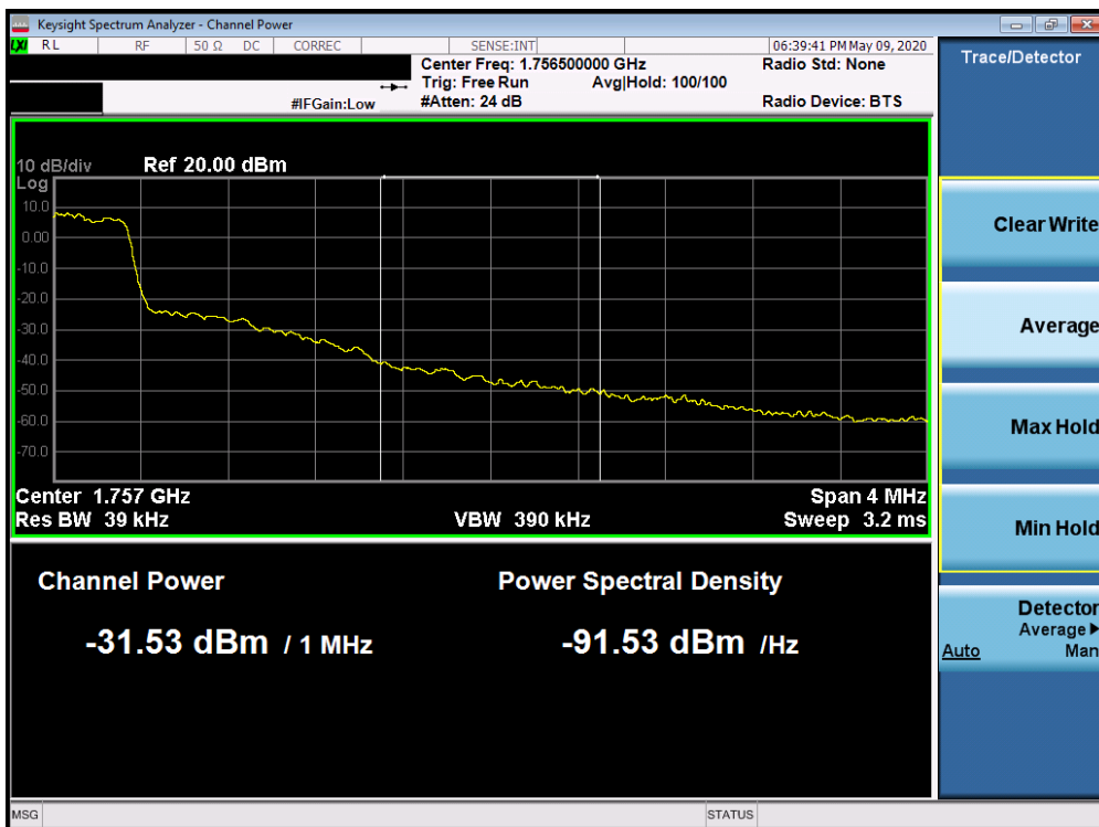
Plot 7-191. Upper Extended Band Edge Plot (Band 4 - 1.4MHz QPSK - Full RB Configuration)
