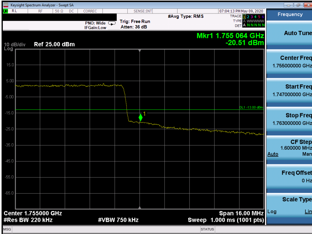
Plot 7-220. Upper Band Edge Plot (Band 4 - 20.0MHz QPSK - Full RB Configuration)
