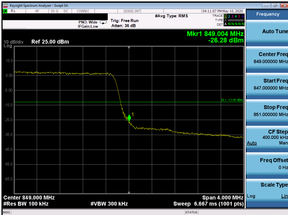
Plot 7-185. Upper Band Edge Plot (Band 5 - 5.0MHz QPSK - Full RB Configuration)
