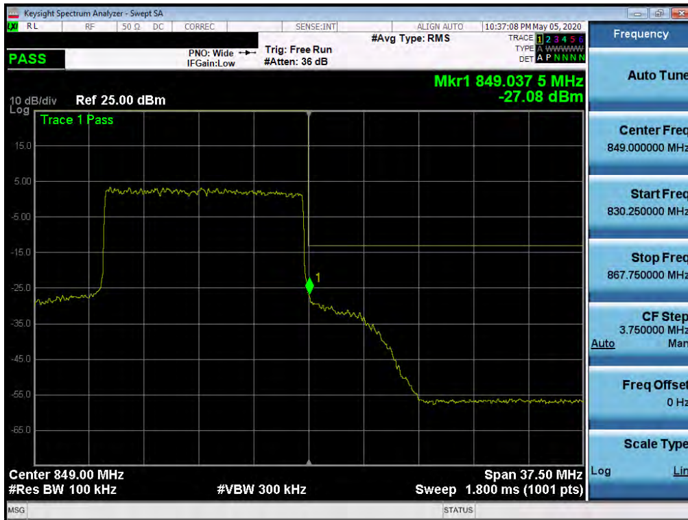
Plot 7-253. Upper Band Edge Plot (NR Band n5 – 15.0MHz - Full RB)
