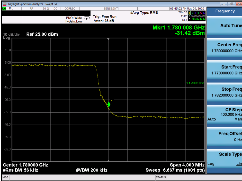
Plot 7-204. Upper Band Edge Plot (Band 66 - 5.0MHz QPSK - Full RB Configuration)
