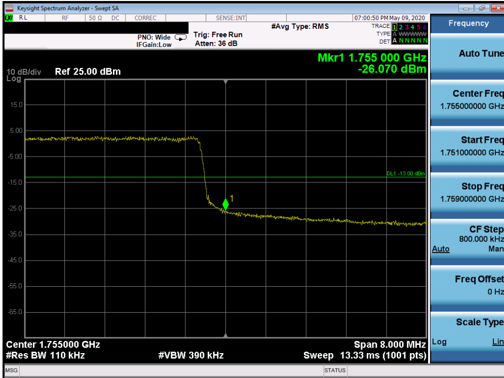
Plot 7-208. Upper Band Edge Plot (Band 4 - 10.0MHz QPSK - Full RB Configuration)
