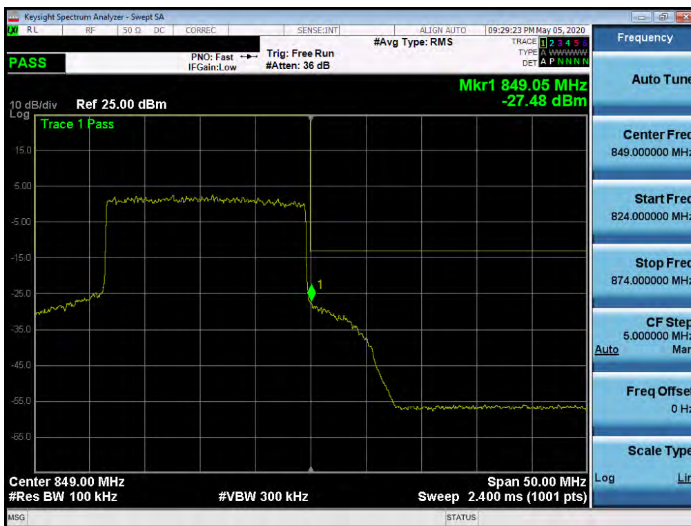
Plot 7-255. Upper Band Edge Plot (NR Band n5 – 20.0MHz - Full RB)
