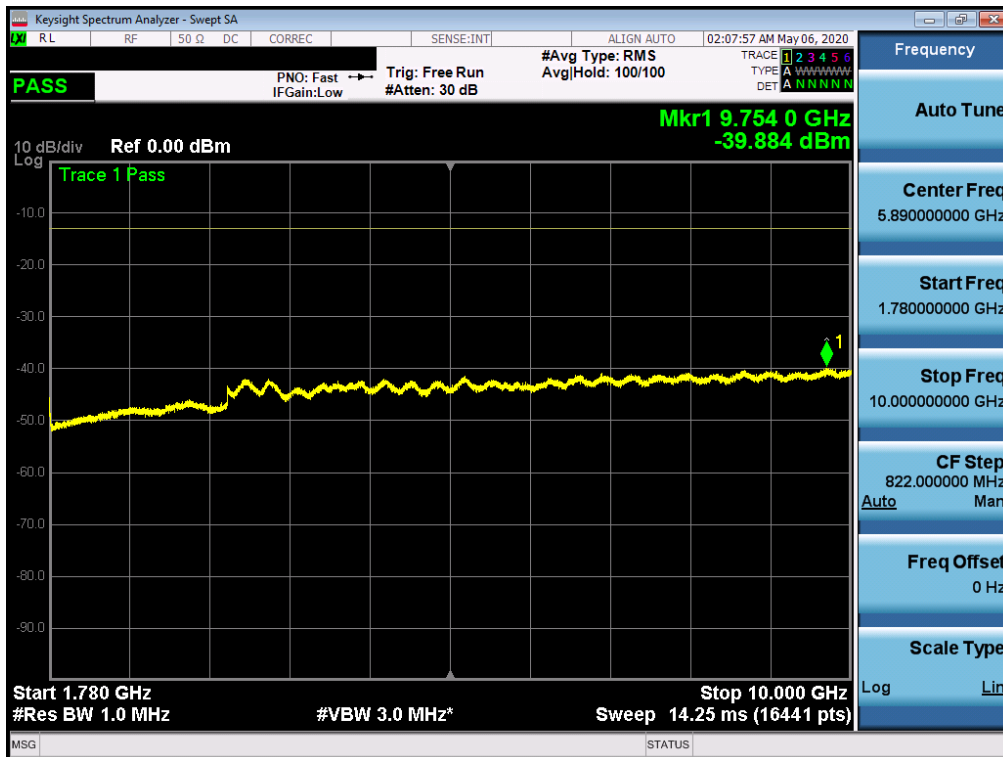
Plot 7-161. Conducted Spurious Plot (NR Band n66 - 20.0MHz - RB Size 1, RB Offset 0 - High Channel)
