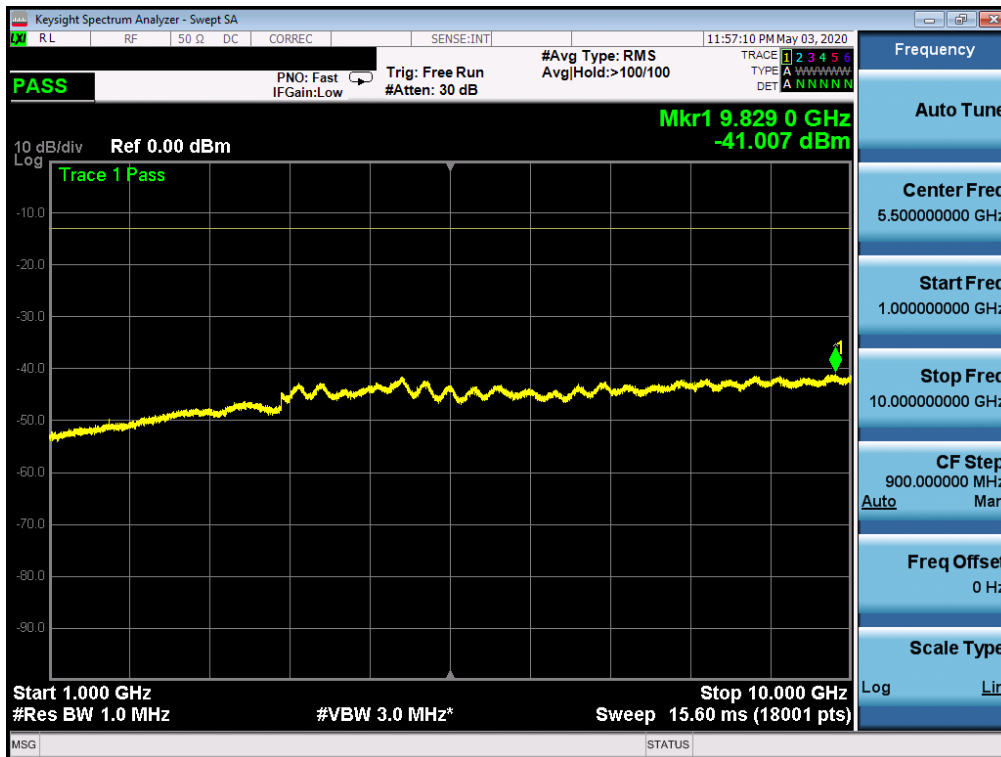
Plot 7-150. Conducted Spurious Plot (NR Band n5 - 20.0MHz - RB Size 1, RB Offset 0 - Mid Channel)
