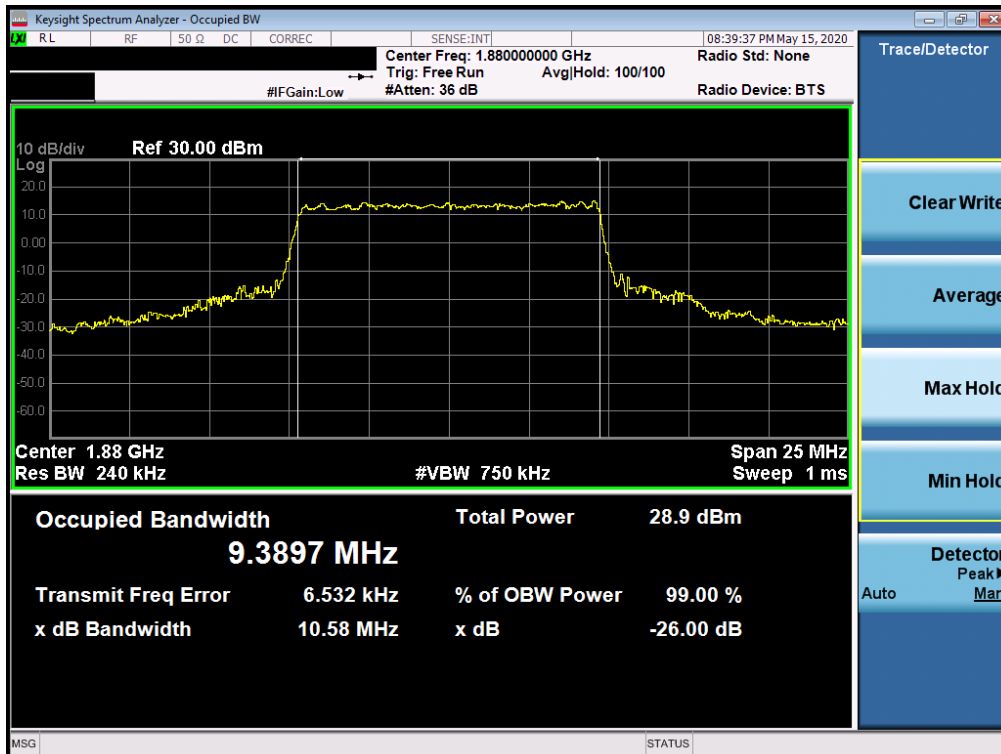
Plot 7-108. Occupied Bandwidth Plot (NR Band n2 - 10MHz CP-OFDM 64-QAM - Full RB Configuration)
