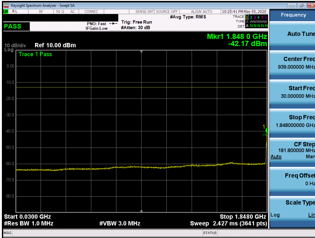
Plot 7-163. Conducted Spurious Plot (NR Band n2 -20.0MHz - RB Size 1, RB Offset 0 - Low Channel)
