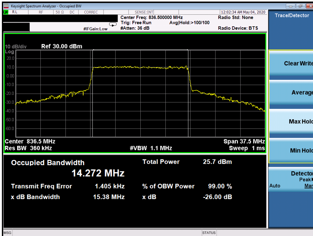
Plot 7-64. Occupied Bandwidth Plot (NR Band n5 - 15MHz CP-OFDM 256-QAM - Full RB Configuration)
