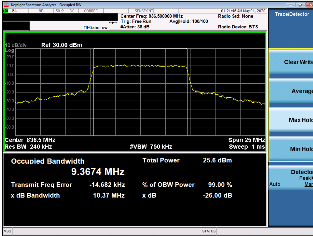
Plot 7-69. Occupied Bandwidth Plot (NR Band n5 - 10MHz CP-OFDM 256-QAM - Full RB Configuration)
