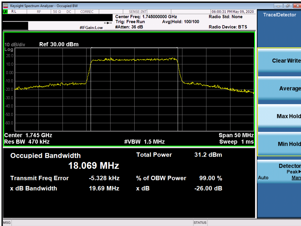
Plot 7-34. Occupied Bandwidth Plot (Band 66/4 - 20.0MHz QPSK - Full RB Configuration)
