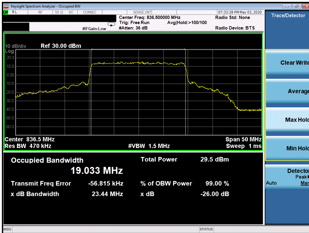
Plot 7-56. Occupied Bandwidth Plot (NR Band n5 - 20MHz CP-OFDM QPSK - Full RB Configuration)
