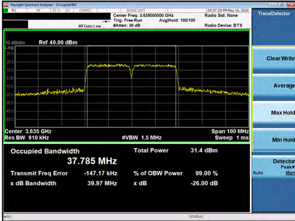
Plot 7-23. Occupied Bandwidth Plot (LTE Band 48 ULCA - 40.0MHz 16-QAM - Full RB Configuration)
