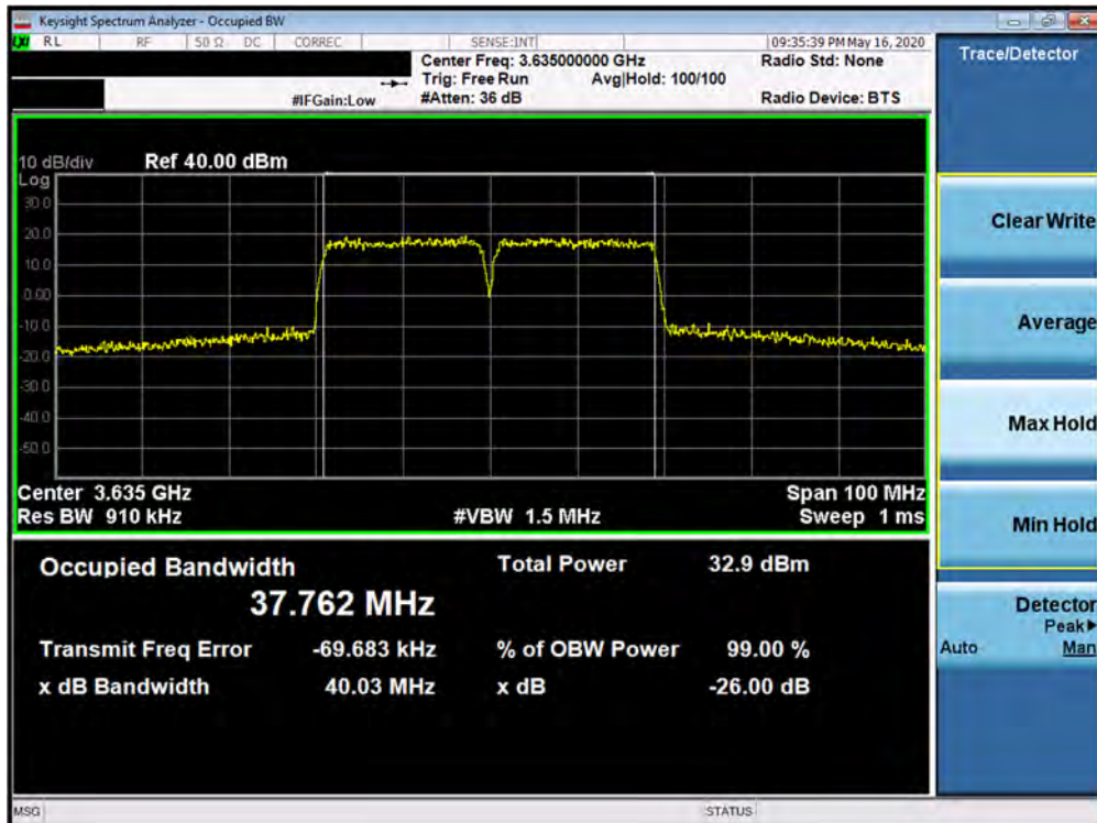
Plot 7-22. Occupied Bandwidth Plot (LTE Band 48 ULCA - 40.0MHz QPSK - Full RB Configuration)
